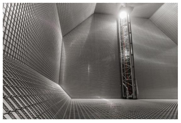
**Image caption:** *LNG fuelled tank design equipped with GTT's membrane containment system. Photo credit: GTT/ Roland Mouron*
