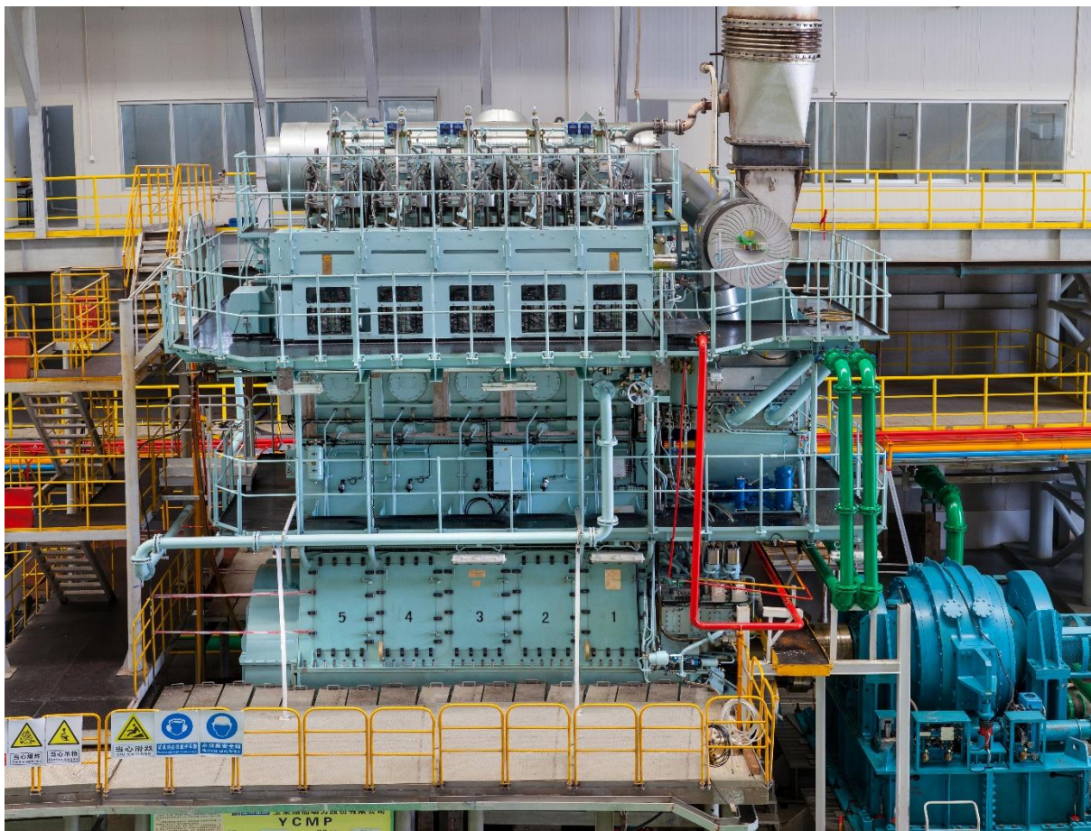
The 5RT-flex50DF is the first two-stroke low-pressure DF engine passing the FAT
