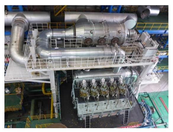
Caption: Pictures: High-pressure SCR system jointly developed by Winterthur Gas & Diesel Ltd and Hudong Heavy Machinery Co Ltd. The cylindrical SCR reactor unit is located in the exhaust duct from the engine cylinders to the turbocharger turbine inlet.
