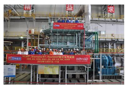
Caption: The Winterthur Gas & Diesel type Wärtsilä 5RT-flex50DF two-stroke engine with low-pressure dual-fuel technology during its Type Approval Test at the works of licensee YCMP at Zhuhai, China.
