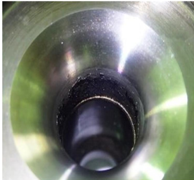
Contact mark on intermediate piece
