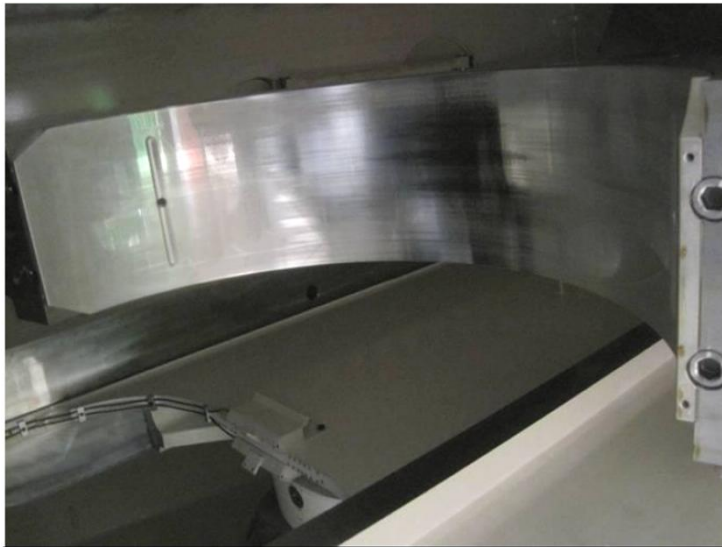
Contact surface of bottom end bearing
