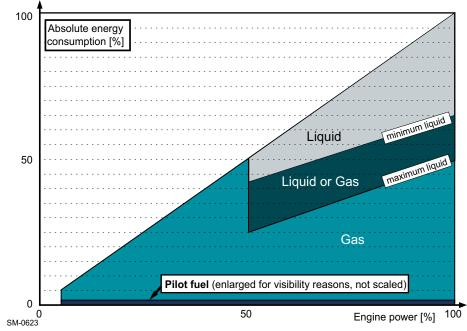
Figure 1-8 FSM — energy amount of different ratios of fuel
