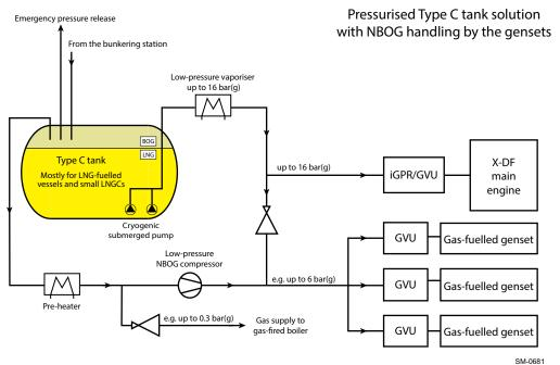
Figure 4-39 Pressurised Type C tank solution with NBOG handling by the gensets
