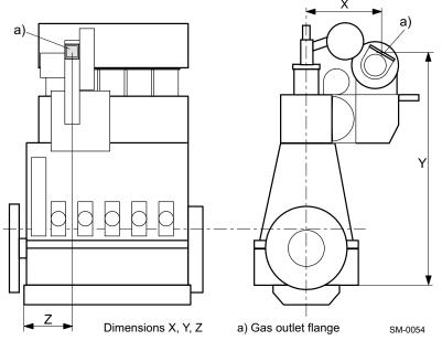
Figure 3-2 Thermal expansion, dim. X, Y, Z
