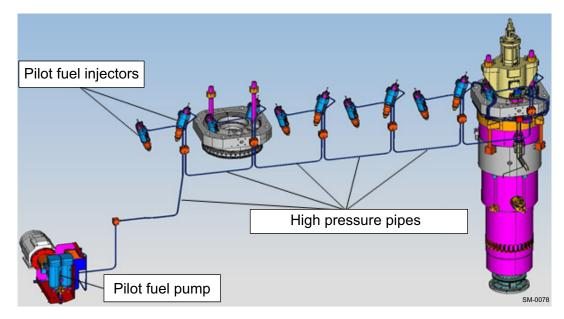
Figure 4-53 Pilot fuel high-pressure system
