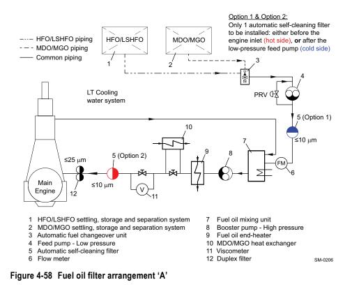
The automatic self-cleaning filter of maximum 10  $\mu$ m abs. is used to protect the engine against serious damage. It captures the catalytic fines which were not removed by the fuel oil separator. In addition, the filter provides a good indication of the separator efficiency.
