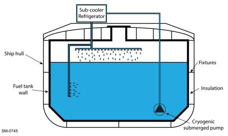
Figure 4-42 An LNG sub-cooler within an integrated tank
