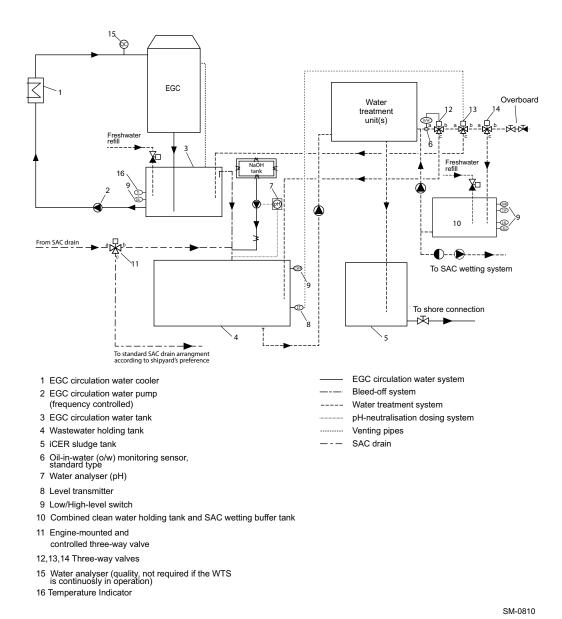
Figure 4-7 A new variant of the unified iCER drainage system
