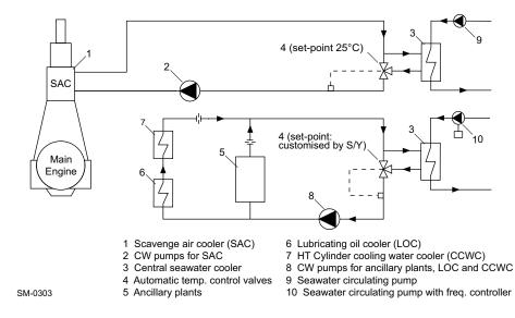
Figure 4-21 Separate SAC and LT cooling circuits
