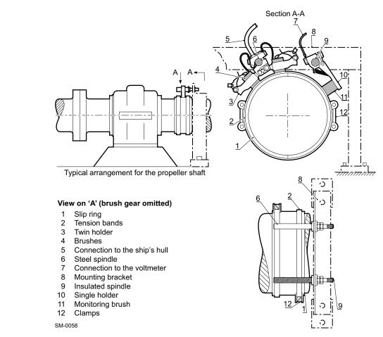
Figure 3-10 Typical shaft earthing arrangement
