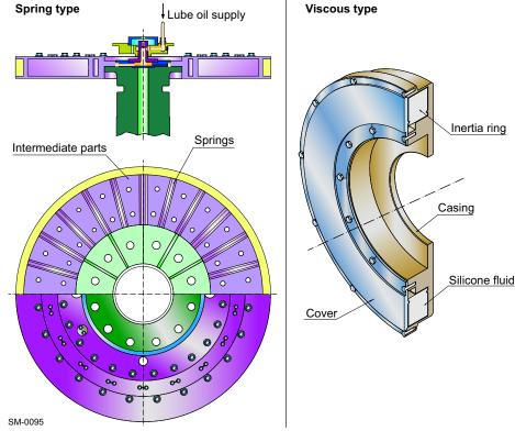
Figure 6-13 Vibration dampers (spring type and viscous type)
