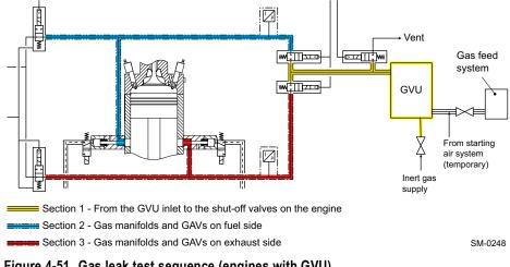
Figure 4-51 Gas leak test sequence (engines with GVU)
