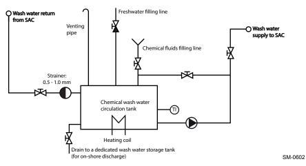
Figure 4-67 Offline SAC washing system (external system)
