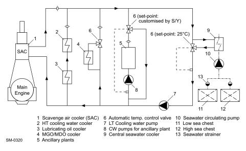
Figure 4-20 LT cooling water circuit — Dual set-point temperatures
