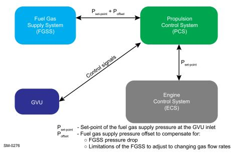
Figure 4-45 Fuel gas supply pressure control at the GVU inlet (engines with GVU)
