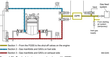
Figure 4-50 Gas leak test sequence (engines with iGPR)
