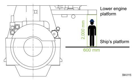
Figure 3-3 Minimum requirements for headroom
