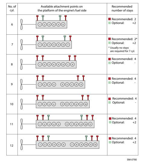
Figure 6-11 Engine stays arrangement on the engine fuel side
