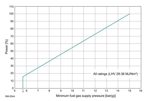
Figure 4-43 Design fuel gas supply pressure requirements
