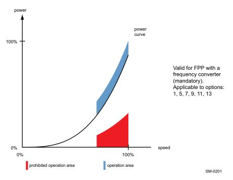
Figure 4-73 FPP with mandatory frequency converter
