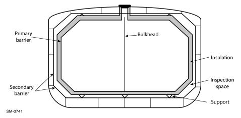
Figure 4-35 Section view of a free-standing Type A tank
