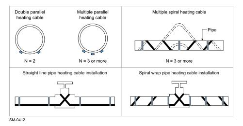
Figure 4-27 Trace heating cable arrangement
