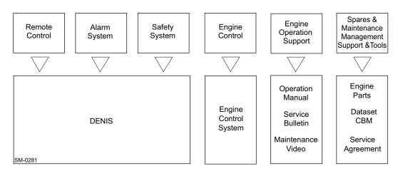
Figure 5-2 Engine management and automation concept
