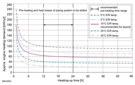
Figure 4-23 Pre-heating power requirement per cylinder
