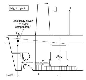
Figure 6-2 Locating an electrically-driven compensator
