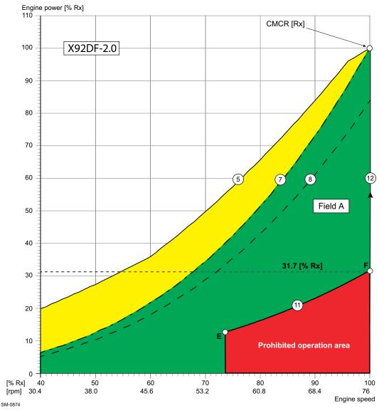
Figure 2-9 The prohibited operation area (CMCR speed = 95% of R1—R2)
