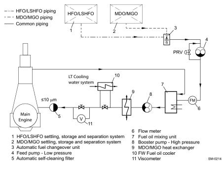
Figure 4-59 Fuel oil filter arrangement 'B'
