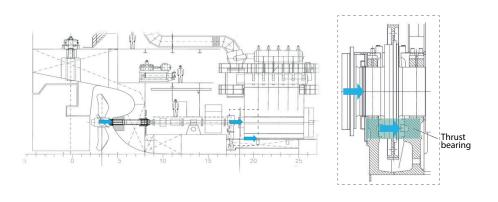
Figure 3-4 Force transmission to the engine foundation
