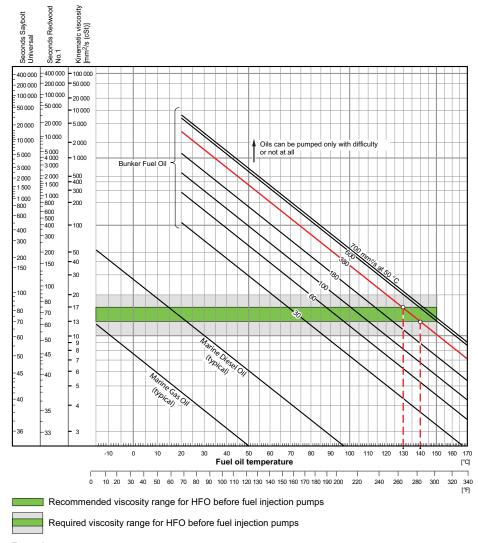
Example To obtain the recommended viscosity before fuel injection pumps a fuel oil of 380 mm<sup>2</sup>/s (cSt) at 50 °C must be heated up to 130 °C to 140 °C.
