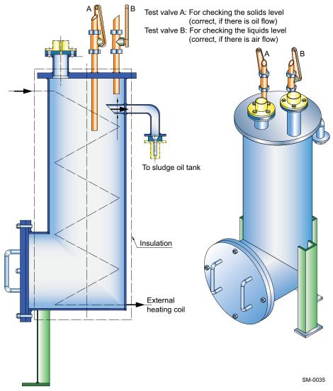
Figure 4-63 Design proposal of the WinGD sludge oil trap
