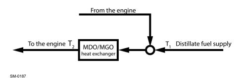
Figure 4-56 MDO/MGO heat exchanger
