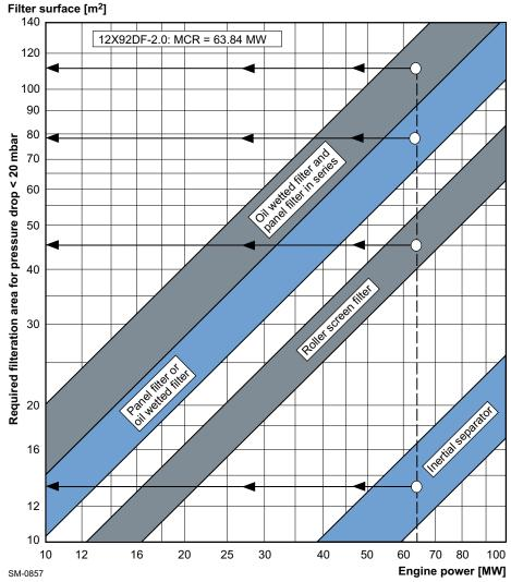
Figure 4-71 Air filter size (example for the 12-cylinder engine)
