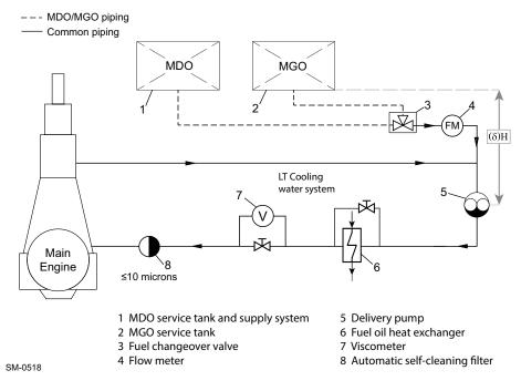
Figure 4-60 Fuel oil system — Arrangement with only MDO/MGO or MGO
