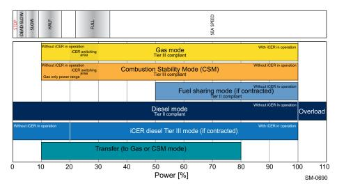
Figure 1-2 Operating modes of the X-DF2.0 engine
