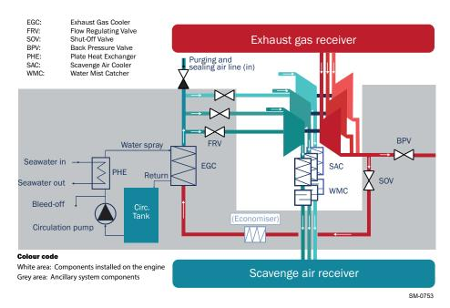
Figure 4-3 The iCER system with three turbochargers and the exhaust gas return pipe routed to the turbocharger connection from below
