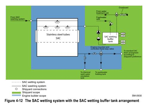
**Functional description** The SAC wetting system is controlled by an SAC wetting control unit. The Engine Control System (ECS) communicates with this control unit, commanding when wetting starts and stops.
