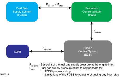
Figure 4-44 Fuel gas supply pressure control at the engine inlet (engines with iGPR)
