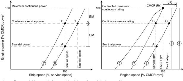
A Power and ship speed during sea-trials - light running and ideal sea condition
