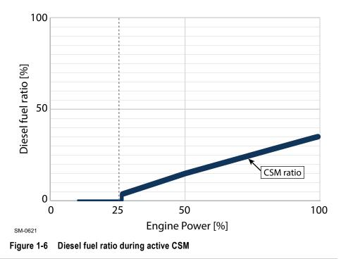
The CSM, like the FSM<sup>1)</sup>, injects liquid fuel by the main injectors, in addition to the gas fuel. However, unlike FSM<sup>1)</sup>, the diesel fuel ratio is set by the CSM, as shown in Figure 1-6,  $\blacksquare$  1-12.
