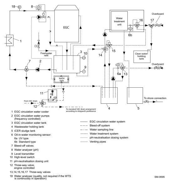
Figure 4-6 The iCER drainage system valid for all iCER operating mode options
