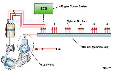
Figure 1-5 The Flex system parts
