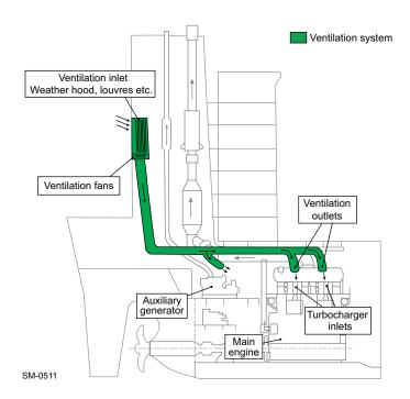
Figure 4-69 Ventilation system arrangement 1: Engine room ventilation system
