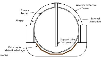
Figure 4-36 Section view of a free-standing Type B tank of moss design
