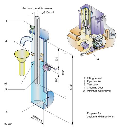
Figure 4-66 Arrangement of automatic water drain
