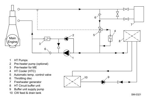
Figure 4-22 HT cooling water circuit
