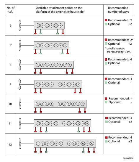
Figure 6-10 Engine stays arrangement on the exhaust side
