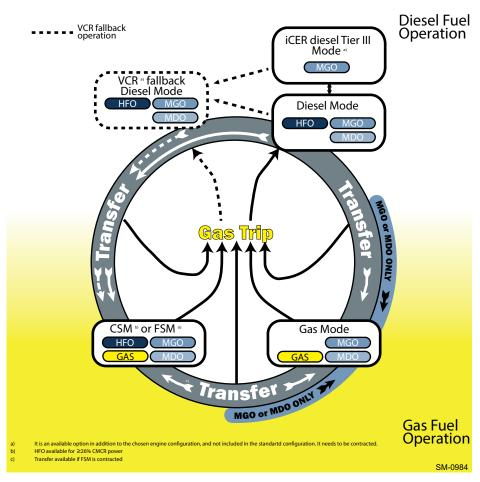
Figure 1-9 The fuel transfers and gas trips
