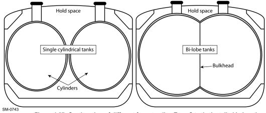
Figure 4-37 Section view of different free-standing Type C tanks installed below the deck
