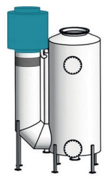
Figure 4-17 Arrangement of the additional economiser (Source: Alfa Laval)
