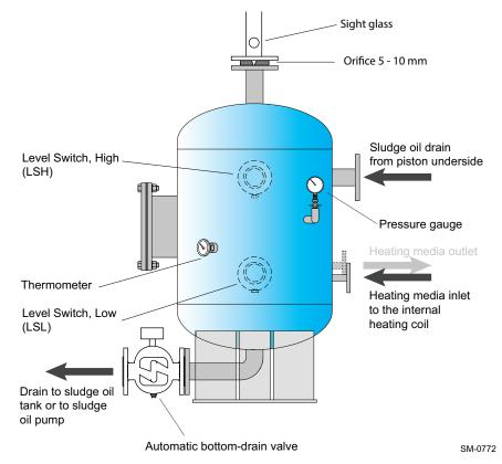
Figure 4-65 Design proposal of an automatically bottom-drained sludge oil trap
