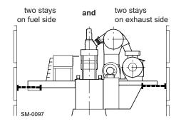
Figure 6-7 General arrangement of hydraulic type stays for both-side installation
