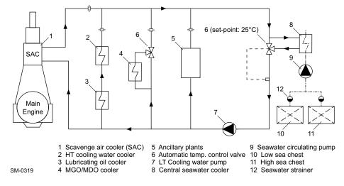
Figure 4-19 LT cooling water circuit — Single set-point temperature
