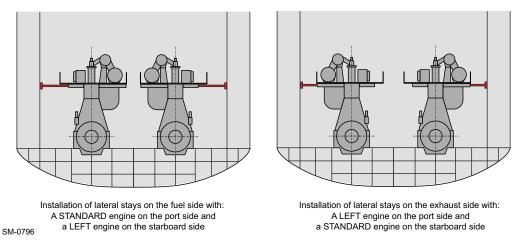
Figure 6-9 Variants of twin-engine installations with a standard and a left engine
