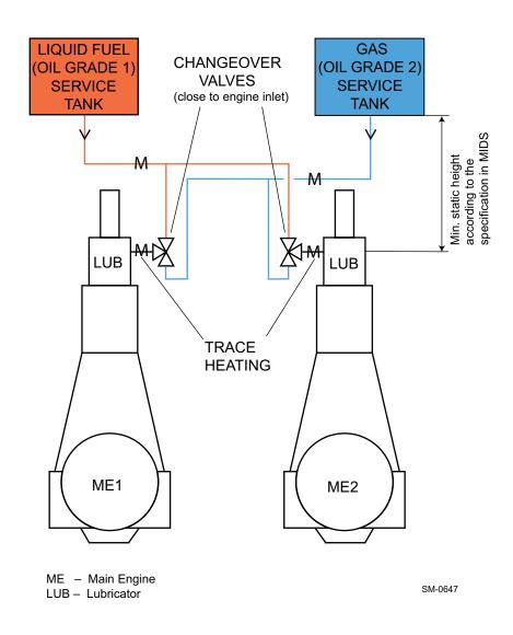
Figure 4-25 Dual cylinder LO installation, enabling independent gas and liquid fuel (maximum 0.50% m/m sulphur) operation with a manual changeover valve
