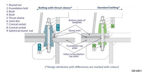
Figure 3-6 Foundation bolting
