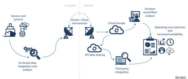
Figure 5-7 The WiDE data collection and analysis process
