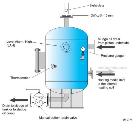
Figure 4-64 Design proposal of a manually bottom-drained sludge oil trap
