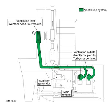
Figure 4-70 Ventilation system arrangement 2: Direct engine ventilation system
