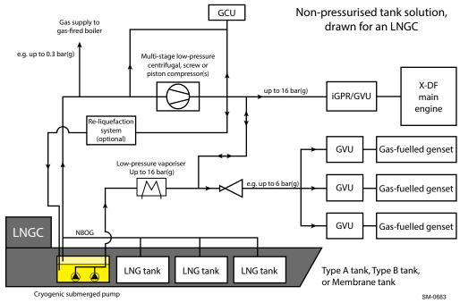
Figure 4-41 Non-pressurised tank solution, drawn for an LNGC
