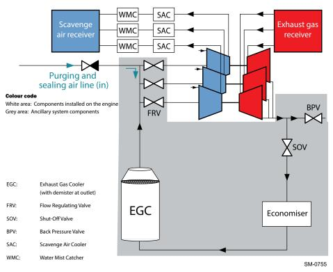
Figure 4-13 The iCER exhaust gas system with three turbochargers and the exhaust gas return pipe routed to the turbocharger connection from below
