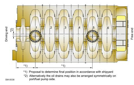
Figure 4-29 Arrangement of vertical LO drains for the 6-cylinder engines
