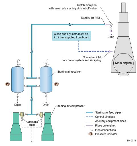
Figure 4-62 Air supply system
