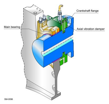
Figure 6-14 Example of axial vibration damper
