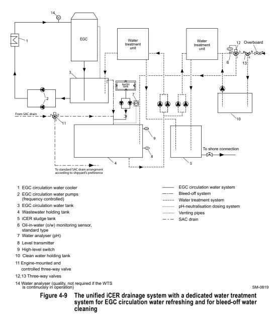
Figure 4-9, 1 4-16 provides a schematic of a solution which refreshes the EGC circulation water tank with water from the wastewater holding tank. This tank includes a mixture of the SAC drain water and bleed-off water, which ensures that the EGC circulation water tank is always filled with sufficient clean water.
