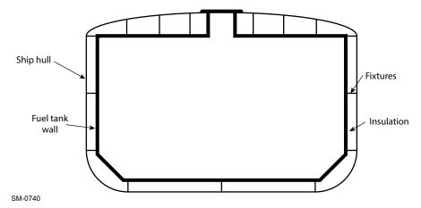
Figure 4-34 Section view of an integrated membrane tank
