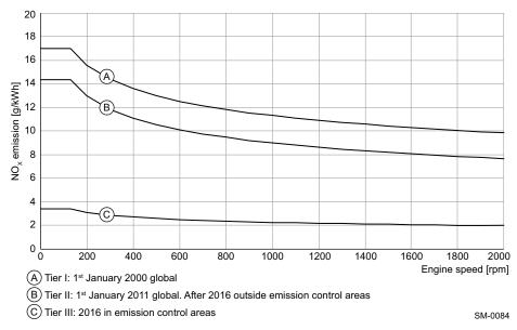
Figure 7-2 Speed dependent maximum allowable average of NO<sub>x</sub> emissions
