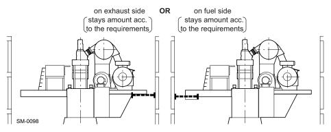
Figure 6-6 General arrangement of hydraulic type stays for one-side installation
