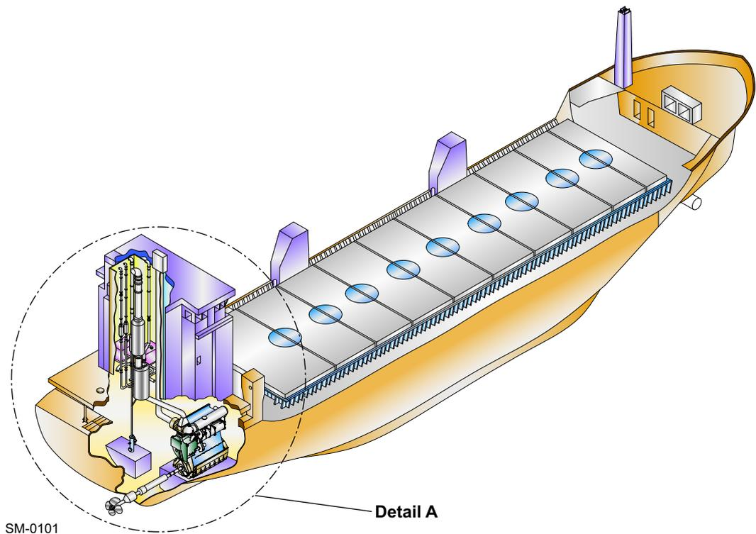
Figure 4-18 Direct suction of combustion air — main and auxiliary engine
