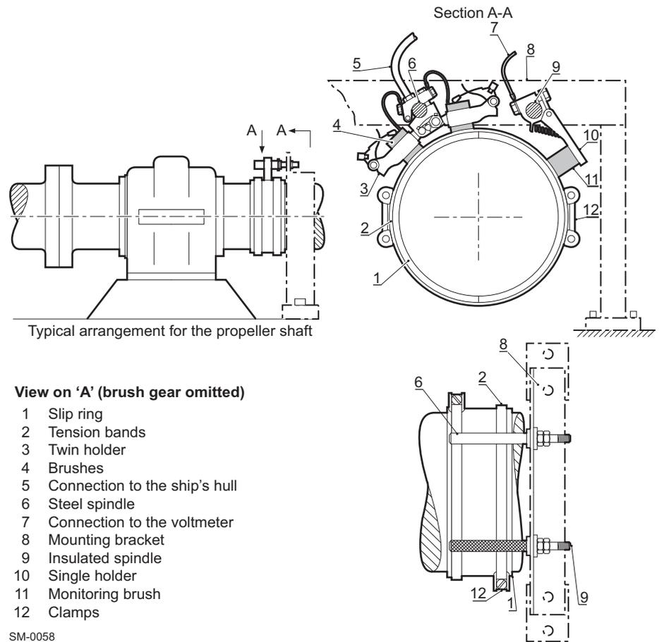
Figure 3-4 Shaft earthing arrangement
