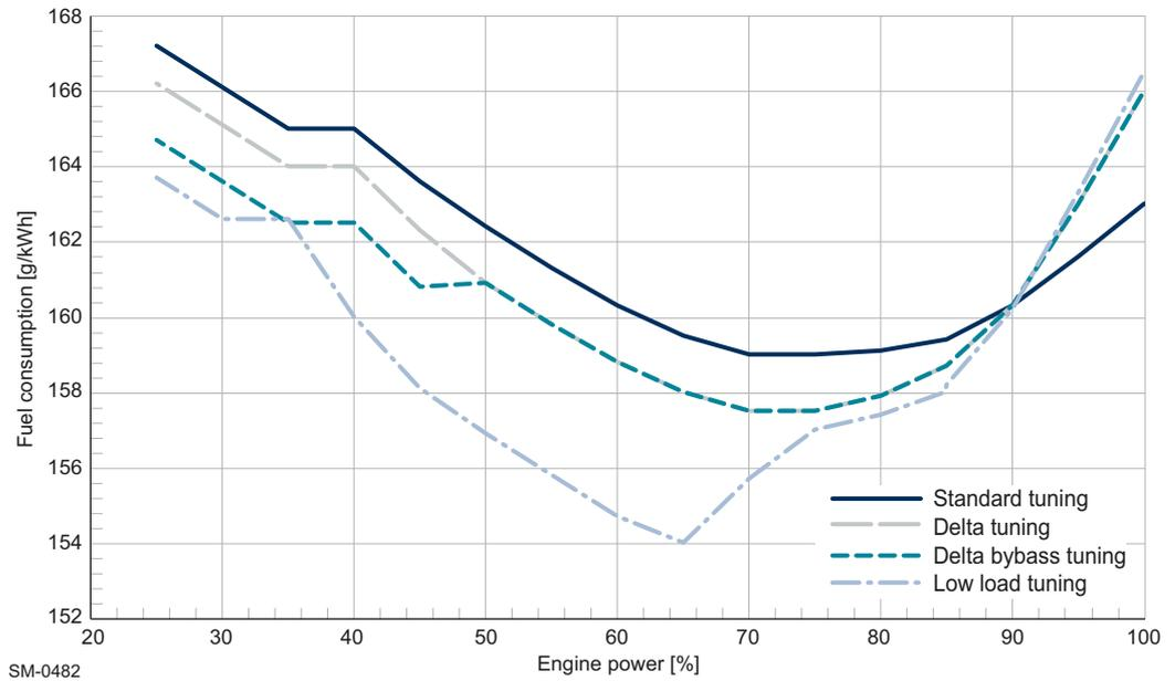
Figure 1-3 Typical BSFC curves in relation to engine power
