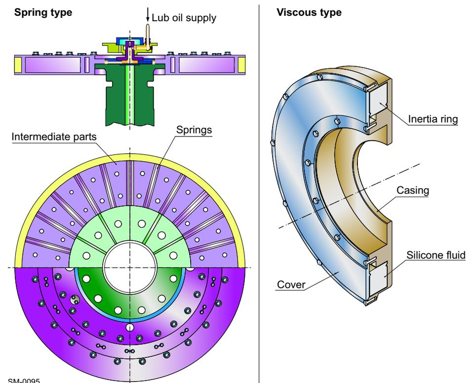
Figure 6-6 Vibration dampers (spring type and viscous type)
