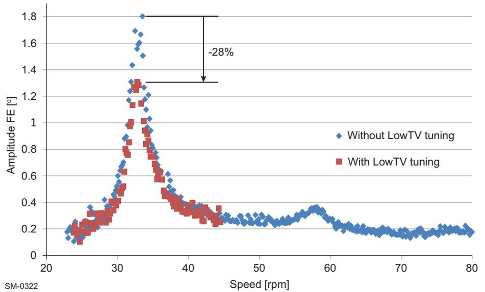
Figure 1-8 Vibration amplitudes - Achievements with default LowTV tuning
