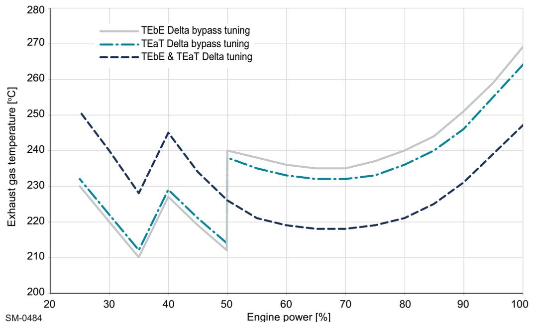
Figure 1-6 Exhaust gas temperature increase with DBT
