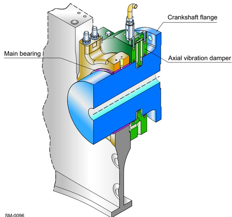
Figure 6-7 Example of axial vibration damper
