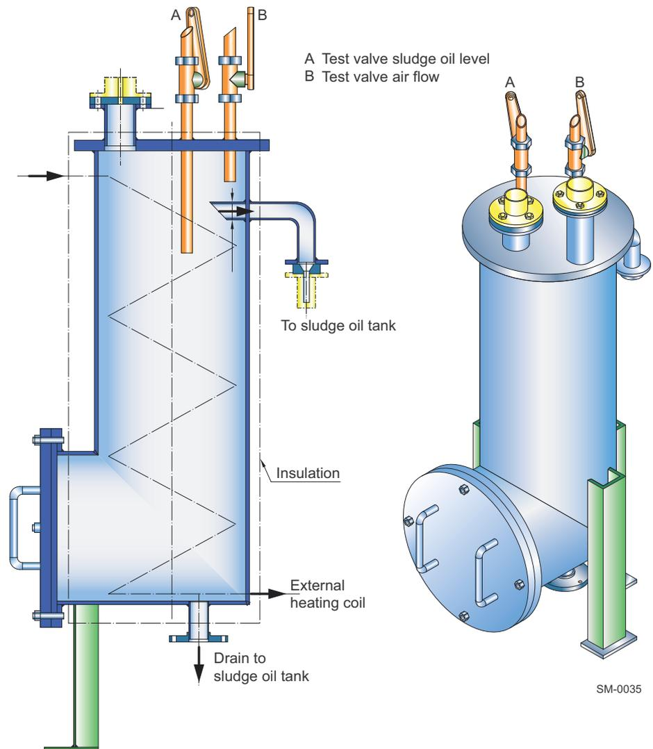
Figure 4-15 Sludge oil trap
