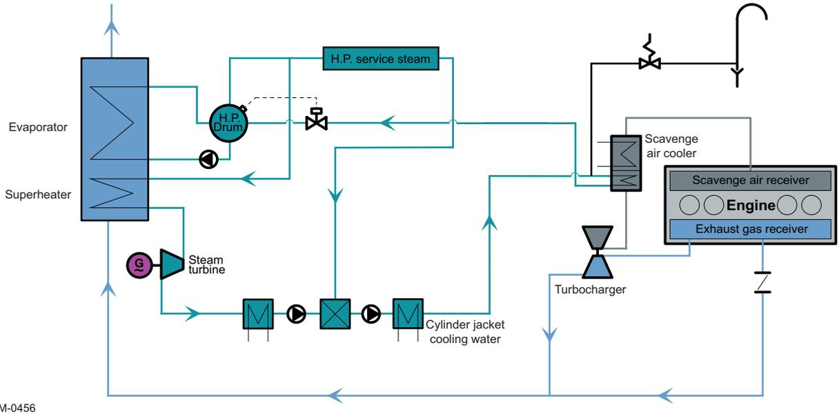
Figure 4-29 Single-pressure steam system with evaporator and superheater
