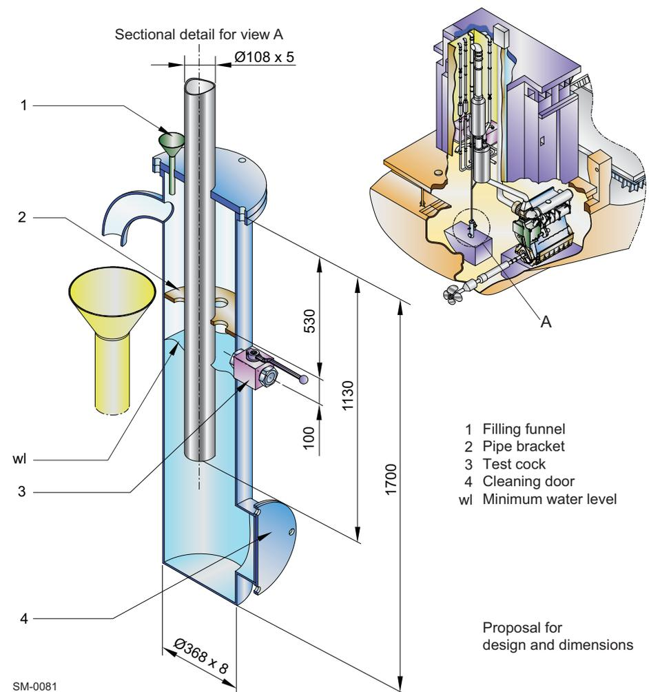
Figure 4-16 Arrangement of automatic water drain
