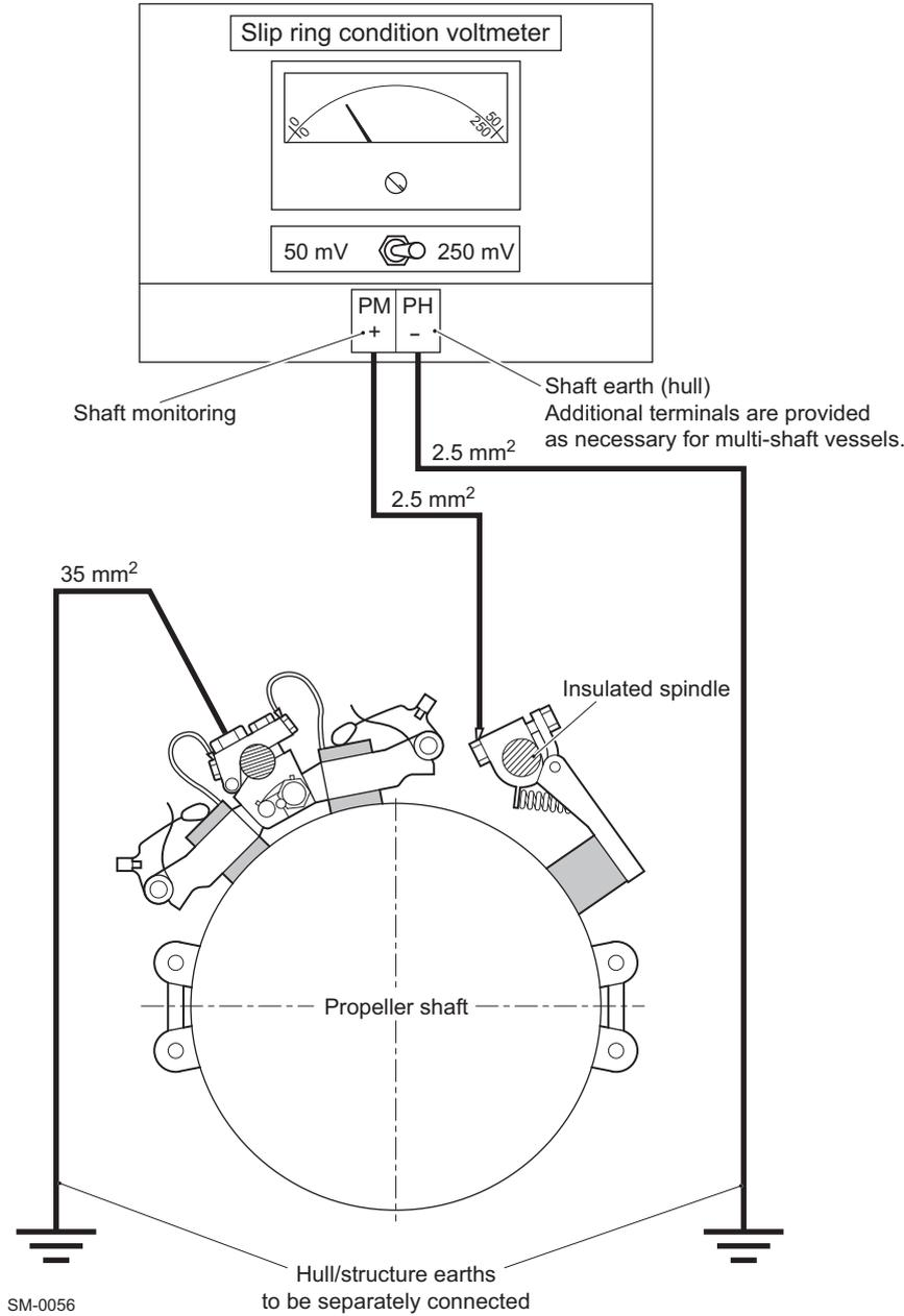
Figure 3-5 Shaft earthing with condition monitoring facility
