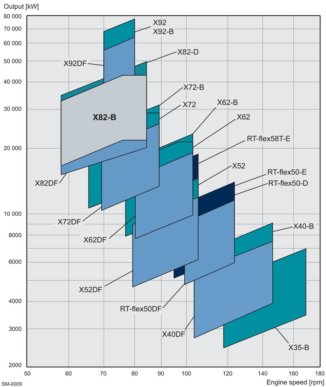
Figure 1-1 Power/speed range of WinGD engines complying with IMO regulations
