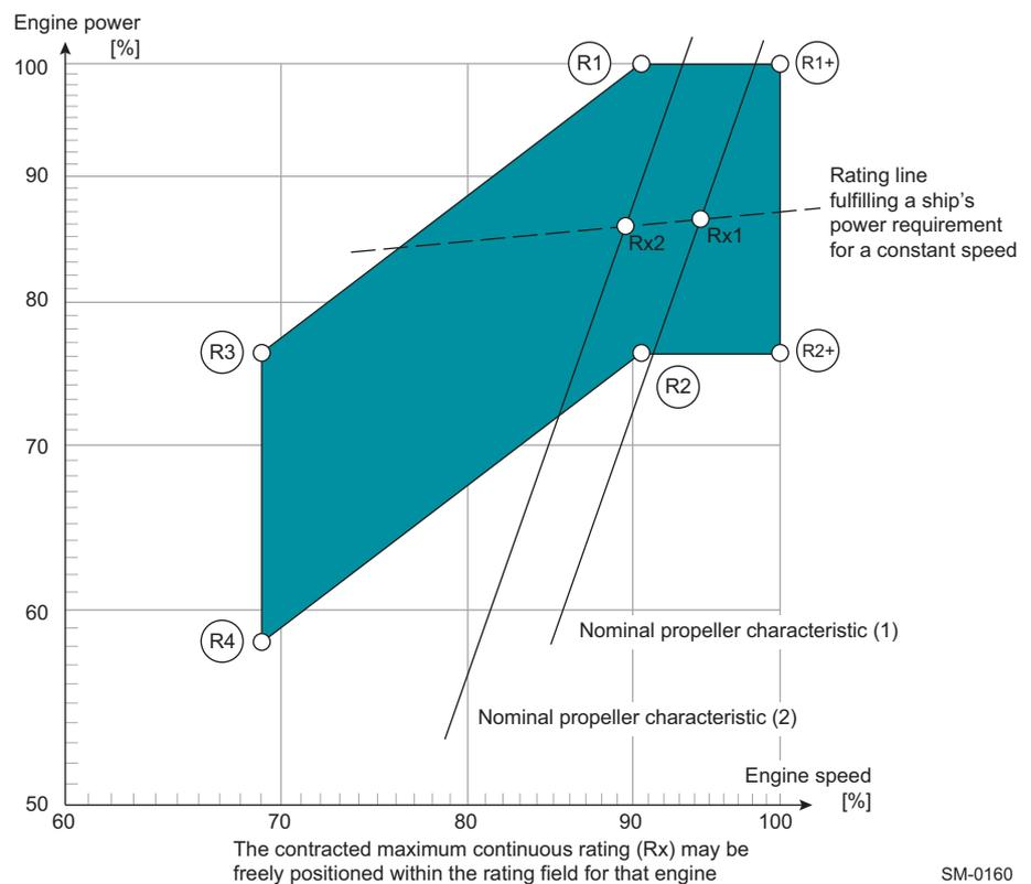
Figure 2-1 Engine rating field for X82-B
