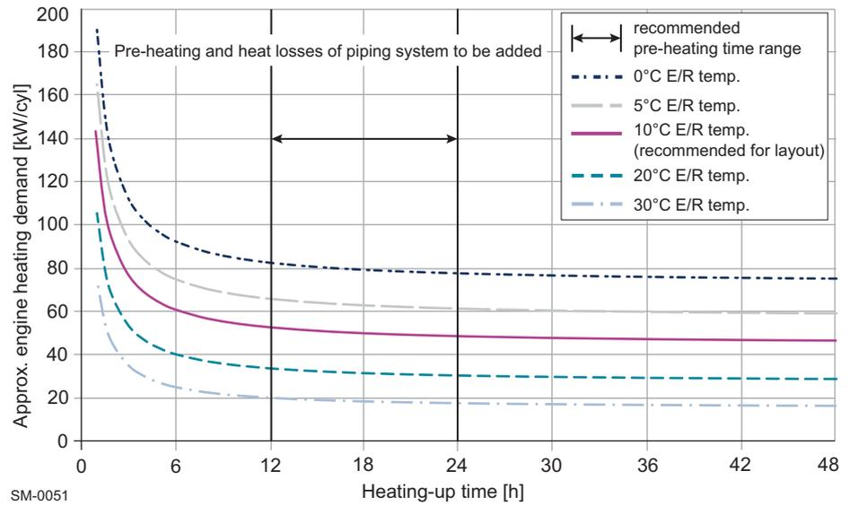
Figure 4-5 Pre-heating power requirement per cylinder
