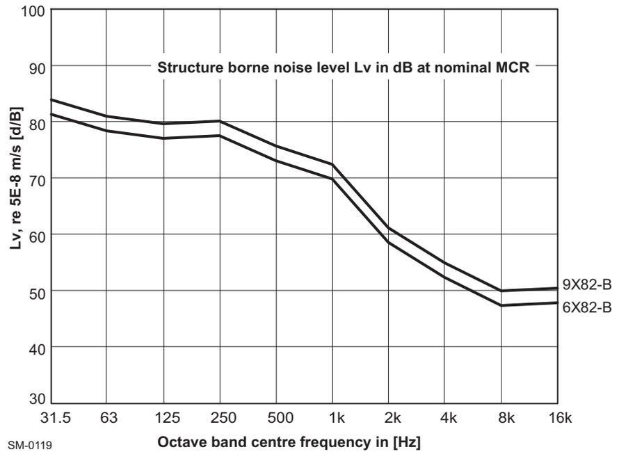
Figure 7-7 Structure-borne noise level at engine feet vertical
