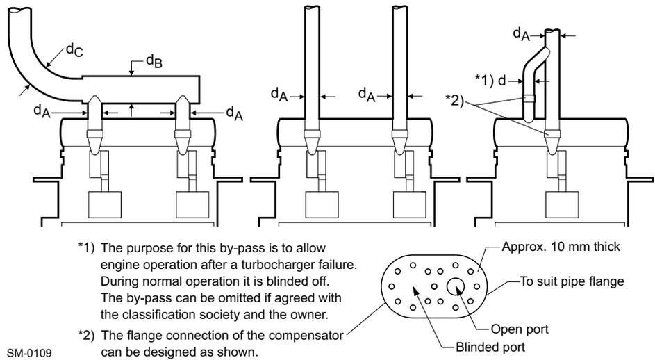
Figure 4-17 Determination of exhaust pipe diameter
