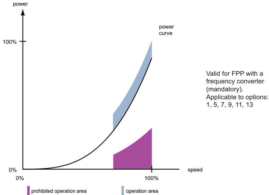
Figure 4-22 FPP with mandatory frequency converter
