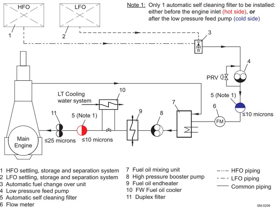
Figure 4-11 Fuel oil filter arrangement 'A'
