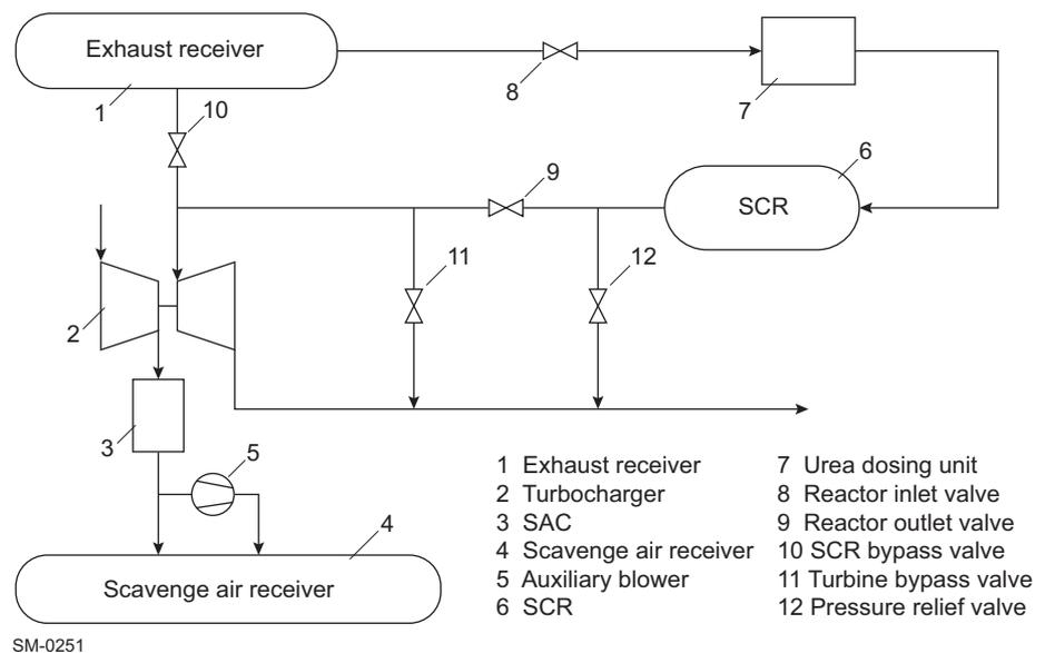
Figure 7-3 High-pressure SCR — arrangement
