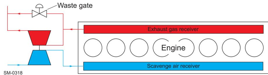
Figure 1-5 Schematic functional principle of an exhaust gas waste gate
