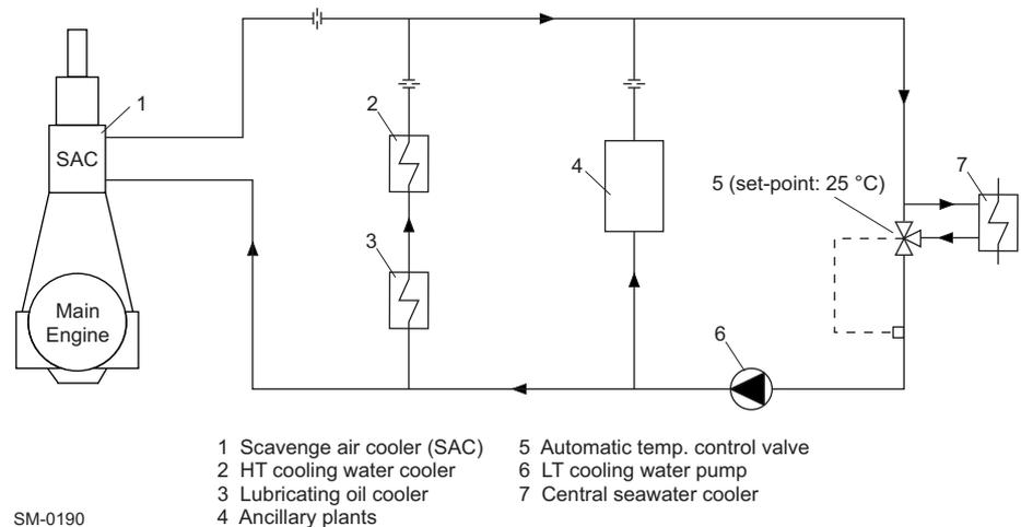
Figure 4-3 Scheme of cooling water system
