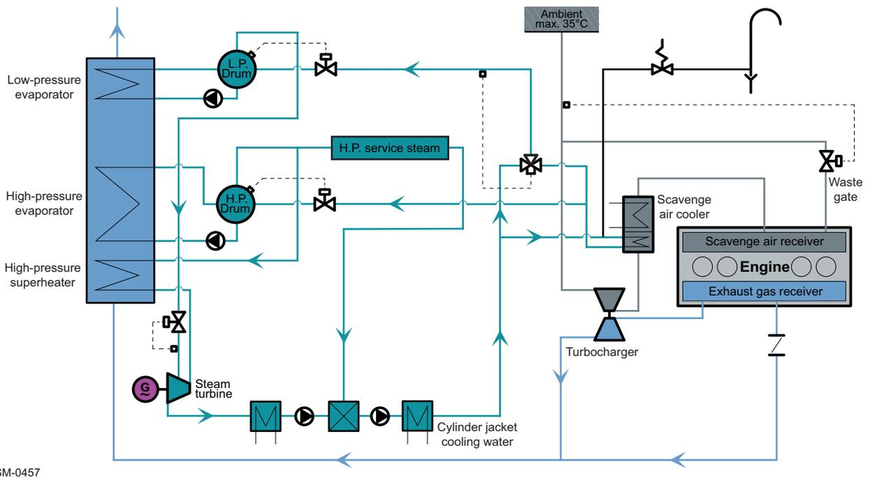
Figure 4-30 Dual-pressure steam system with HP superheater
