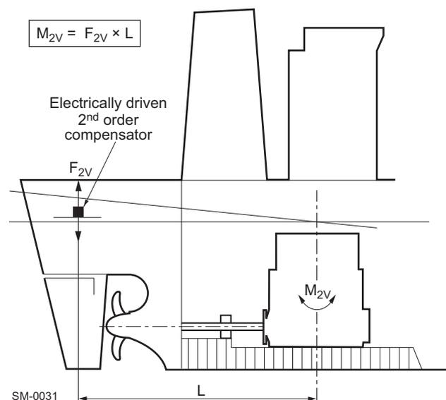
Figure 6-2 Locating an electrically driven compensator
