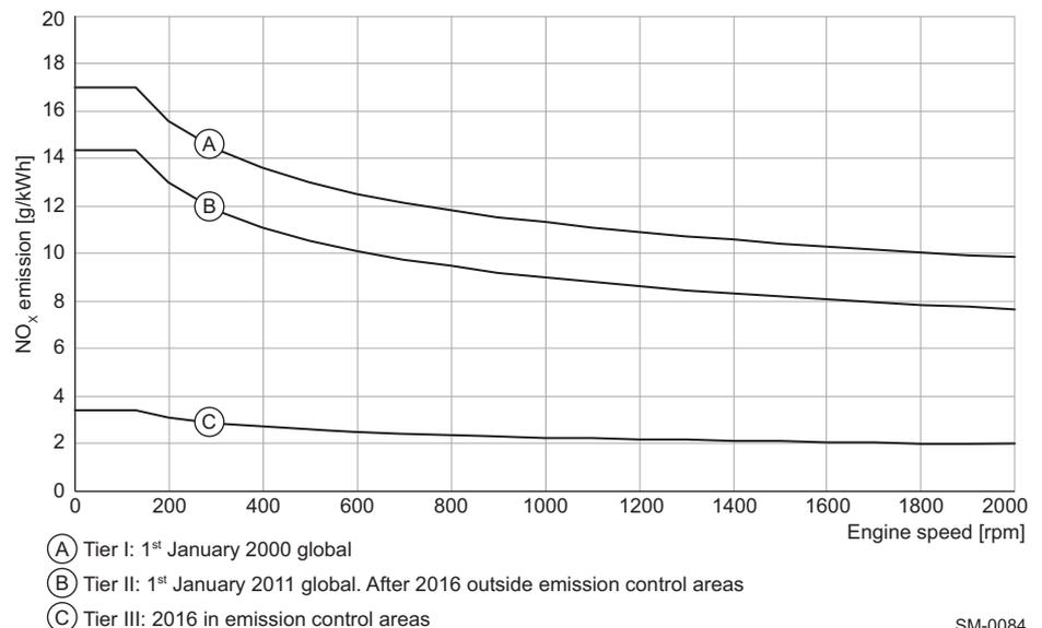
Figure 7-1 Speed dependent maximum allowable average of NO<sub>x</sub> emissions
