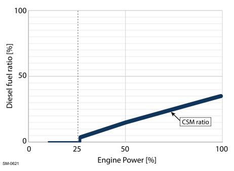
Figure 1-7 Diesel fuel ratio during active CSM
