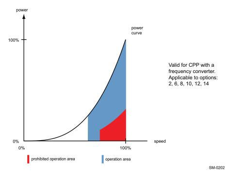
Figure 4-81 CPP in combination with an optional frequency converter
