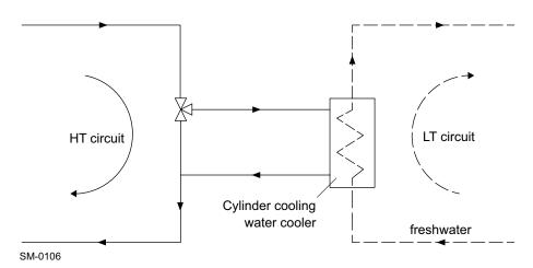
Figure 4-25 Separate HT cooling water circuit
