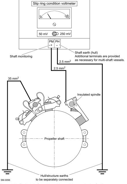
Figure 3-12 Typical shaft earthing with condition monitoring facility
