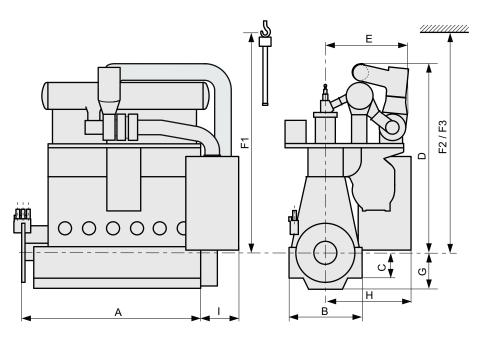
Figure 3-2 Engine dimensions with the iCER on-engine option
