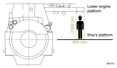
Figure 3-4 Minimum requirements for headroom
