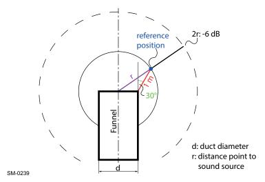
Figure 7-5 Exhaust noise reference point
