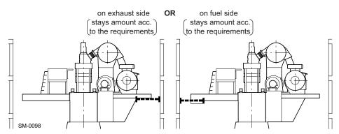
Figure 6-7 General arrangement of hydraulic type stays for one-side installation
