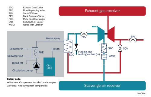
Figure 1-5 The iCER on-engine system
