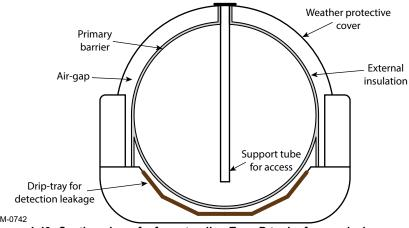
Figure 4-43 Section view of a free-standing Type B tank of moss design
