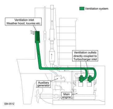
Figure 4-77 Ventilation system arrangement 2: Direct engine ventilation system
