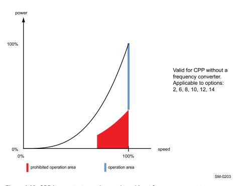
Figure 4-82 CPP in constant speed operation without frequency converter
