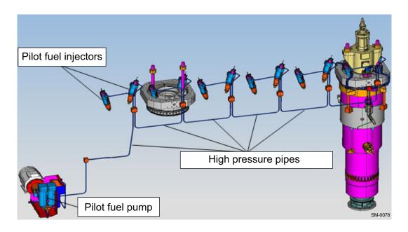
Figure 4-60 Pilot fuel high-pressure system
