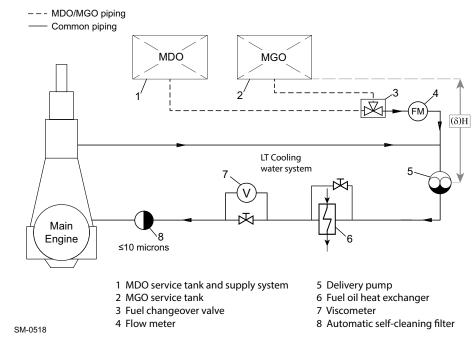
Figure 4-67 Fuel oil system — Arrangement with only MDO/MGO or MGO
