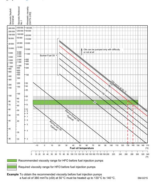
Figure 4-68 Fuel oil viscosity-temperature diagram
