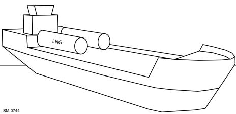
Figure 4-45 Type C tank on the deck of a vessel
