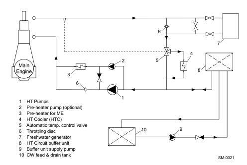
Figure 4-29 HT cooling water circuit
