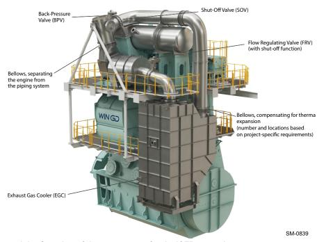
Figure 4-4 Overview of the components for the iCER on-engine system
