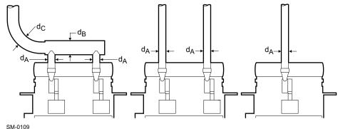
Figure 4-75 Determination of exhaust pipe diameter
