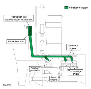
Figure 4-76 Ventilation system arrangement 1: Engine room ventilation system
