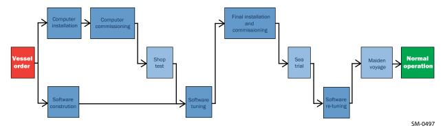
Figure 5-9 The WiDE installation process
