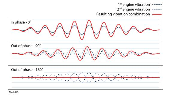
Figure 6-17 Resulting vibration from SPS combinations
