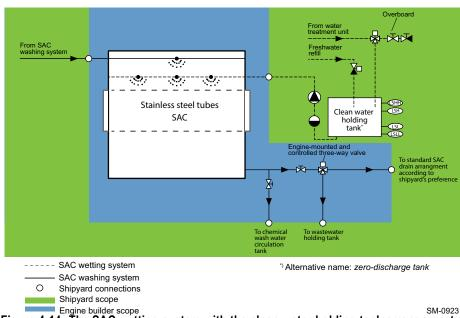
Figure 4-14 The SAC wetting system with the clean water holding tank arrangement
