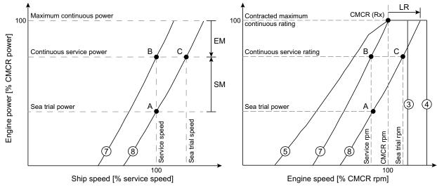
A Power and ship speed during sea-trials - light running and ideal sea condition
