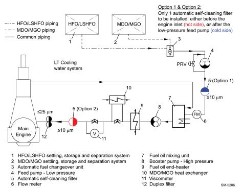
Figure 4-65 Fuel oil filter arrangement 'A'
