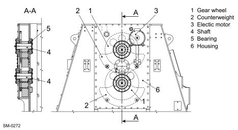
Figure 6-2 Major components and details of the iELBA
