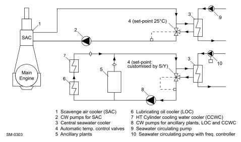
Figure 4-28 Separate SAC and LT cooling circuits
