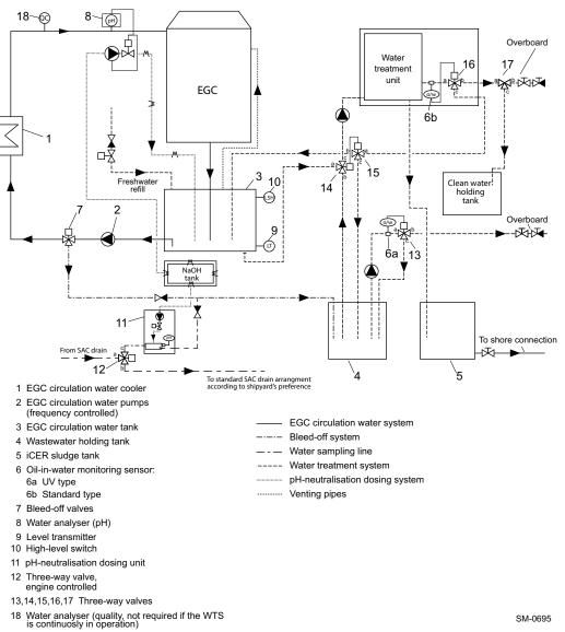
Figure 4-9 The iCER drainage system valid for all iCER operating mode options (onand off-engine option)
