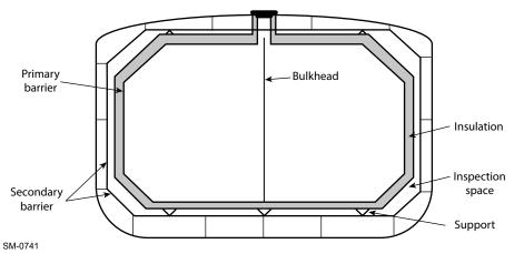
Figure 4-42 Section view of a free-standing Type A tank
