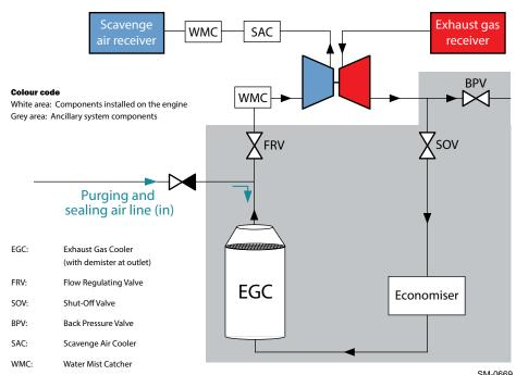
Figure 4-16 The iCER exhaust gas system (off-engine option) with the exhaust gas return pipe routed to the turbocharger connection from above
