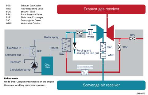
Figure 4-5 The iCER system (off-engine option) with the exhaust gas return pipe routed to the turbocharger connection from above
