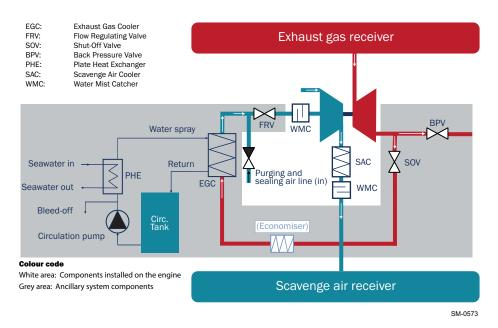
Figure 1-4 The iCER system (off-engine option) with the exhaust gas return pipe routed to the turbocharger connection from above
