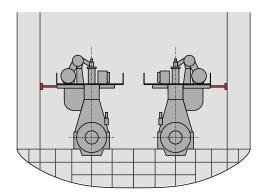
Installation of lateral stays on the exhaust side with:
