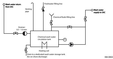
Figure 4-74 Offline SAC washing system (external system)
