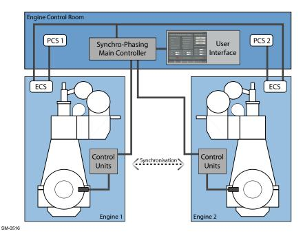
Figure 6-18 Synchro-Phasing System
