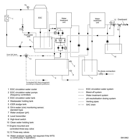
Figure 4-13 The unified iCER drainage system (on- and off-engine option) with a dedicated water treatment system for EGC circulation water cleaning and for bleed-off water cleaning
