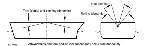
Figure 4-37 Inclination angles
