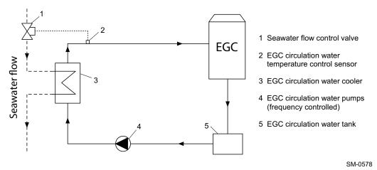
Figure 4-7 The EGC circulation water system (off-engine option)
