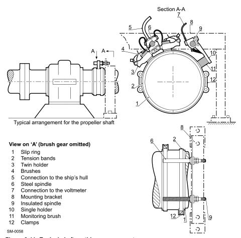
Figure 3-11 Typical shaft earthing arrangement
