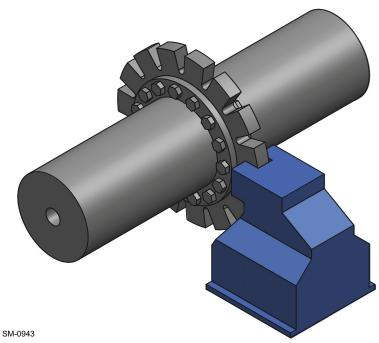
Figure 3-13 Example of a shaft-locking device
