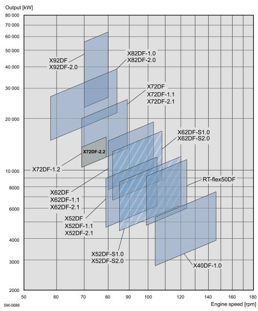
Figure 1-1 Power/speed range of the WinGD X-DF engines
