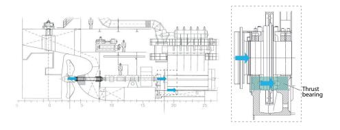
Figure 3-5 Force transmission to the engine foundation
