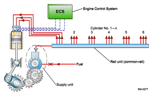
Figure 1-6 The Flex system parts
