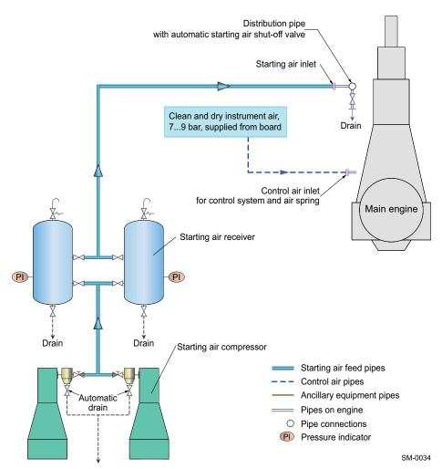
Figure 4-69 Air supply system
