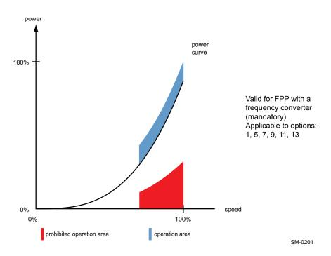
Figure 4-80 FPP with mandatory frequency converter
