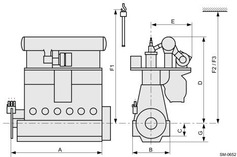
Figure 3-1 Engine dimensions with the iCER off-engine option
