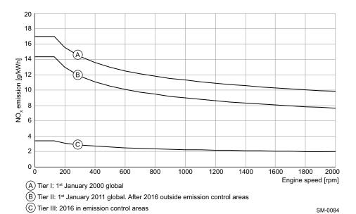
Figure 7-2 Speed dependent maximum allowable average of NO<sub>x</sub> emissions
