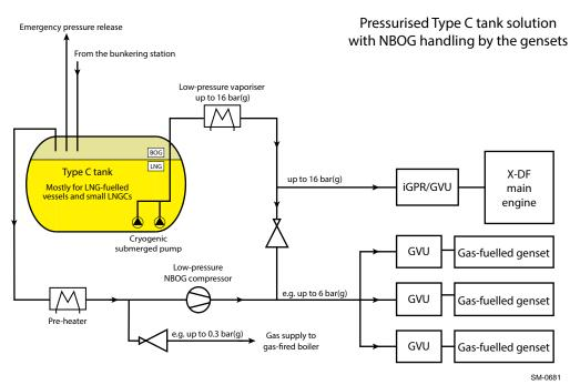
Figure 4-46 Pressurised Type C tank solution with NBOG handling by the gensets
