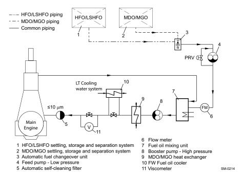
Figure 4-66 Fuel oil filter arrangement 'B'
