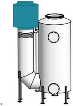
Figure 4-23 Arrangement of the additional economiser (Source: Alfa Laval)
