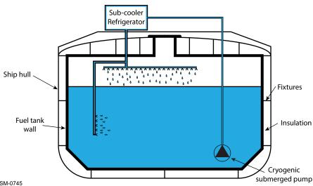
Figure 4-49 An LNG sub-cooler within an integrated tank
