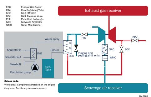
Figure 4-6 The iCER on-engine system
