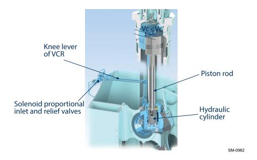
Figure 4-24 The VCR system components
