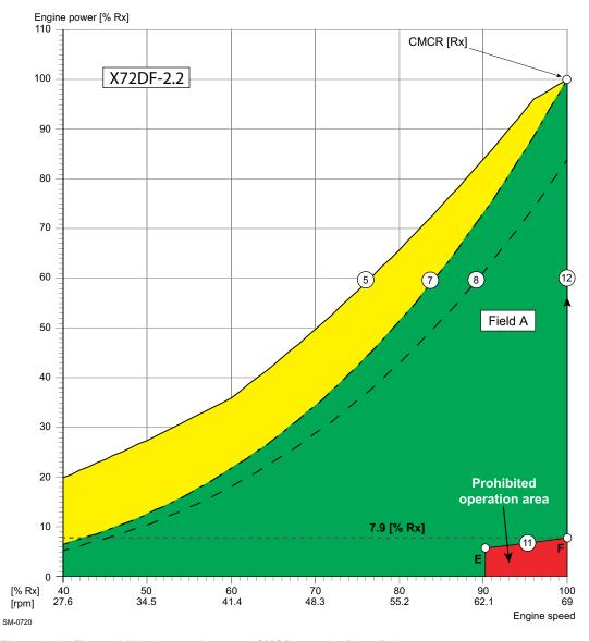
Figure 2-10 The prohibited operation area (CMCR speed = R3—R4)
