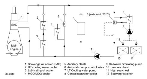
Figure 4-26 LT cooling water circuit — Single set-point temperature
