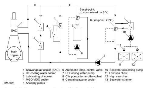
Figure 4-27 LT cooling water circuit — Dual set-point temperatures
