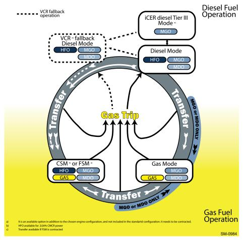
Figure 1-10 The fuel transfers and gas trips
