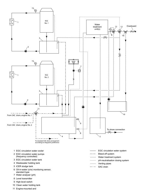
Figure 4-11 The unified iCER drainage system (on- and off-engine option) for the twin-engine installations
