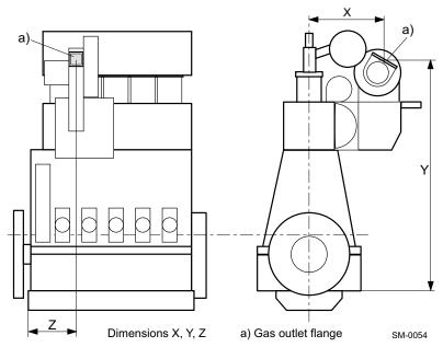
Figure 3-3 Thermal expansion, dim. X, Y, Z
