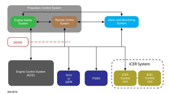
Figure 5-1 Engine automation architecture
