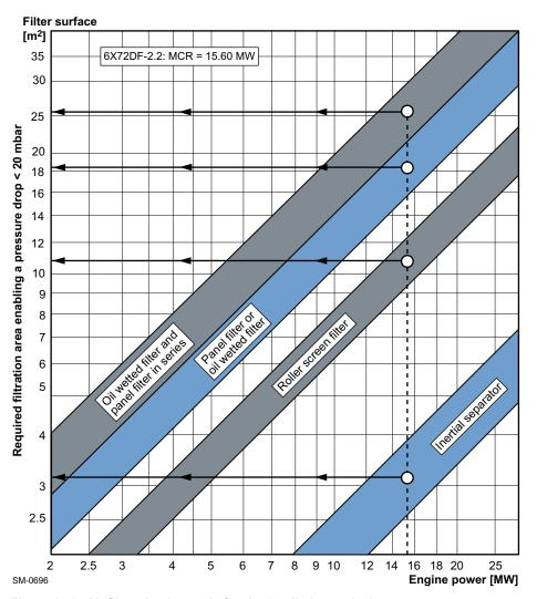
Figure 4-78 Air filter size (example for the 6-cylinder engine)
