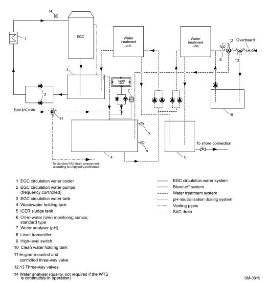
Figure 4-12 The unified iCER drainage system (on- and off-engine option) with a dedicated water treatment system for EGC circulation water refreshing and for bleed-off water cleaning
