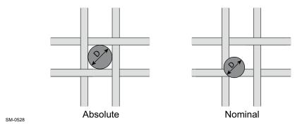
Figure 4-64 Mesh size difference between absolute and nominal
