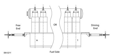
Figure 6-14 Arrangement of longitudinal stays
