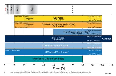
Figure 1-2 Operating modes of the engine
