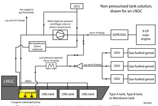
Figure 4-48 Non-pressurised tank solution, drawn for an LNGC
