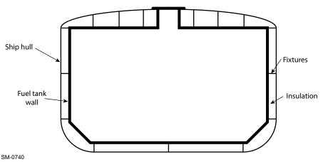
Figure 4-41 Section view of an integrated membrane tank
