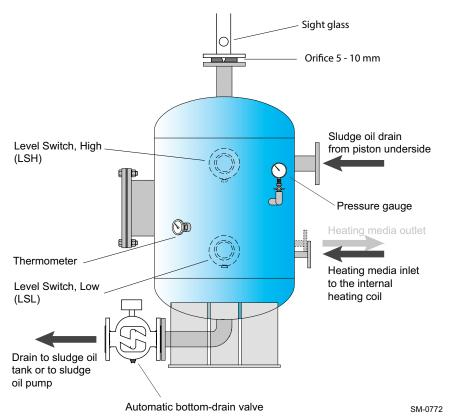
Figure 4-72 Design proposal of an automatically bottom-drained sludge oil trap
