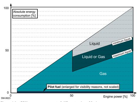
Figure 1-9 FSM — energy amount of different ratios of fuel
