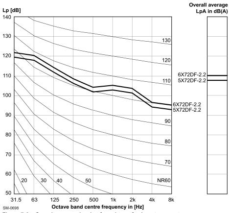
Figure 7-6 Sound pressure level at funnel top of exhaust gas system
