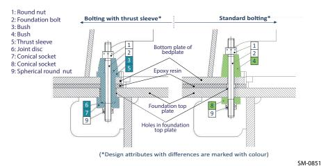
Figure 3-7 Foundation bolting
