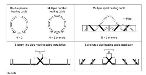
Figure 4-34 Trace heating cable arrangement
