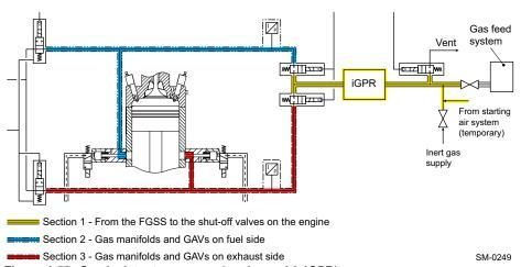
Figure 4-57 Gas leak test sequence (engines with iGPR)
