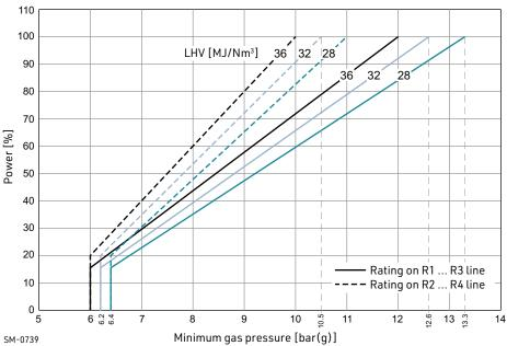
Figure 4-50 Design fuel gas supply pressure requirements
