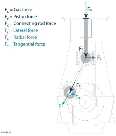
Figure 6-4 Forces through the engine
