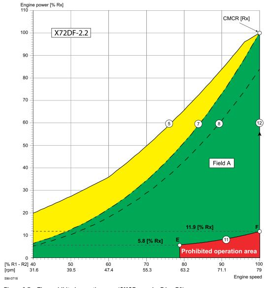
Figure 2-7 The prohibited operation area (CMCR speed = R1—R2)
