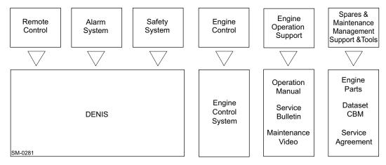
Figure 5-2 Engine management and automation concept
