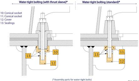
Figure 3-10 Proposed designs for water-tight bolting
