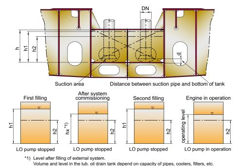
The oil volume in tank contains part of the oil quantity which drains back when the pumps sm-0037 are stopped.
