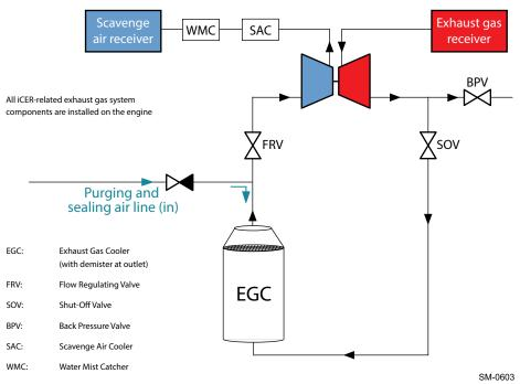
Figure 4-17 The iCER on-engine exhaust gas system
