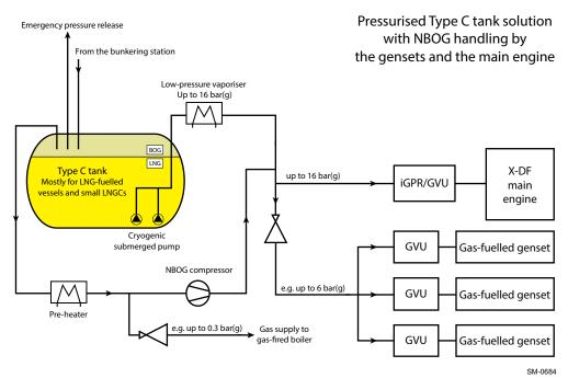
Figure 4-47 Pressurised Type C tank solution with NBOG handling by the gensets and the main engine
