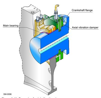
Figure 6-16 Example of axial vibration damper
