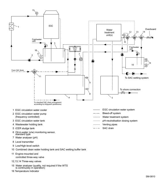
Figure 4-10 A new variant of the unified iCER drainage system (on- and off-engine option)
