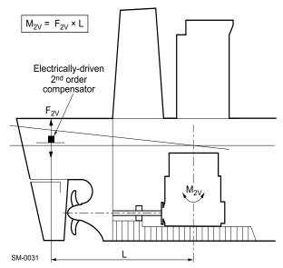
Figure 6-3 Location of an electrically-driven compensator
