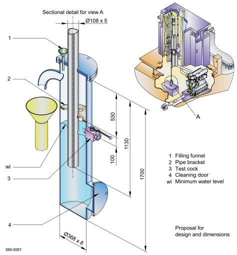
Figure 4-73 Arrangement of automatic water drain
