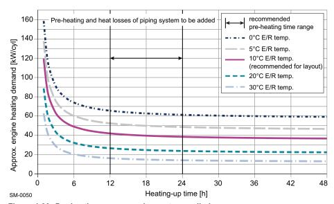
Figure 4-30 Pre-heating power requirement per cylinder
