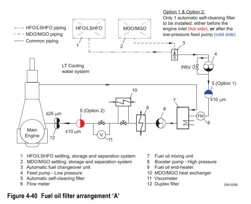
The automatic self-cleaning filter of maximum  $10\,\mu$ m abs. is used to protect the engine against serious damage. It captures the catalytic fines which were not removed by the fuel oil separator. In addition, the filter provides a good indication of the separator's efficiency.
