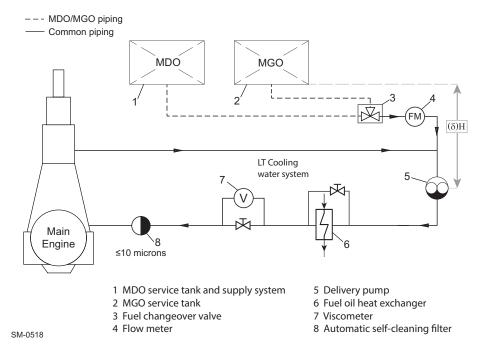
Figure 4-42 Fuel oil system — Arrangement with only MDO/MGO or MGO
