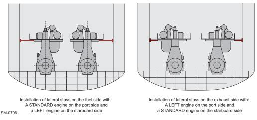
Figure 6-10 Variants of twin-engine installations with a standard and a left engine
