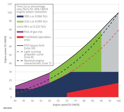
Figure 4-59 Maximum power decrease rate for PTO application in gas mode
