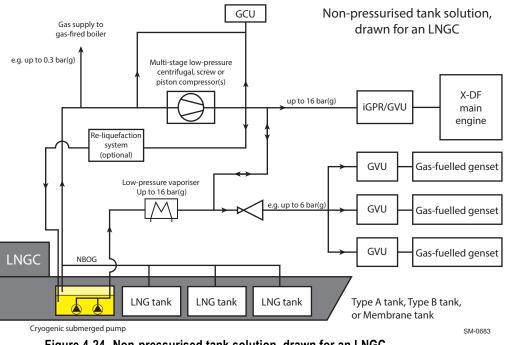
Figure 4-24 Non-pressurised tank solution, drawn for an LNGC
