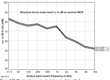
Figure 7-10 Structure-borne noise level at engine feet vertical
