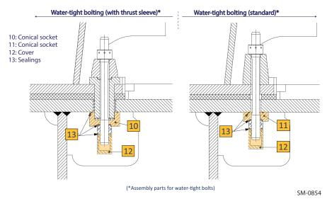
Figure 3-9 Proposed designs for water-tight bolting
