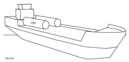
Figure 4-21 Type C tank on the deck of a vessel
