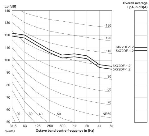
Figure 7-9 Sound pressure level at funnel top of exhaust gas system
