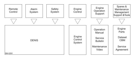
Figure 5-2 Engine management and automation concept
