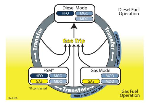
Figure 1-7 Fuel transfers and gas trips
