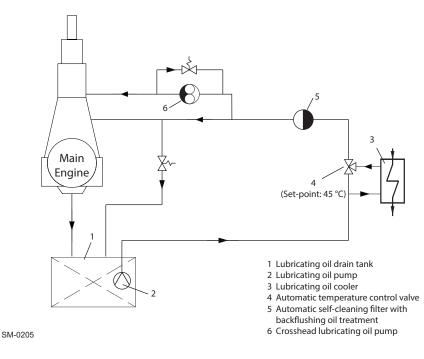
Figure 4-8 Lubricating oil system
