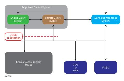
Figure 5-1 Engine automation architecture
