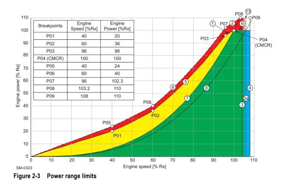
Line 1 100% Torque Limit Constant MEP or torque line through CMCR from 100% (speed and power) down to 96% (speed and power).
