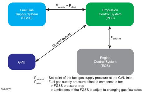
Figure 4-28 Fuel gas supply pressure control at the GVU inlet (engines with GVU)
