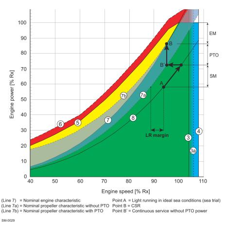
Figure 2-4 Power range diagram of an engine with a PTO
