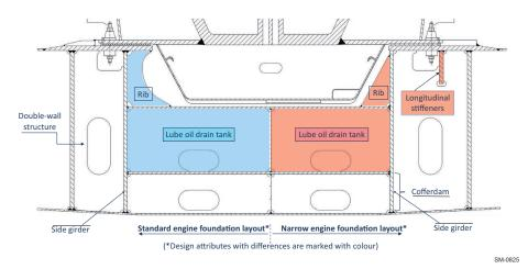
Figure 3-5 A comparison of the standard and narrow engine foundation layout
