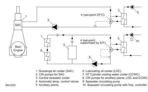
Figure 4-5 Separate SAC and LT cooling circuits
