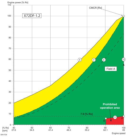
Figure 2-10 The prohibited operation area (CMCR speed = R3—R4)
