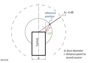
Figure 7-8 Exhaust noise reference point
