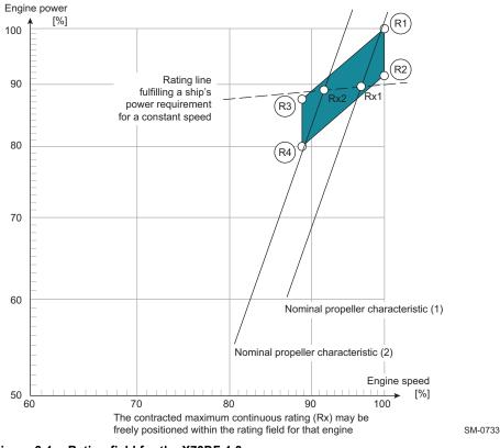
Figure 2-1 Rating field for the X72DF-1.2
