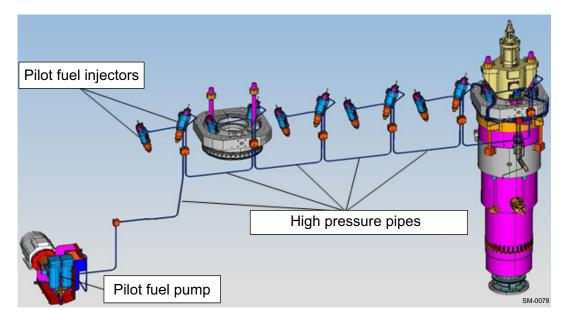
Figure 4-36 Pilot fuel high-pressure system
