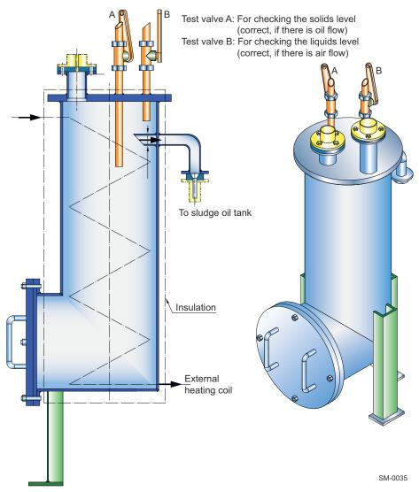
Figure 4-45 Design proposal of WinGD's sludge oil trap
