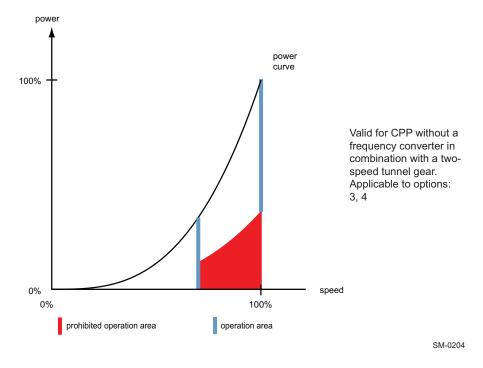
Figure 4-57 CPP with two fixed operation speeds without frequency converter
