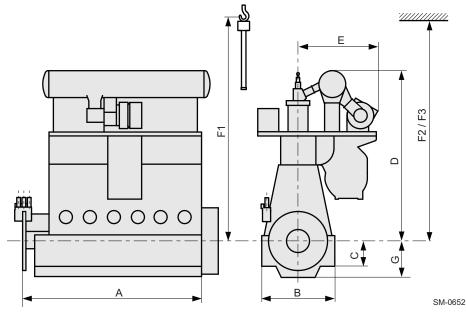
Figure 3-1 Engine dimensions
