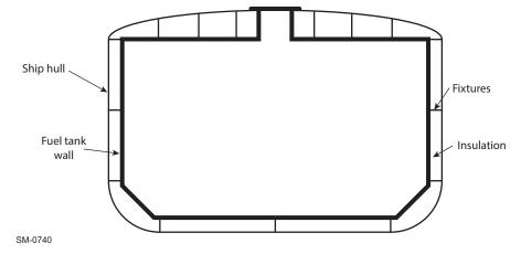
Figure 4-17 Section view of an integrated membrane tank
