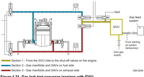
Figure 4-34 Gas leak test sequence (engines with GVU)
