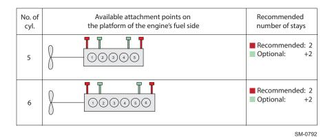
Figure 6-12 Engine stays arrangement on the engine's fuel side
