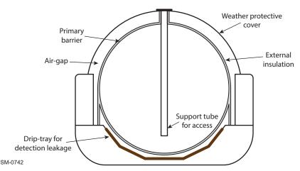
Figure 4-19 Section view of a free-standing Type B tank of moss design
