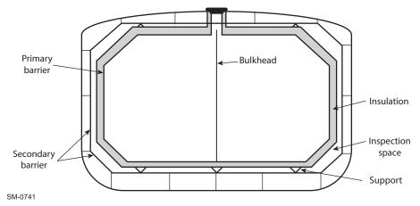
Figure 4-18 Section view of a free-standing Type A tank
