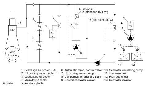
Figure 4-4 LT cooling water circuit — Dual set-point temperatures
