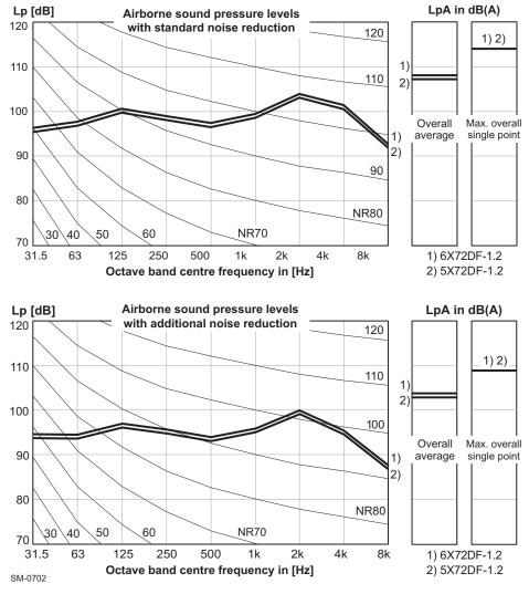
Figure 7-7 Sound pressure level at 1m distance from engine
