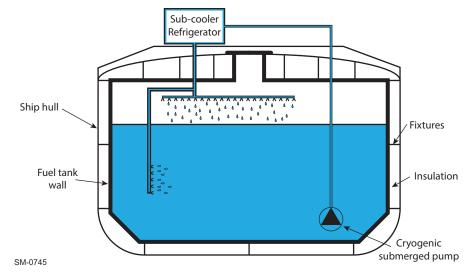
Figure 4-25 An LNG sub-cooler within an integrated tank
