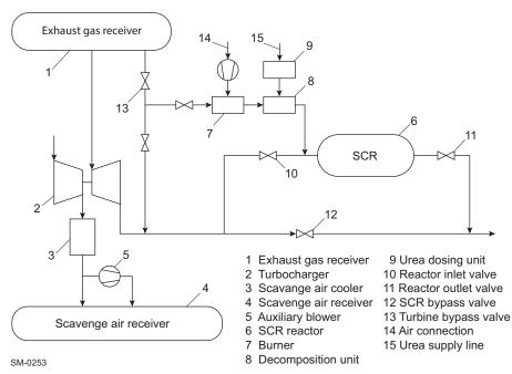
Figure 7-6 Low-pressure SCR with indirect urea injection (bypass rate controlled)
