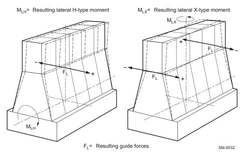
Figure 6-5 Lateral vibration — X-type and H-type
