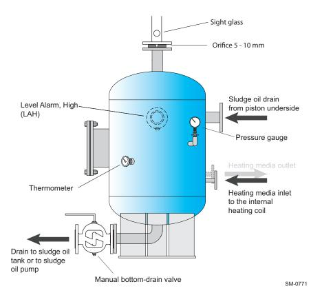
Figure 4-46 Design proposal of a manually bottom-drained sludge oil trap
