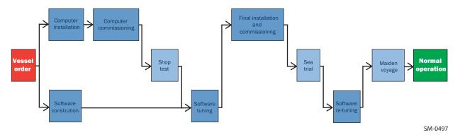
Figure 5-9 The WiDE installation process
