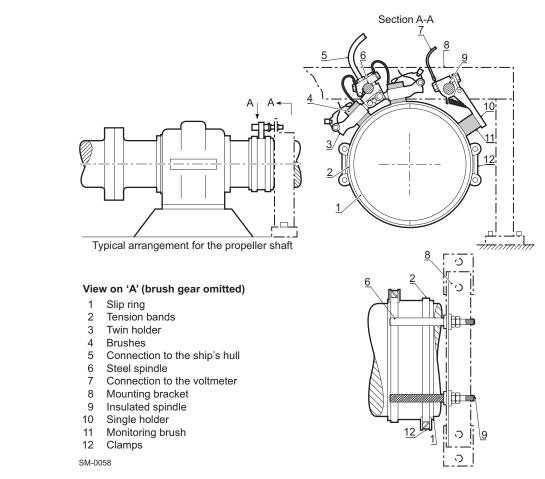
Figure 3-10 Typical shaft earthing arrangement
