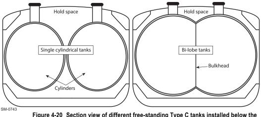
Figure 4-20 Section view of different free-standing Type C tanks installed below the deck
