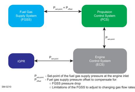
Figure 4-27 Fuel gas supply pressure control at the engine inlet (engines with iGPR)
