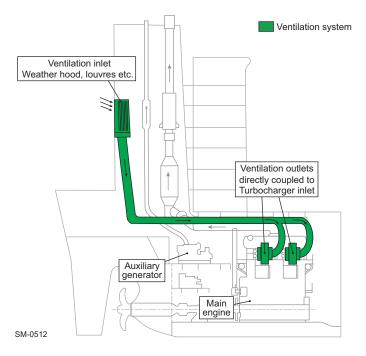
Figure 4-51 Ventilation system arrangement 2 — Direct engine ventilation system
