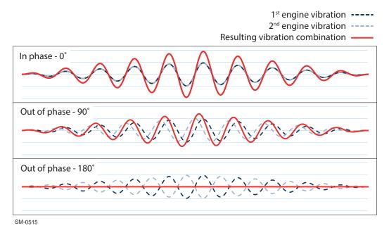
Figure 6-17 Resulting vibration from SPS combinations
