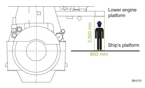
Figure 3-3 Minimum requirements for headroom
