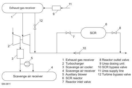
Figure 7-4 Low-pressure SCR with direct urea injection
