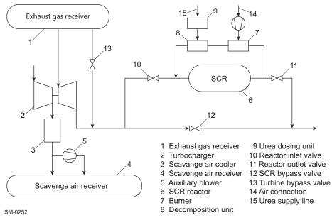
Figure 7-5 and Figure 7-6 include sketches of LP SCR with the indirect urea injection system.
