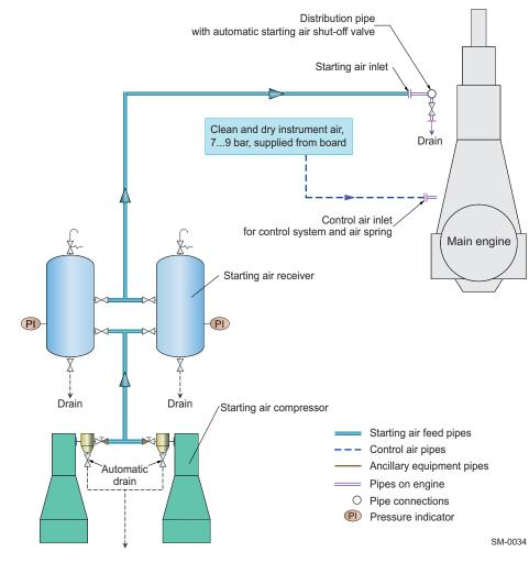
Figure 4-44 Air supply system
