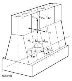
$\begin{array}{ll} F_{1V} & \mbox{Resulting first order vertical mass force} \\ F_{1H} & \mbox{Resulting first order horizontal mass force} \\ F_{2V} & \mbox{Resulting second order vertical mass force} \\ F_{4V} & \mbox{Resulting fourth order vertical mass force} \\ M_{1V} & \mbox{First order vertical mass moment} \\ M_{1H} & \mbox{First order horizontal mass moment} \\ M_{2V} & \mbox{Second order vertical mass moment} \\ M_{4V} & \mbox{Fourth order vertical mass moment} \\ \end{array}$
