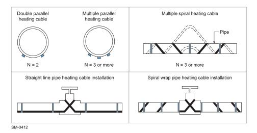
Figure 4-11 Trace heating cable arrangement
