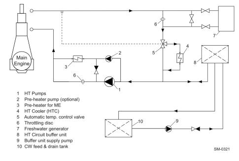
Figure 4-6 HT cooling water circuit
