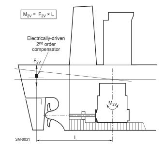
Figure 6-3 Locating an electrically-driven compensator
