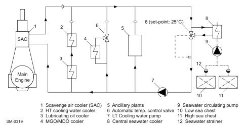
Figure 4-3 LT cooling water circuit — Single set-point temperature
