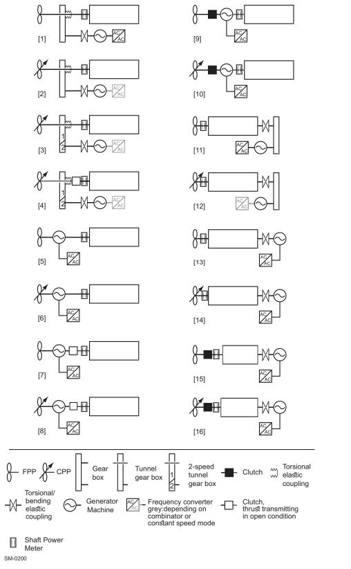
Figure 4-53 Arrangements for PTO, PTI, PTH
