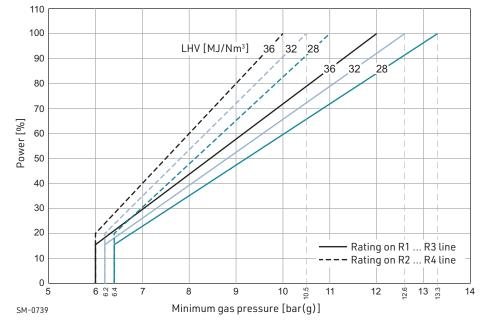
Figure 4-26 Design fuel gas supply pressure requirements
