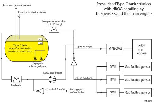
Figure 4-23 Pressurised Type C tank solution with NBOG handling by the gensets and the main engine
