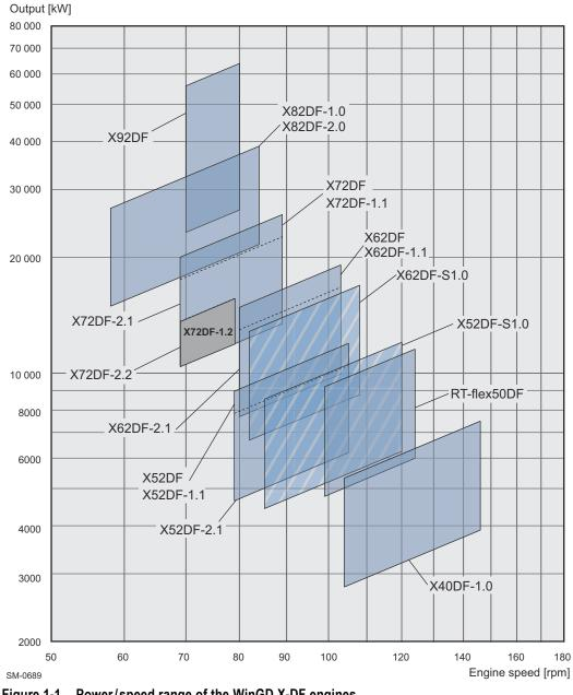
Power/speed range of the WinGD X-DF engines Figure 1-1
