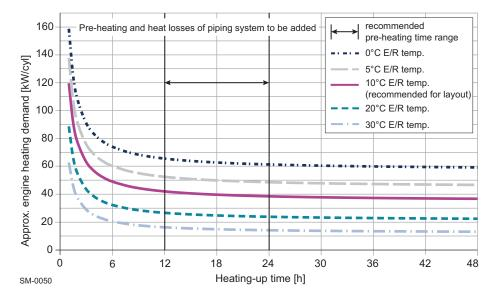
Figure 4-7 Pre-heating power requirement per cylinder
