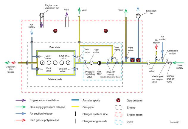
Figure 4-30 Fuel gas supply system with the iGPR
