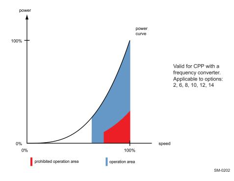
Figure 4-55 CPP in combination with an optional frequency converter
