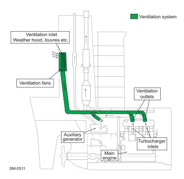
Figure 4-50 Ventilation system arrangement 1 — Engine room ventilation system
