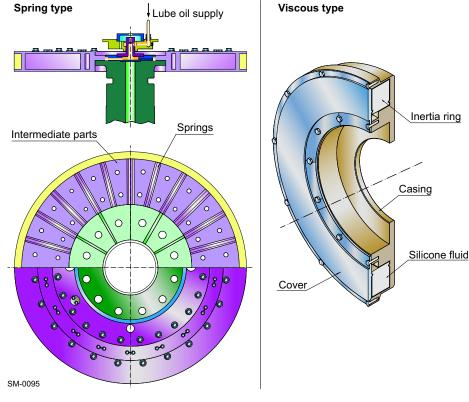
Figure 6-15 Vibration dampers (spring type and viscous type)
