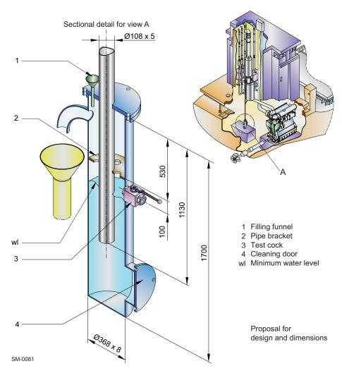
Figure 4-48 Arrangement of automatic water drain
