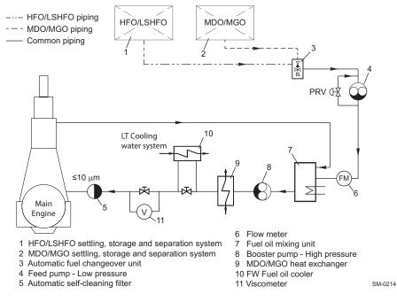
Figure 4-41 Fuel oil filter arrangement 'B'
