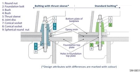
Figure 3-6 Foundation bolting
