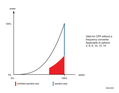
Figure 4-56 CPP in constant speed operation without frequency converter
