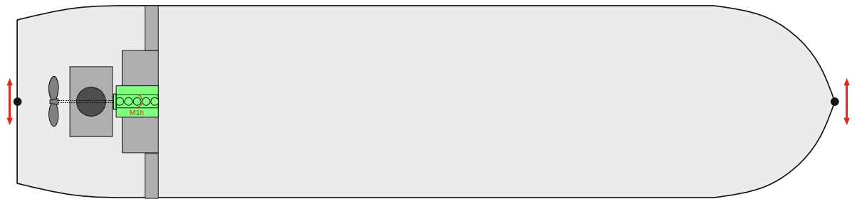
Horizontal hull girder vibrations due to M_{1h}
