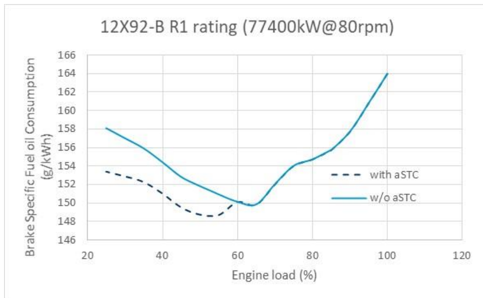
Figure 2-1 Fuel consumption savings with the aSTC option as a function of engine power
