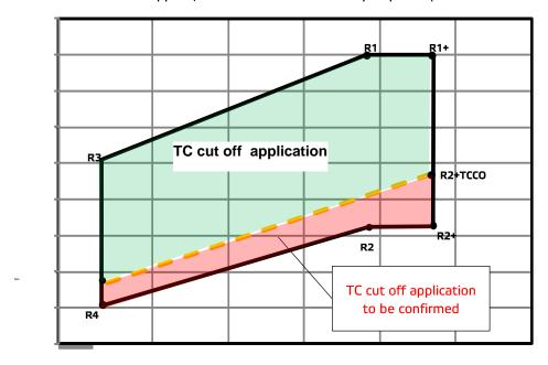
Figure 2: Summary of limitations to TC cut-off application for Wärtsilä engines
