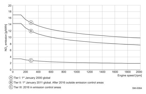
Figure 7-1 Speed dependent maximum allowable average of NO<sub>x</sub> emissions
