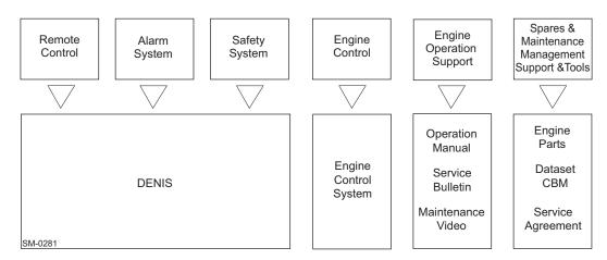
Figure 5-2 Engine management and automation concept
