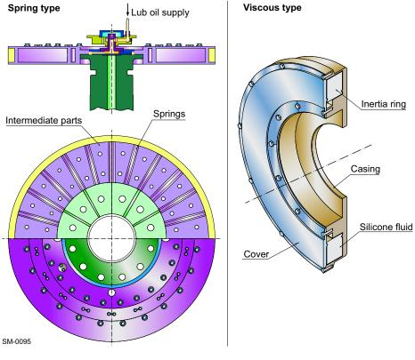
Figure 6-8 Vibration dampers (spring type and viscous type)
