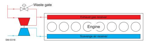
Figure 1-6 Functional principle of an exhaust gas waste gate
