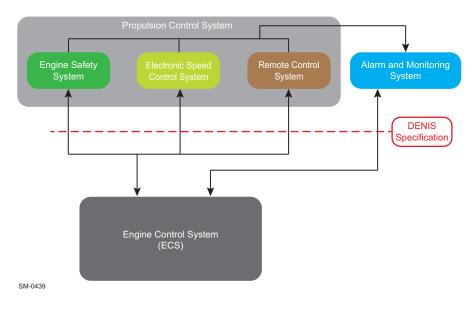
Figure 5-1 Engine automation architecture
