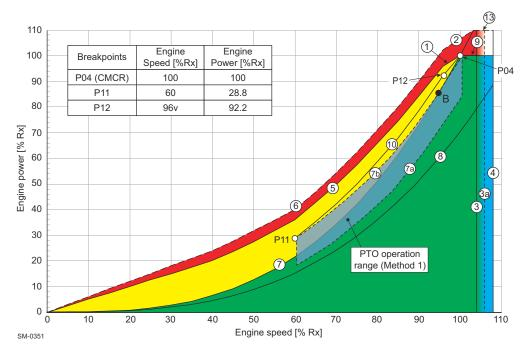
Figure 2-5 Power range limits for PTO operation — Method 1
