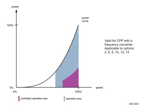
Figure 4-24 CPP in combination with an optional frequency converter
