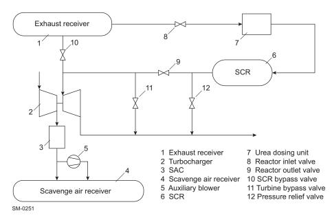
Figure 7-3 High-pressure SCR — Arrangement
