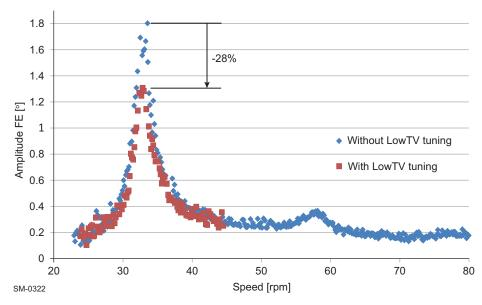
Figure 1-9 Vibration amplitudes - Achievements with default LowTV tuning
