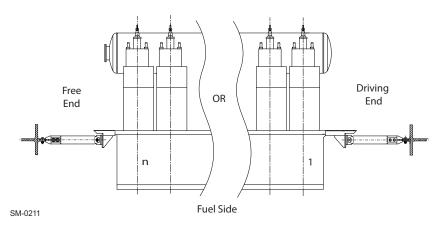
Figure 6-7 Arrangement of longitudinal stays
