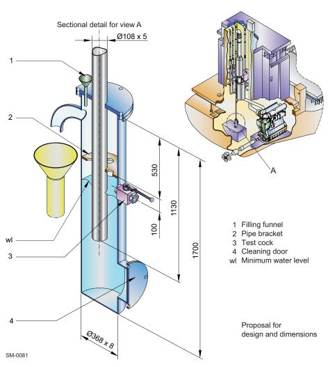
Figure 4-17 Arrangement of automatic water drain
