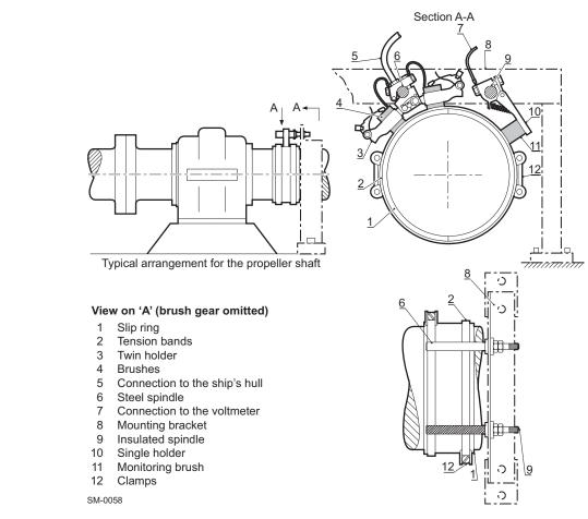
Figure 3-4 Typical shaft earthing arrangement
