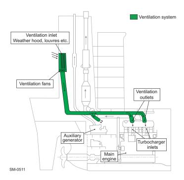
Figure 4-19 Ventilation system arrangement 1 — Engine room ventilation system
