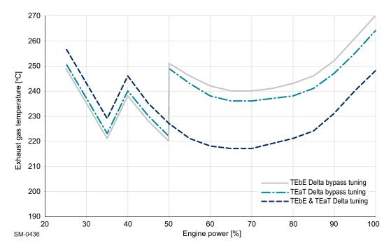
Figure 1-7 Exhaust gas temperature increase with DBT
