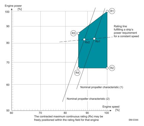
Figure 2-1 Rating field for RT-flex58T-E
