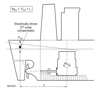
Figure 6-2 Locating an electrically driven compensator
