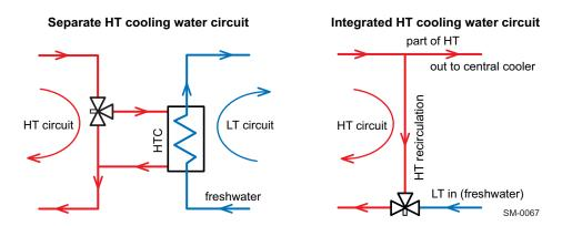
Figure 4-4 Principal layouts of HT cooling water circuit
