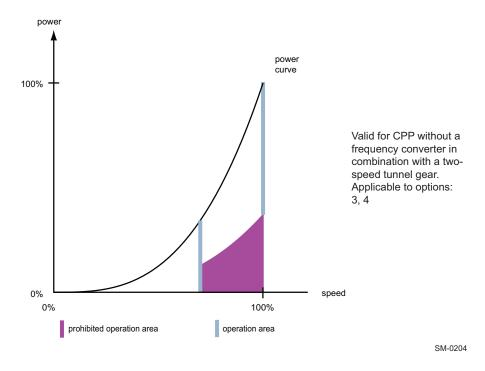
Figure 4-26 CPP with two fixed operation speeds without frequency converter
