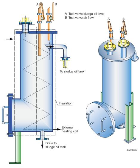
Figure 4-16 Sludge oil trap
