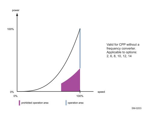
Figure 4-25 CPP in constant speed operation without frequency converter
