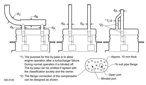
Figure 4-18 Determination of exhaust pipe diameter
