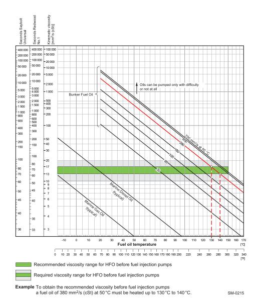
Figure 4-14 Fuel oil viscosity-temperature diagram
