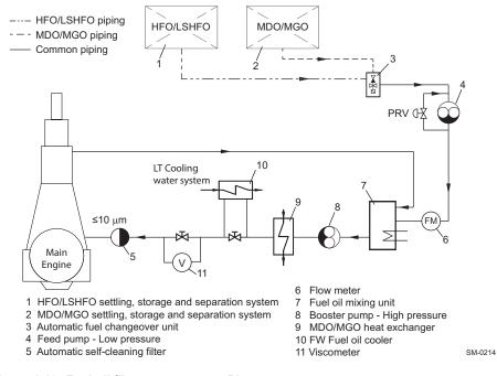
Figure 4-13 Fuel oil filter arrangement 'B'
