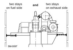
Figure 6-6 General arrangement of hydraulic stays for both-side installation
