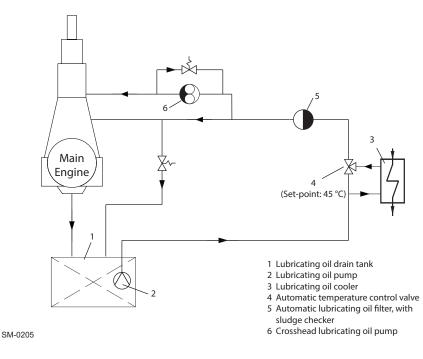
Figure 4-6 Lubricating oil system
