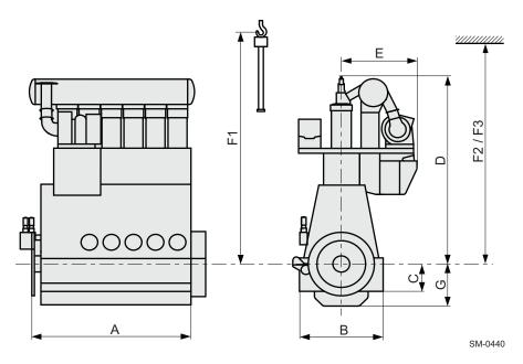
Figure 3-1 Engine dimensions
