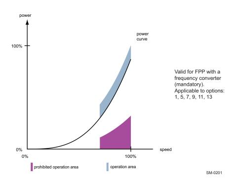
Figure 4-23 FPP with mandatory frequency converter
