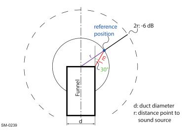
Figure 7-5 Exhaust noise reference point
