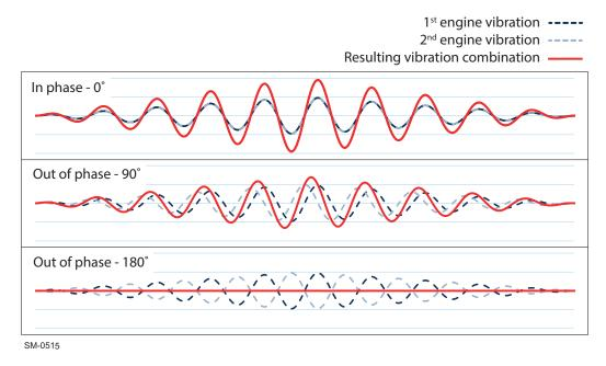
Figure 6-10 Resulting vibration from SPS combinations
