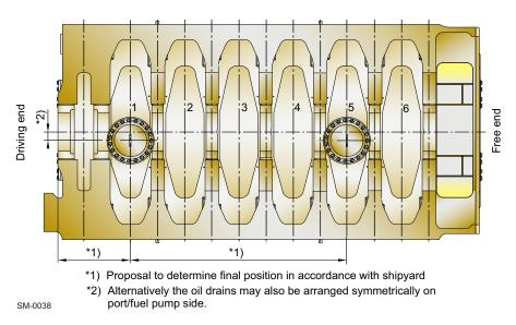
Figure 4-8 Arrangement of vertical lubricating oil drains for 6-cylinder engines
