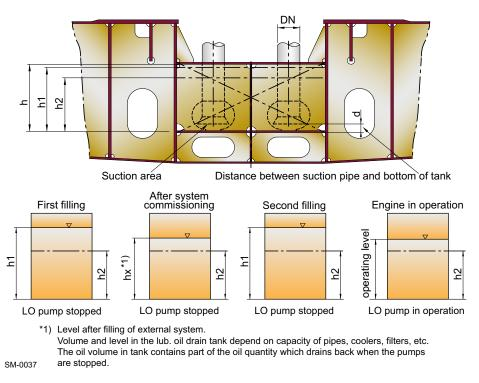
Figure 4-7 Dimensioning and filling process of lubricating oil drain tank
