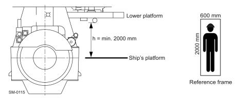
Figure 3-3 Minimum requirements for headroom
