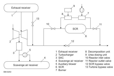
Figure 7-2 Low-pressure SCR — Arrangement
