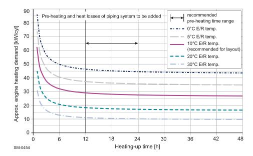
Figure 4-5 Pre-heating power requirement per cylinder
