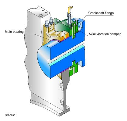
Figure 6-9 Example of axial vibration damper
