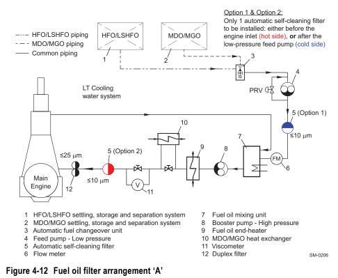
The automatic self-cleaning filter of maximum 10µm abs. is used to protect the
