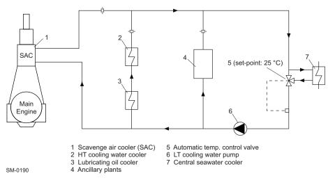
Figure 4-3 Scheme of cooling water system
