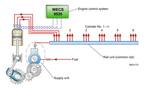
Figure 1-11 Flex system parts
