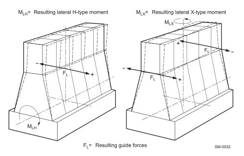
Figure 6-4 Lateral vibration — X-type and H-type
