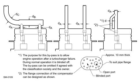
Figure 4-40 Determination of exhaust pipe diameter
