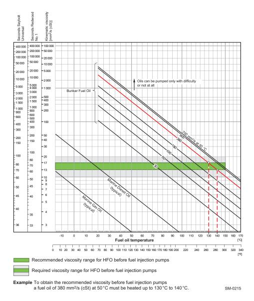
Figure 4-21 Fuel oil viscosity-temperature diagram
