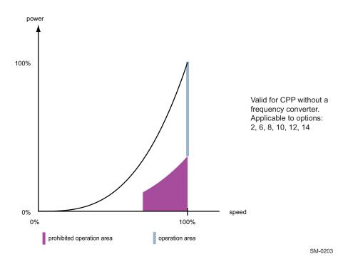
Figure 4-47 CPP in constant speed operation without frequency converter
