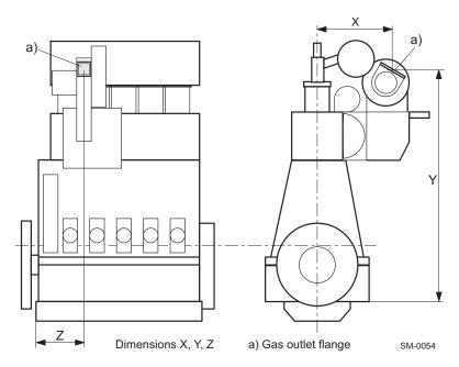
Figure 3-2 Thermal expansion, dim. X, Y, Z
