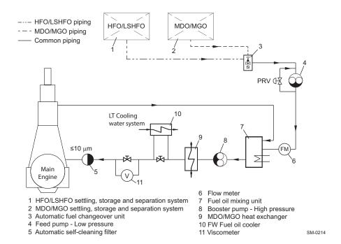
Figure 4-19 Fuel oil filter arrangement 'B'
