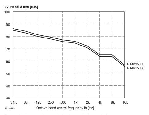
Figure 7-6 Structure-borne noise level at engine feet vertical
