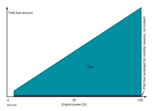
Figure 1-4 Gas mode operation
