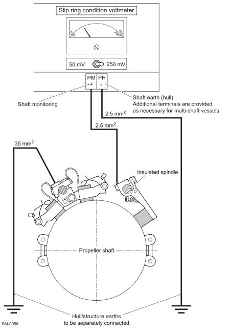
Figure 3-5 Typical shaft earthing with condition monitoring facility
