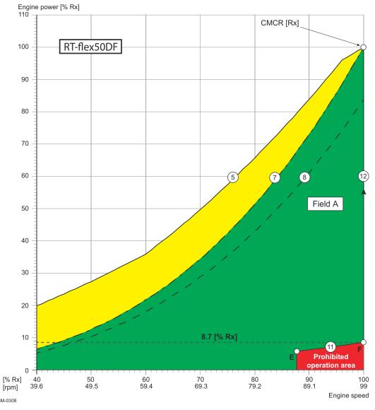
Figure 2-10 Prohibited engine operation area (CMCR speed = R3—R4)
