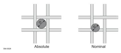
Figure 4-17 Mesh size difference between absolute and nominal
