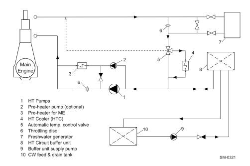
Figure 4-8 HT cooling water circuit
