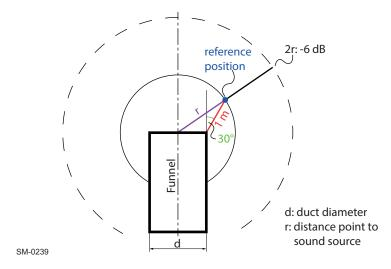
Figure 7-4 Exhaust noise reference point
