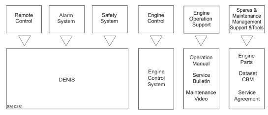
Figure 5-2 Engine management and automation concept
