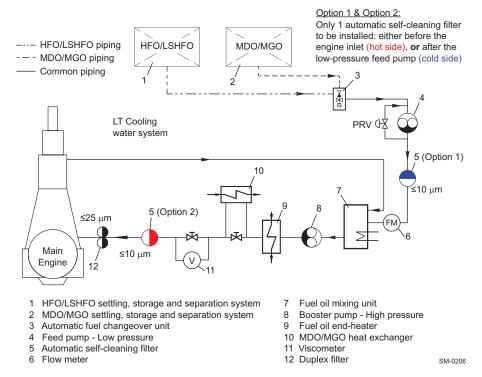
Figure 4-18 Fuel oil filter arrangement 'A'
