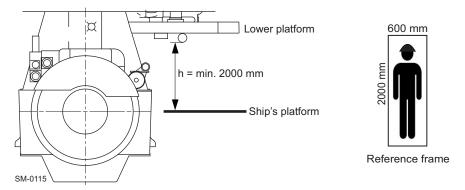
Figure 3-3 Minimum requirements for headroom
