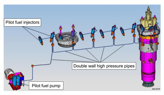
Figure 4-23 Pilot fuel high-pressure system
