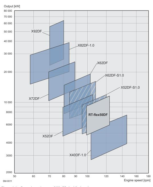
Figure 1-1 Power/speed range of WinGD dual-fuel engines
