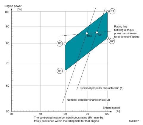
Figure 2-1 Rating field for RT-flex50DF
