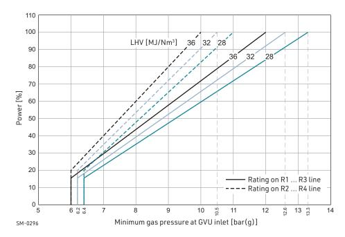
Figure 4-26 Design gas feed pressure requirements (engines with GVU)
