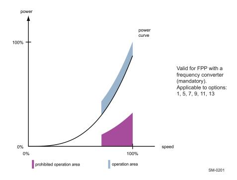
Figure 4-45 FPP with mandatory frequency converter
