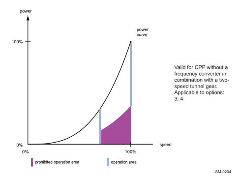
Figure 4-48 CPP with two fixed operation speeds without frequency converter
