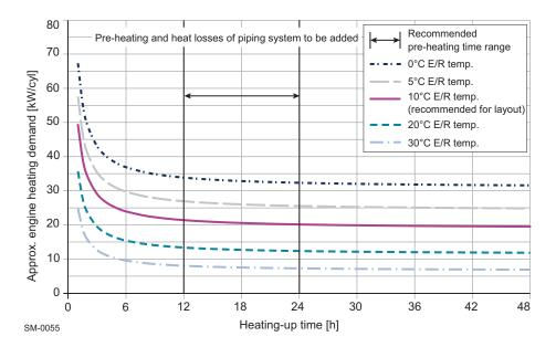
Figure 4-9 Pre-heating power requirement per cylinder
