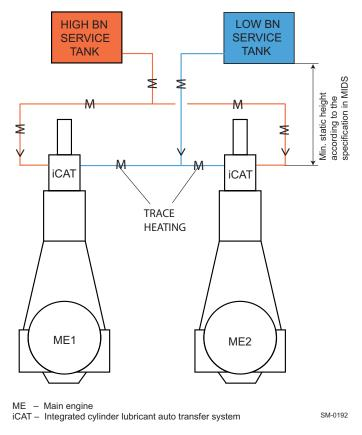
Figure 4-2 Cylinder LO system with iCAT for variable sulphur content in fuel
