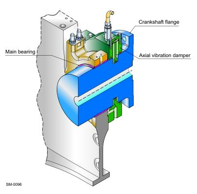
Figure 6-9 Example of axial vibration damper
