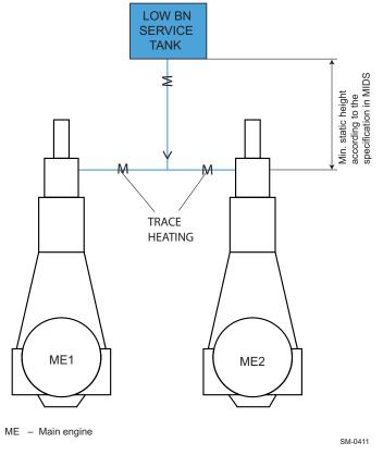
Figure 4-3 Cylinder LO system for fuel with ultra low sulphur content (max. 0.1%)
