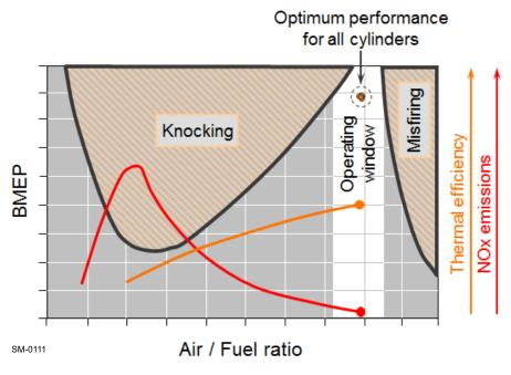
Figure 4-25 Lean-burn operation window (engines with GVU)
