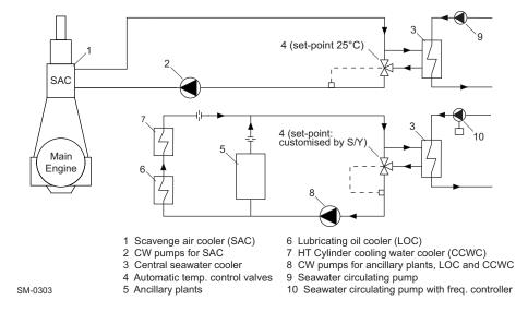
Figure 4-7 Separate SAC and LT cooling circuits
