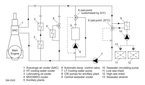
Figure 4-6 LT cooling water circuit — dual set-point temperatures
