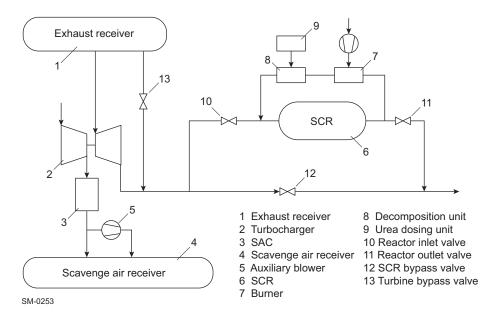
Figure 7-2 Low-pressure SCR — Arrangement
