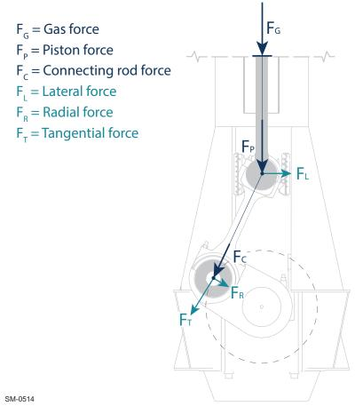
Figure 6-3 Forces through the engine
