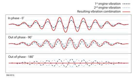
Figure 6-10 Resulting vibration from SPS combinations
