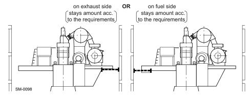
Figure 6-5 General arrangement of hydraulic stays for one-side installation
