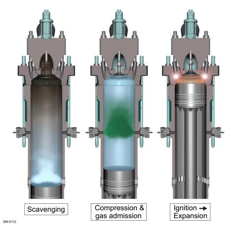
Figure 4-31 Lean burn with pilot ignition (engines with iGPR)
