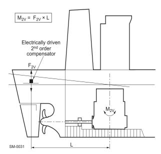
Figure 6-2 Locating an electrically driven compensator
