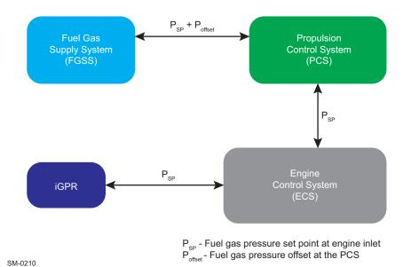
Figure 4-34 Fuel gas pressure control at engine inlet (engines with iGPR)
