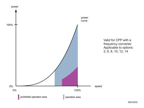
Figure 4-46 CPP in combination with an optional frequency converter
