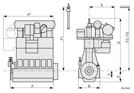
Figure 3-1 Engine dimensions
