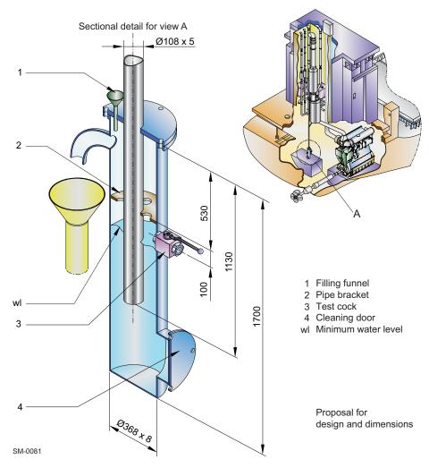
Figure 4-39 Arrangement of automatic water drain
