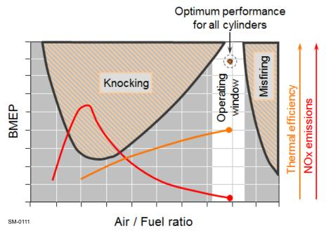
Figure 4-32 Lean-burn operation window (engines with iGPR)
