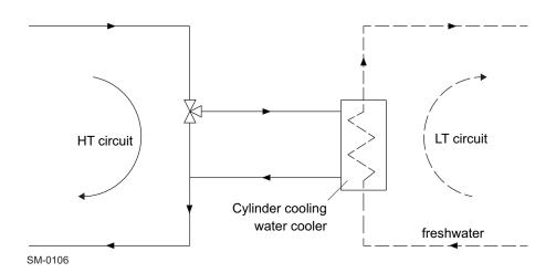
Figure 4-4 Separate HT cooling water circuit
