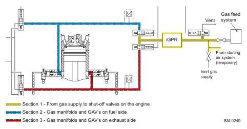
Figure 4-36 Gas leak test sequence (engines with iGPR)
