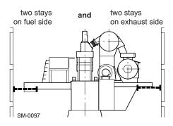
Figure 6-6 General arrangement of hydraulic stays for both-side installation
