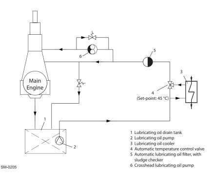
Figure 4-10 Lubricating oil system
