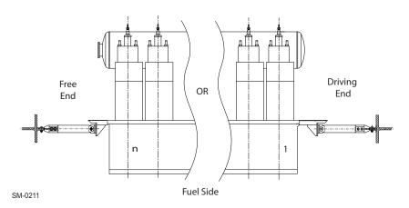
Figure 6-7 Arrangement of longitudinal stays
