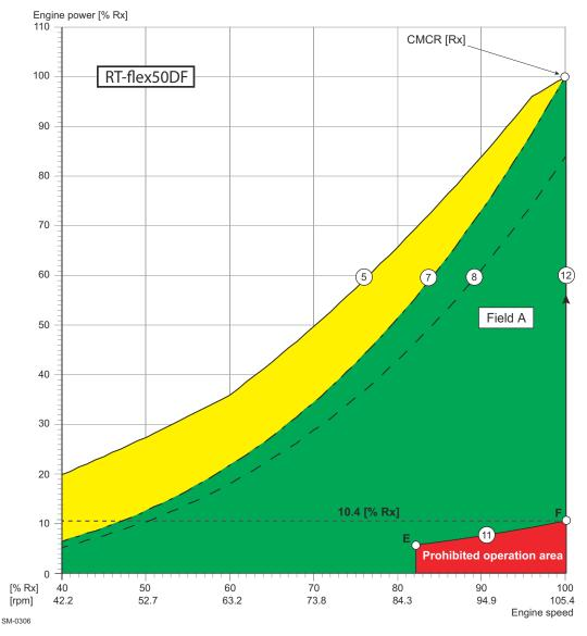
Figure 2-9 Prohibited engine operation area (CMCR speed = 85% of R1—R2)
