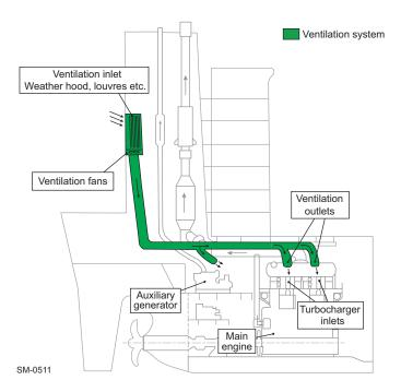
Figure 4-41 Ventilation system arrangement 1 — Engine room ventilation system
