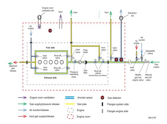
Figure 4-35 Gas system with iGPR
