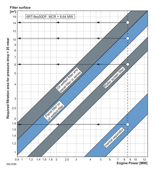
Figure 4-43 Air filter size (example for 6-cyl. engine)
