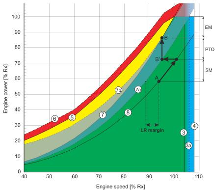
Figure 2-4 Power range diagram of an engine with main-engine driven generator
