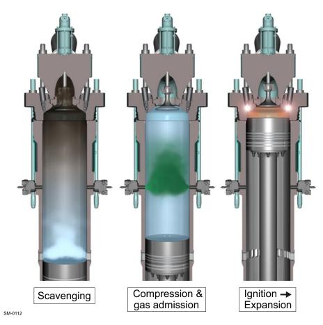
Figure 4-24 Lean burn with pilot ignition (engines with GVU)
