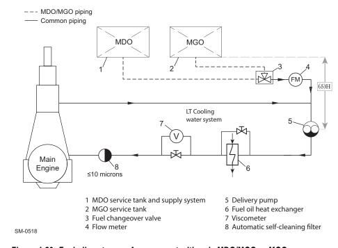
Figure 4-20 Fuel oil system — Arrangement with only MDO/MGO or MGO
