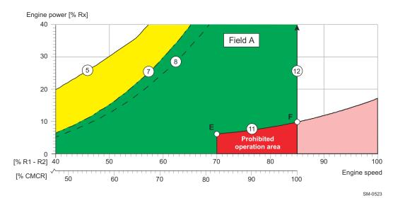
Figure 2-8 Calculating prohibited operation area for CMCR speed
