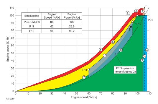
Figure 2-6 Power range limits for PTO operation — Method 2
