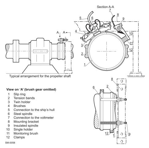
Figure 3-4 Typical shaft earthing arrangement
