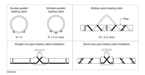
Figure 4-12 Trace heating cable arrangement
