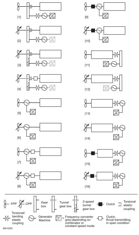
Figure 4-44 Arrangements for PTO, PTI, PTH
