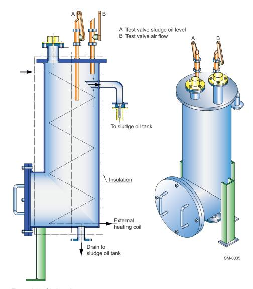
Figure 4-38 Sludge oil trap
