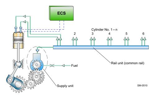
Figure 1-9 Flex system parts
