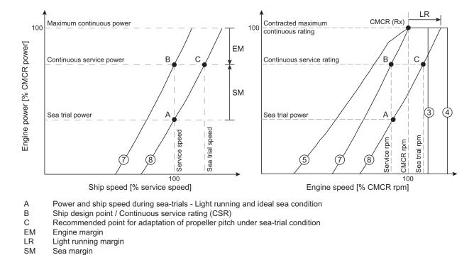
Line 3 Maximum engine speed limit for continuous operation
