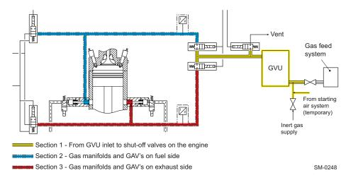
Figure 4-30 Gas leak test sequence (engines with GVU)
