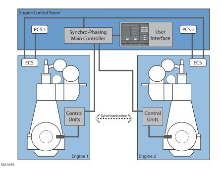
Figure 6-11 Synchro-Phasing system
