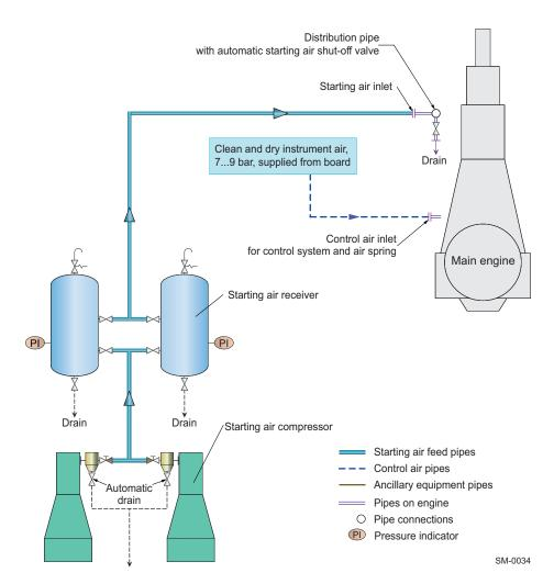
Figure 4-37 Starting and control air system
