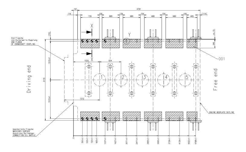
B-B ENGINE SIDE STOPPER ARRANGE WITH FLAME-CUT OR WELDED TYPE
