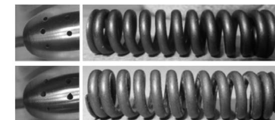
An injector tip and the spring in the injection control unit (ICU) block before and after the tests (above and below respectively). The orifice on the right of the picture of the injector tip shows clear signs of erosion, with some material broken off at the top.
