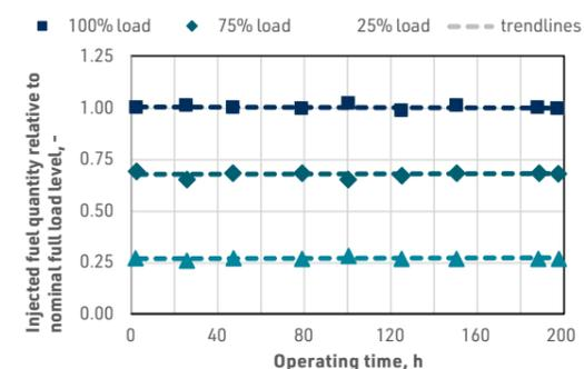
A biofuel was tested for roughly two million injection cycles each (about 200 hours) at three different loads. The injected quantity remained constant at all loads, indicating that application of the fuel is not associated with any injection system performance degradation that would require taking appropriate countermeasures.
