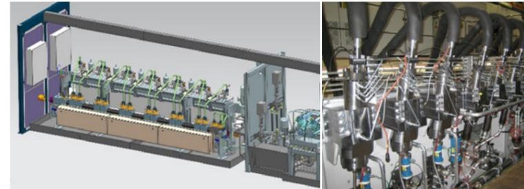
A test rig for examining the compatibility of liquid fuels with existing fuel systems.
