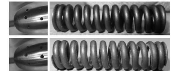
An injector tip and the spring in the injection control unit (ICU) block before and after the tests (above and below respectively). The orifice on the right of the picture of the injector tip shows clear signs of erosion, with some material broken off at the top.
