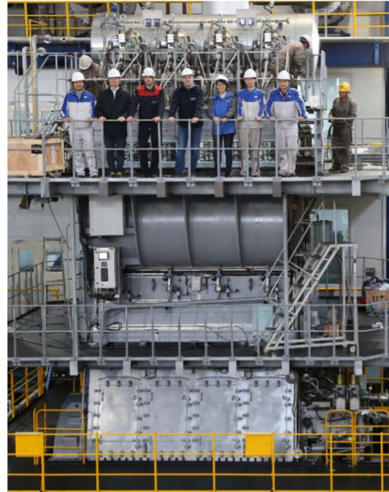
New lab engines – RTX-7 (DF engine, above), and RTX-8 being erected on the commissioning testbed (Diesel engine, below).
