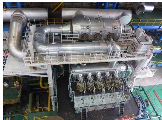
Figure 9: WinGD pilot SCR on CMD test bed
