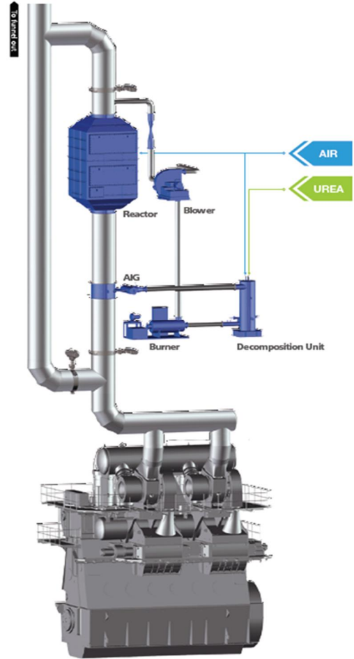
Figure 6: Tier III package; including main engine and LP-SCR system with burner arrangement. (picture courtesy of Doosan)
