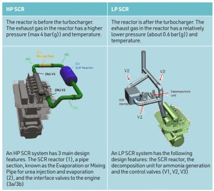
The HP SCR reactor is typically installed in the engine room. The ship designer has the choice to position the reactor in a horizontal or vertical position according to the engine room layout and available space.
