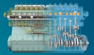
The most powerful marine internal combustion Otto cycle engine commercially available is the WinGD 12X92DF
