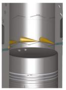
WinGD Piston Running Concept with Pulse Jet Cylinder Lubrication System
