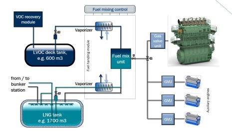
The VOC recovery system captures VOC emissions during loading and turns it into a valuable fuel
