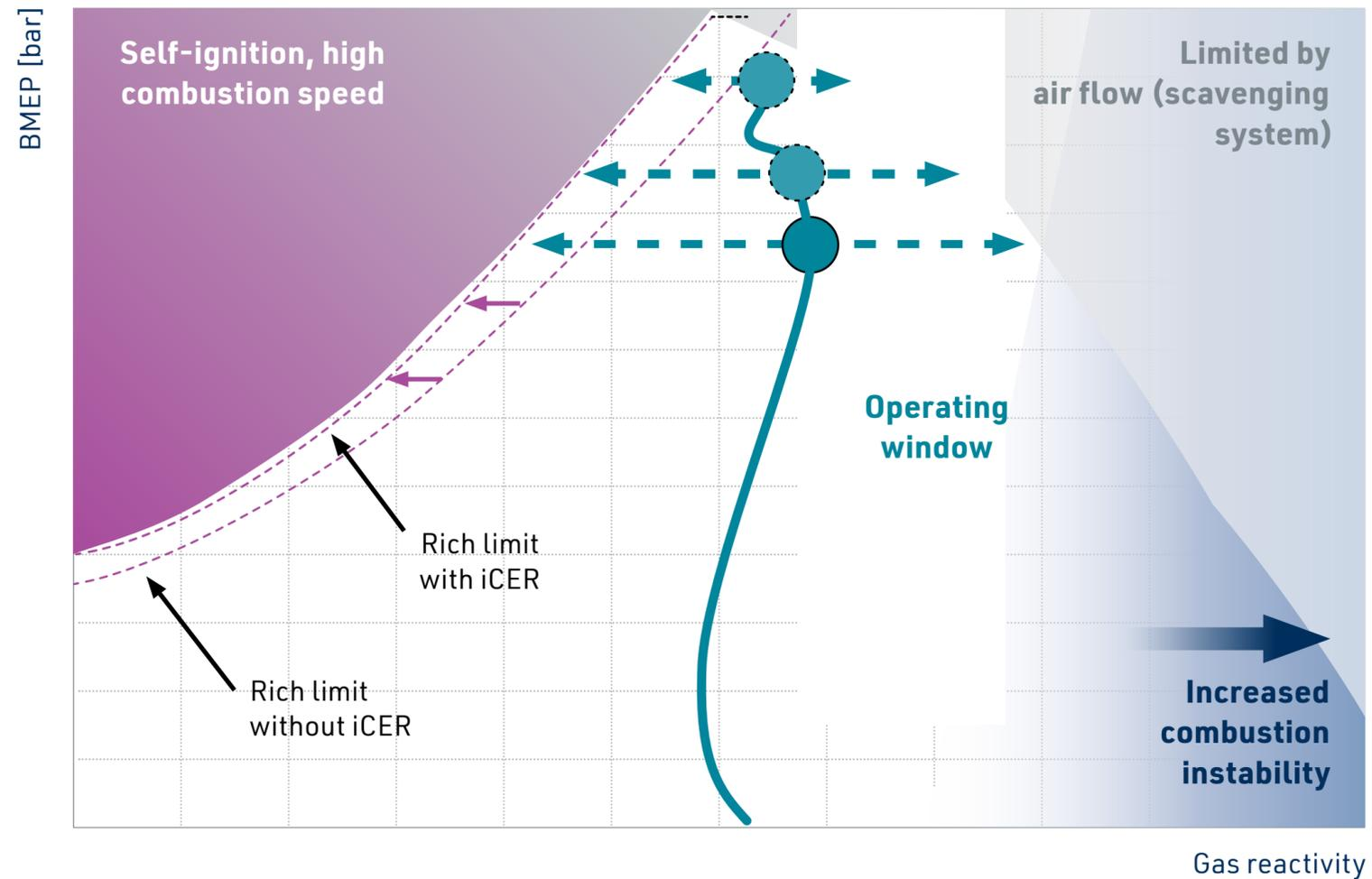
The iCER system extends the operating window of X-DF engines
