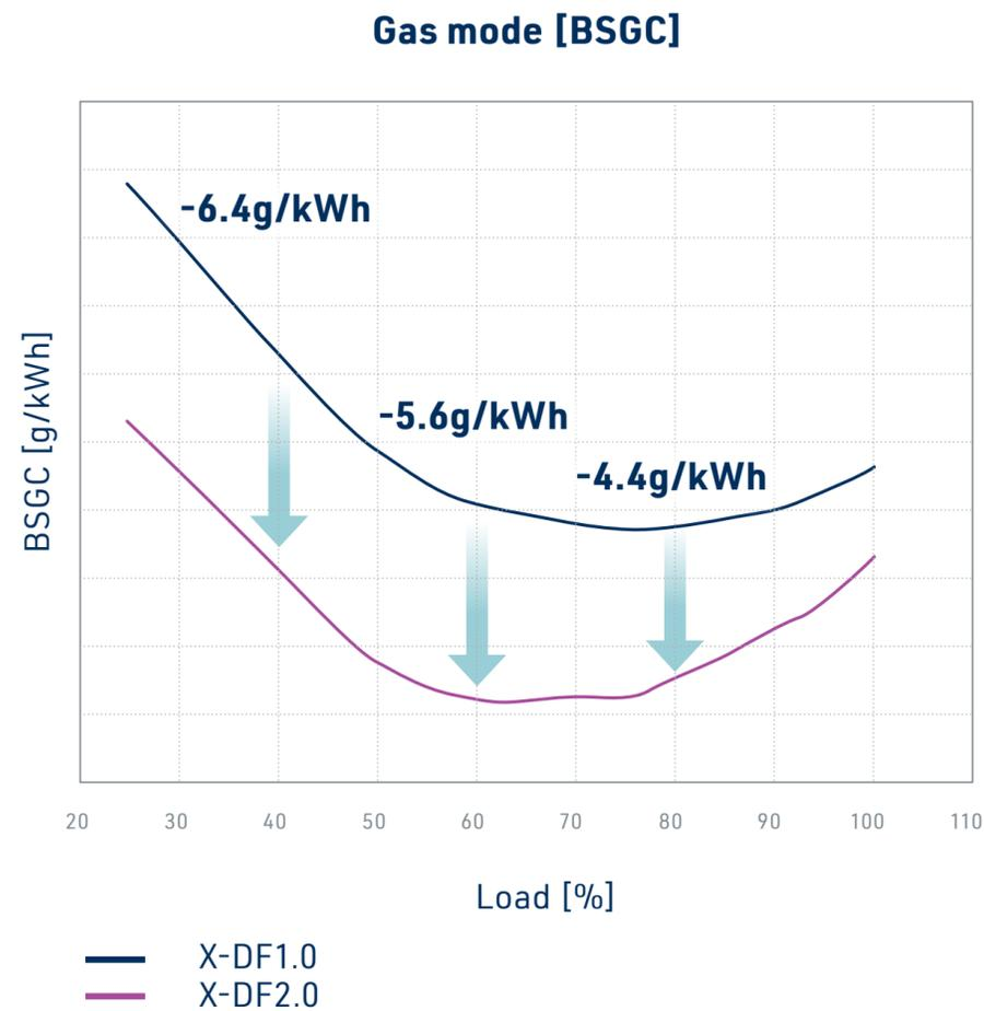
Fuel consumption improvement with increase of compression ratio for a typical 5X72DF engine
