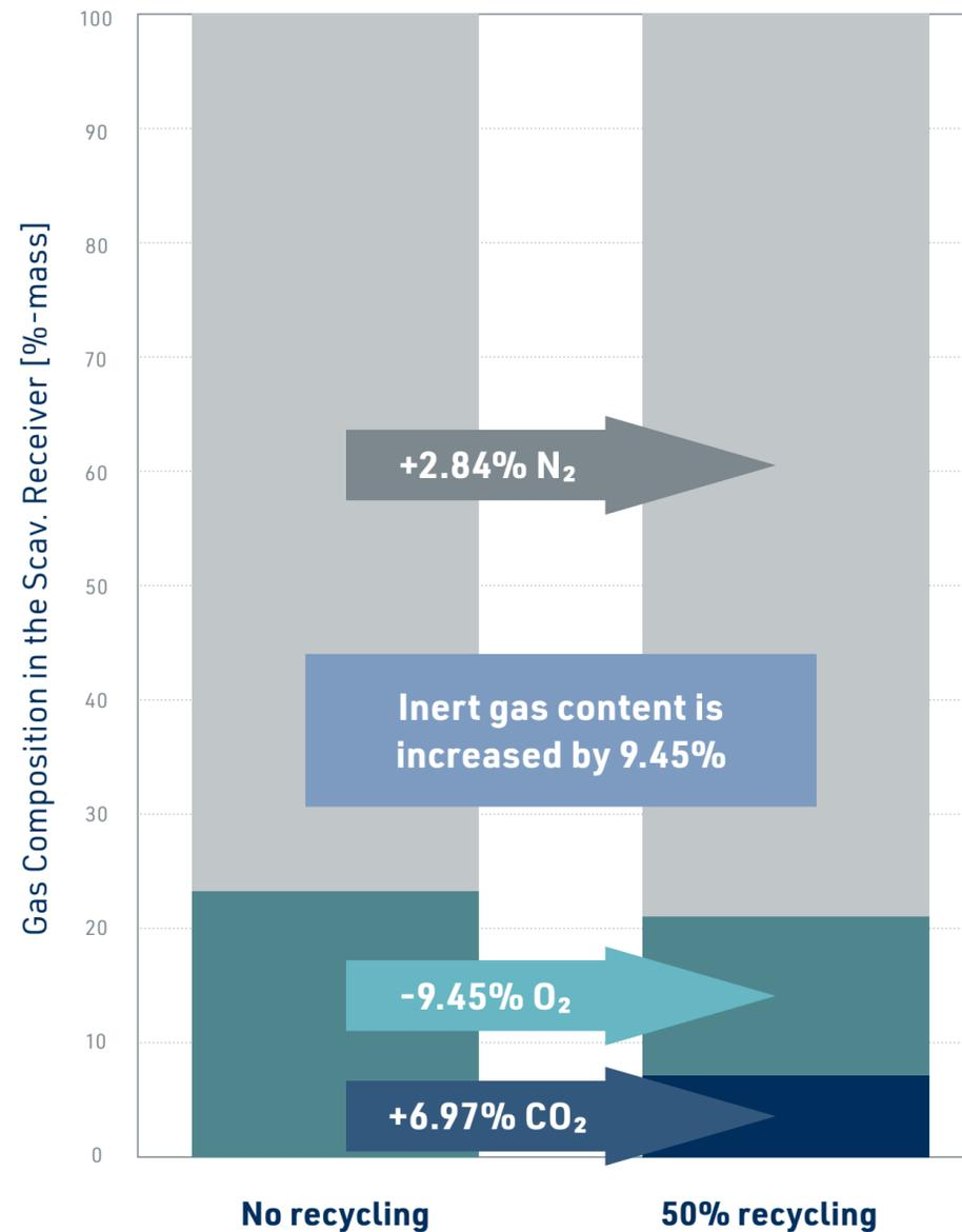
How the gas mixture changes with the introduction of exhaust gas recycling.
