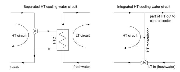
Figure 1: The two principal types of cooling water systems
