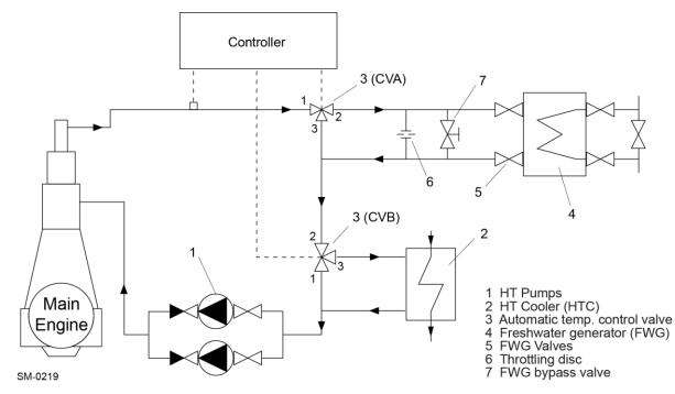
Figure 4: Optimised installation: FWG with installation alternative 'B'
