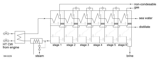
Figure 9: Principal flow diagram of a multi-stage flash evaporator
