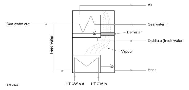
Figure 2: General flow diagram of a single-stage evaporator
