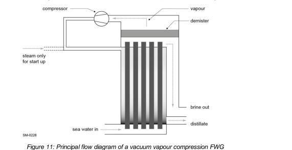
A mechanical compressor extracts the water vapour from the evaporation chamber,
