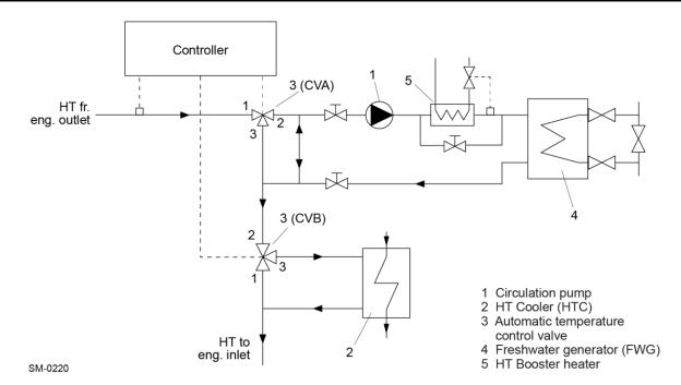
Figure 6: Booster heater integrated into the system of installation alternative 'B'
