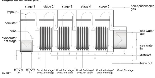
The Figure 8 shows the working principle of a multi-effect evaporation FWG with five stages as an example.
