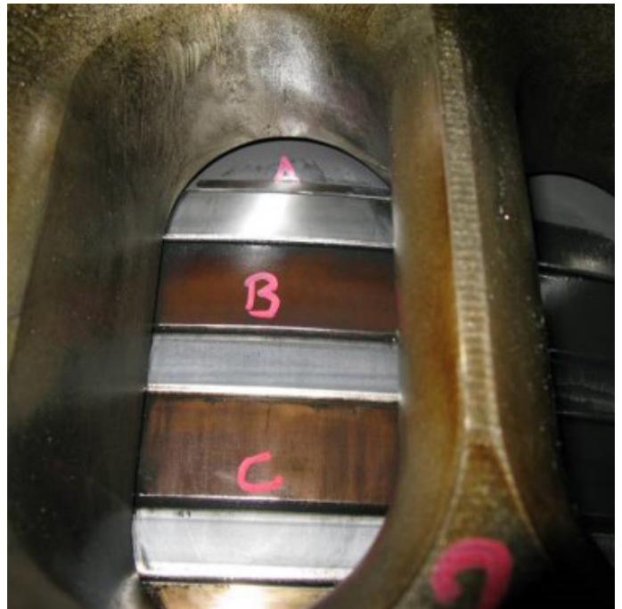
Clean the ring package and mark the piston rings
