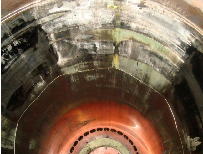
Picture 1: Cylinder liner surface with signs of extreme corrosive attack
