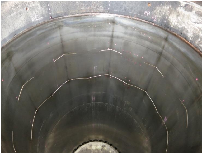
Picture 2: Cylinder liner surface with regular running surface appearance
