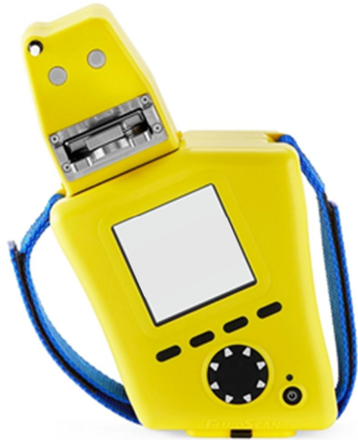
Picture 9: Infrared-spectrometer for BN measurement
