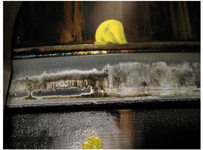
Picture 3: Piston ring running surface with signs of extreme corrosive attack
