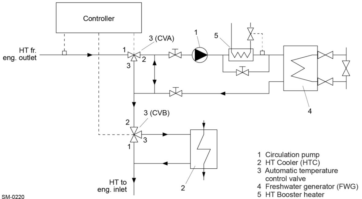
Figure 6: Booster heater integrated into the system of installation alternative 'B'
