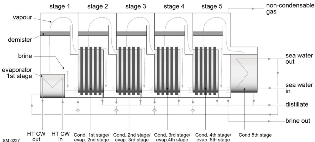
Figure 8: Principal flow diagram of a multi-stage FWG
