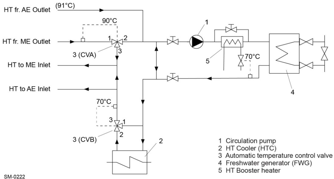
Figure 7: Booster heater integrated into the system of installation utilising ME and AE CCW heat dissipation
