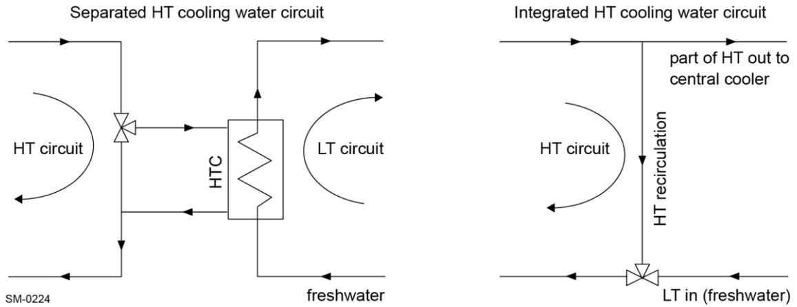
Figure 1: The two principal types of cooling water systems
