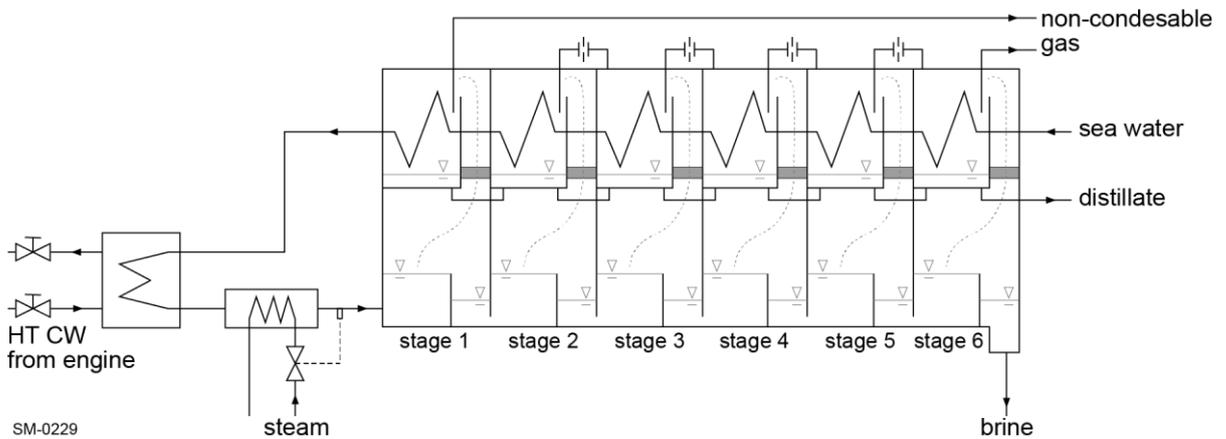
Figure 9: Principal flow diagram of a multi-stage flash evaporator
