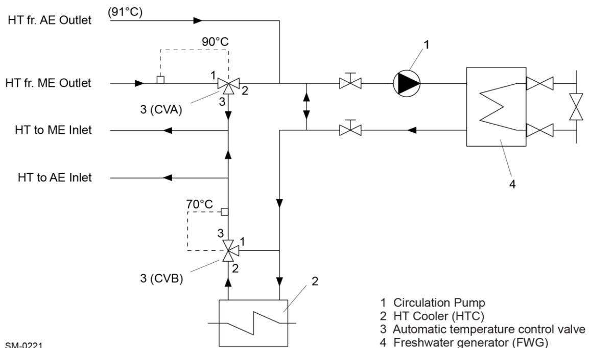
Figure 5: Installation option utilising ME and AE CCW heat dissipation
