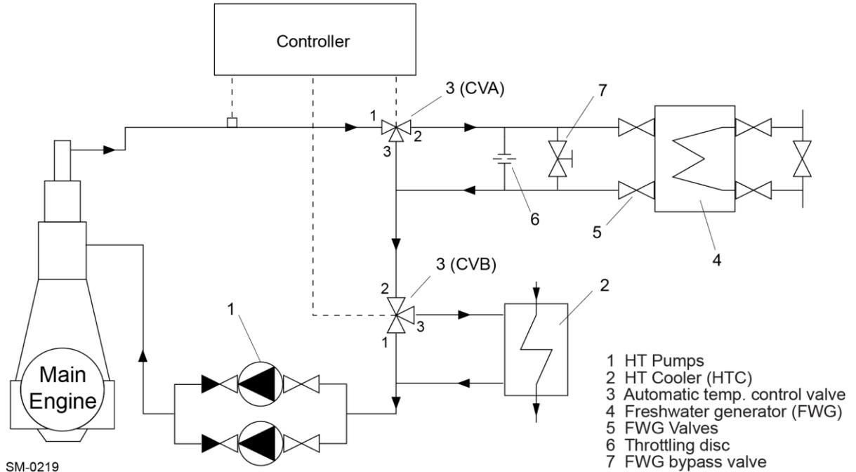
Figure 4: Optimised installation: FWG with installation alternative 'B'
