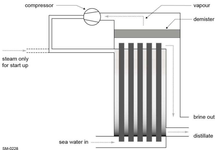
Figure 11: Principal flow diagram of a vacuum vapour compression FWG
