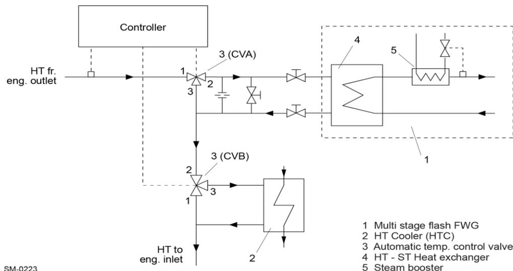
Figure 10: Multi-stage flash evaporator system integration
