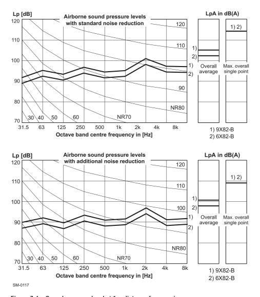
Figure 7-4 Sound pressure level at 1m distance from engine
