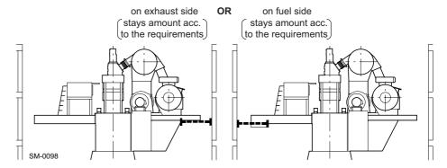
Figure 6-4 General arrangement of hydraulic stays for one-side installation
