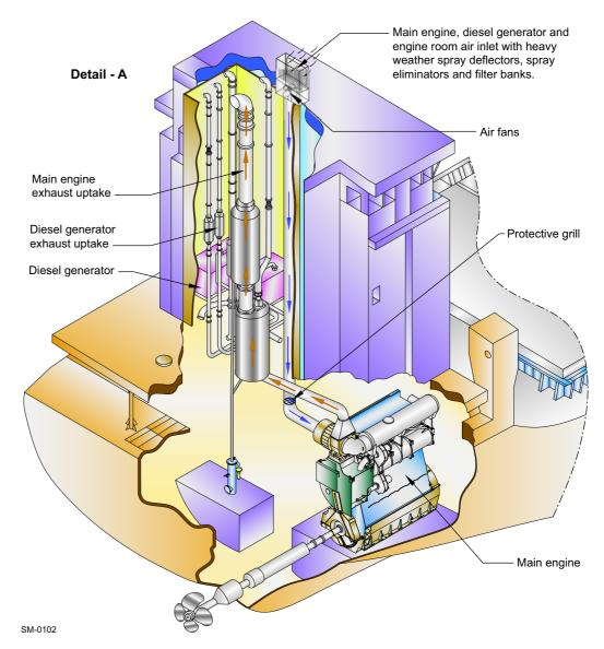
Figure 4-19 Direct suction of combustion air (detail)
