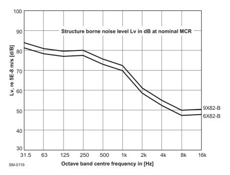
Figure 7-7 Structure-borne noise level at engine feet vertical
