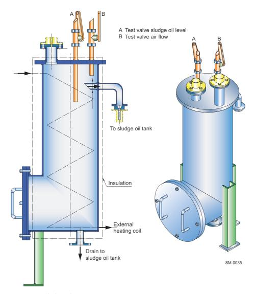
Figure 4-15 Sludge oil trap
