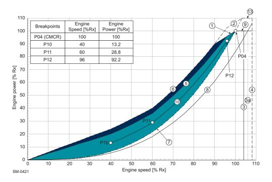
Figure 2-4 Power range limits for PTO operation
