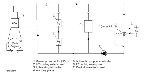
Figure 4-3 Scheme of cooling water system
