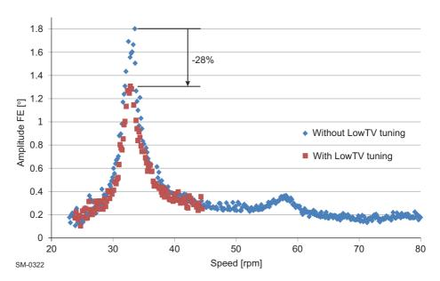
Figure 1-8 Vibration amplitudes - Achievements with default LowTV tuning
