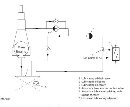
Figure 4-6 Scheme of lubricating oil system
