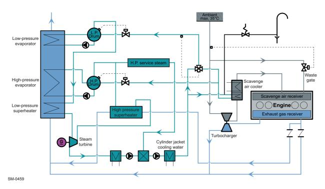
Figure 4-32 Dual-pressure system with LP superheater & separate HP superheater
