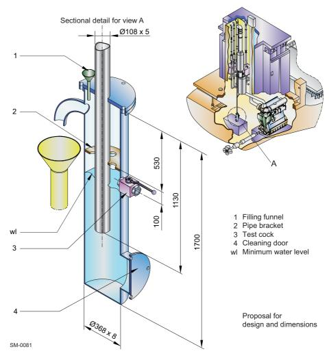
Figure 4-16 Arrangement of automatic water drain
