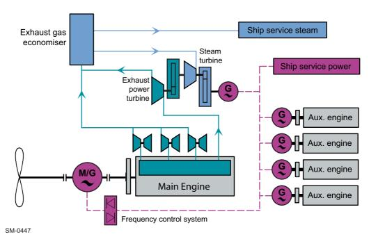
Figure 4-28 Heat recovery with power and steam turbines and PTI/PTO
