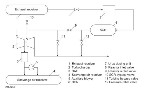
Figure 7-3 High-pressure SCR — arrangement
