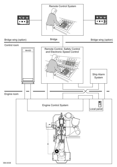
Figure 5-3 Remote Control System layout
