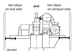
Figure 6-5 General arrangement of hydraulic stays for both-side installation
