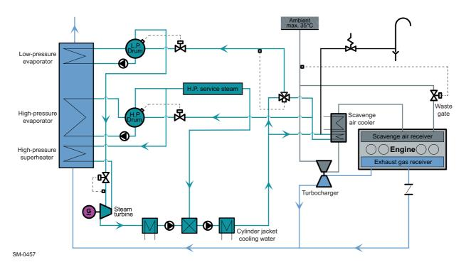
Figure 4-30 Dual-pressure steam system with HP superheater
