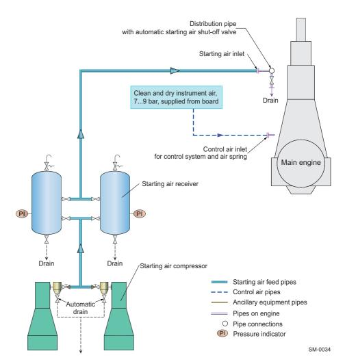
Figure 4-14 Starting and control air system
