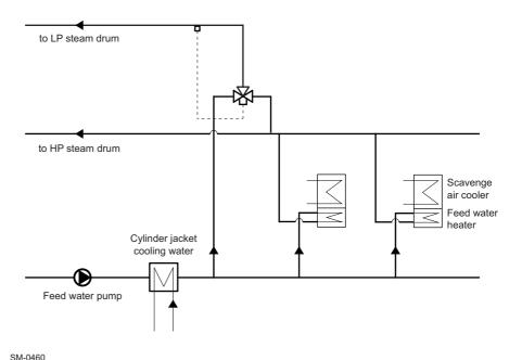
Figure 4-25 Feed water heating
