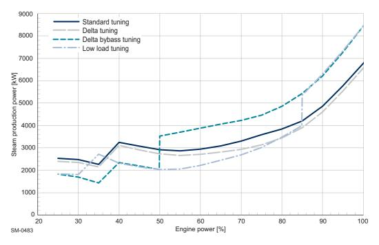
Figure 1-4 Steam production power diagram
