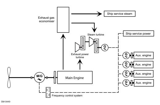
Figure 4-23 Heat recovery — typical system layout
