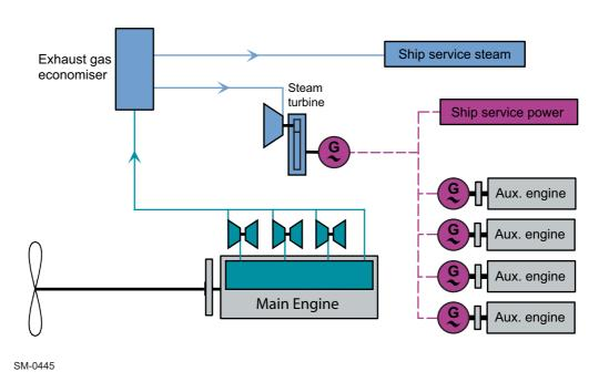
Figure 4-26 Heat recovery with steam turbine
