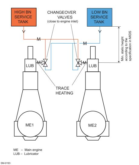
Figure 4-2 Cylinder LO system layout for twin-engine installation
