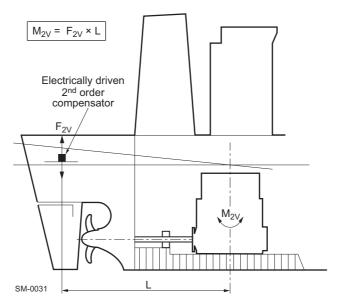
Figure 6-2 Locating an electrically driven compensator
