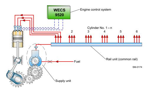
Figure 1-10 Flex system parts
