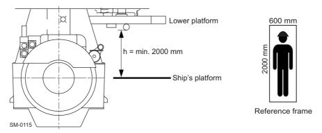
Figure 3-3 Minimum requirements for headroom
