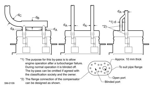
Figure 4-17 Determination of exhaust pipe diameter
