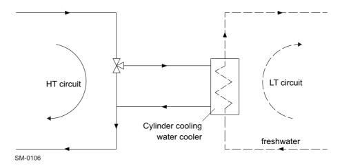
Figure 4-4 Separate HT cooling water circuit
