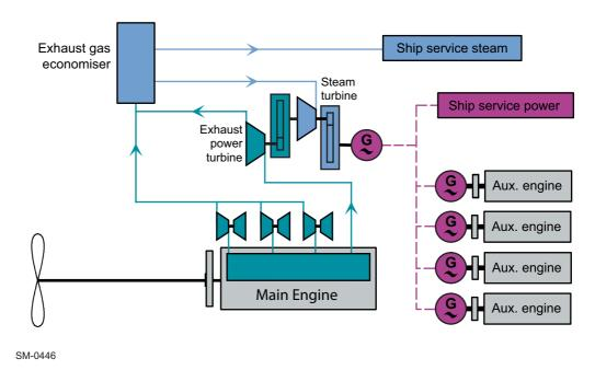
Figure 4-27 Heat recovery with power and steam turbines
