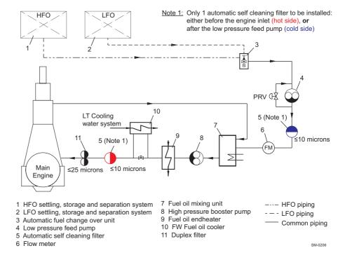
Figure 4-11 Fuel oil filter arrangement 'A'
