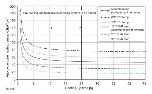
Figure 4-5 Pre-heating power requirement per cylinder
