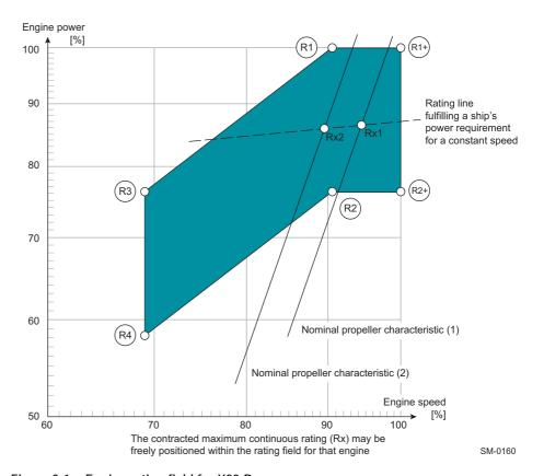
Figure 2-1 Engine rating field for X82-B
