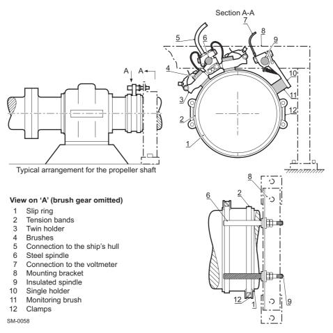
Figure 3-4 Shaft earthing arrangement
