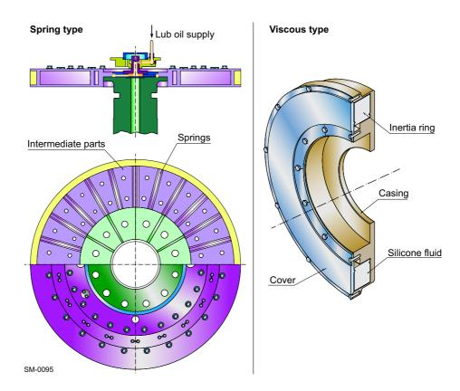
Figure 6-6 Vibration dampers (spring type and viscous type)
