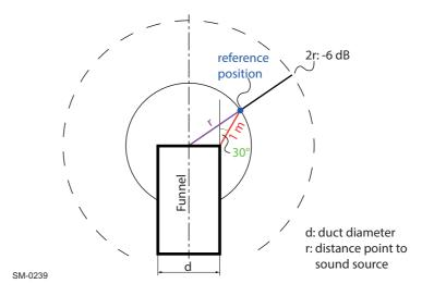
Figure 7-5 Exhaust noise reference point
