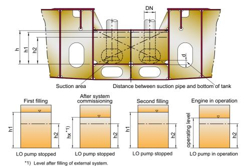
Volume and level in the lub. oil drain tank depend on capacity of pipes, coolers, filters, etc.
