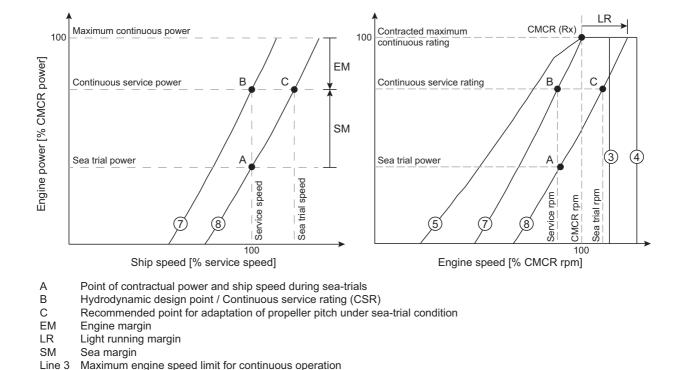
Figure 2-2 Propeller curves and operational points
