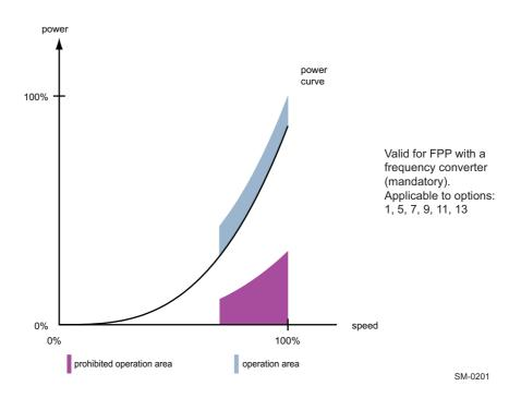
Figure 4-22 FPP with mandatory frequency converter
