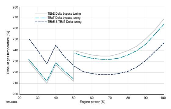
Figure 1-6 Exhaust gas temperature increase with DBT
