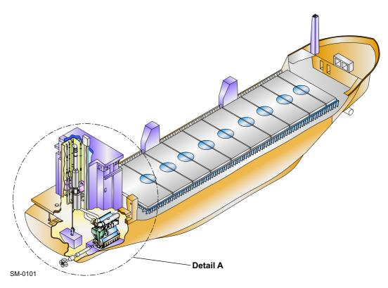
Figure 4-18 Direct suction of combustion air — main and auxiliary engine
