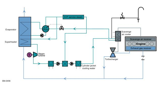
Figure 4-29 Single-pressure steam system with evaporator and superheater
