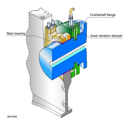
Figure 6-7 Example of axial vibration damper
