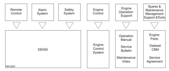
Figure 5-2 Engine management and automation concept
