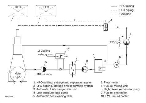
Figure 4-12 Fuel oil filter arrangement 'B'
