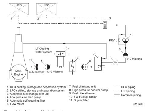
Figure 4-9 Scheme of fuel oil system
