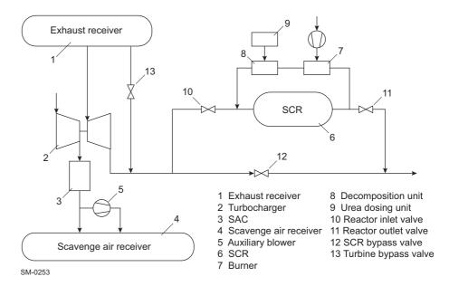
Figure 7-2 Low-pressure SCR — arrangement
