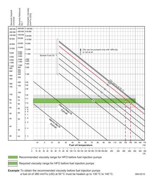
Figure 4-13 Fuel oil viscosity-temperature diagram
