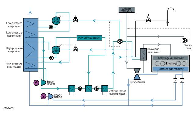
Figure 4-31 Dual-pressure steam system with HP and LP superheaters
