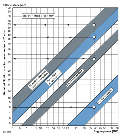
Figure 4-20 Air filter size (example for 8-cyl. engine)
