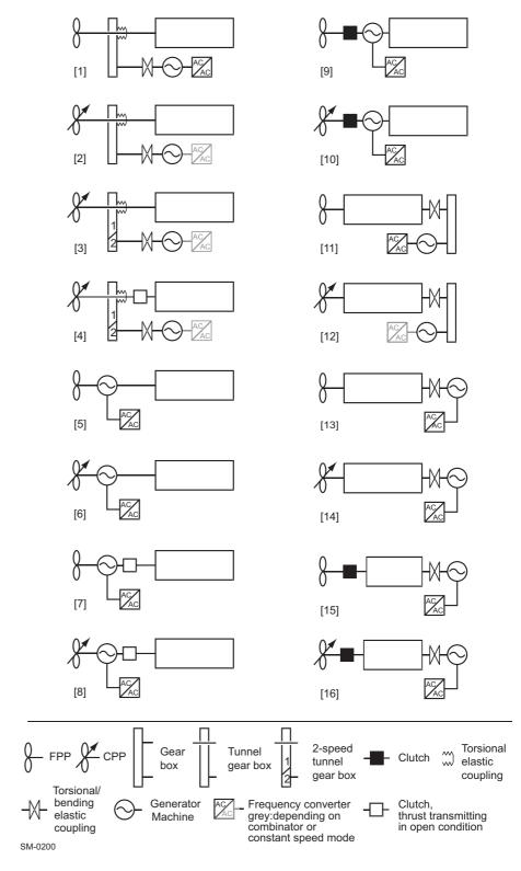
Figure 4-21 Arrangements for PTO, PTI, PTH
