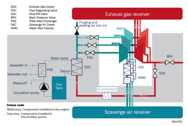
Figure 2-34: The iCER system (off-engine option) with three turbochargers and the exhaust gas return pipe return pipe routed to the turbocharger connection from below
