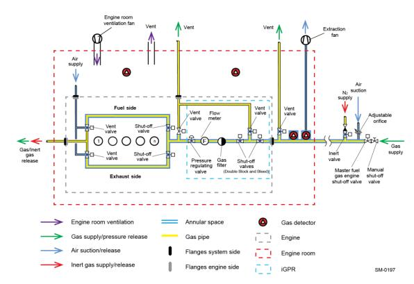
Figure 2-13: Typical sketch of the iGPR layout
