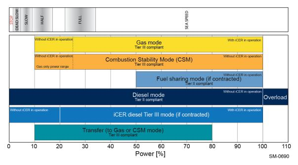
Figure 2-28: Operating modes of X-DF2.0 engines Tier III
