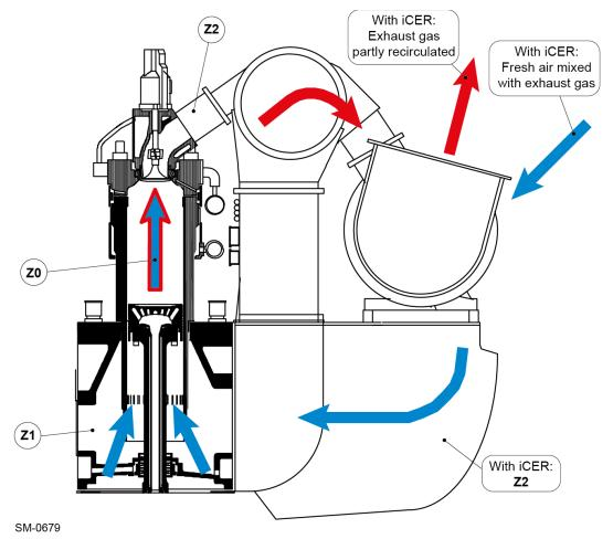
Figure 3-2: Cylinder unit and piston underside (hazard zones)
