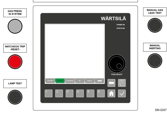
Figure 2-9: The GVU Human Machine Interface (HMI)
