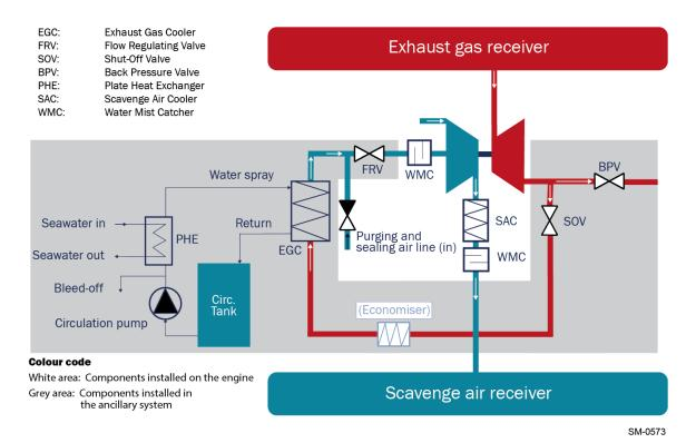
Figure 2-32: The iCER system (off-engine option) with one turbocharger and the exhaust gas return pipe routed to the turbocharger connection from above
