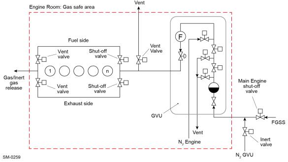
Figure 2-12: The GVU process component diagram
