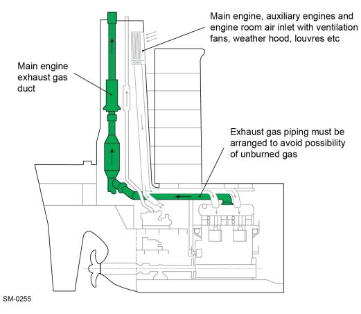
Figure 2-16: External exhaust gas system
