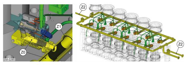
Figure 3-3: Fuel gas system (hazard zones)
