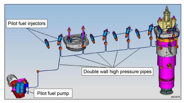
Figure 2-15: Pilot fuel high-pressure system
