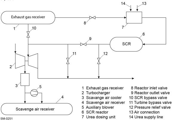
Figure 2-22: High-pressure SCR
