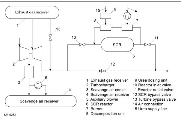
Figure 2-20: LP SCR with indirect urea injection (temperature controlled)
