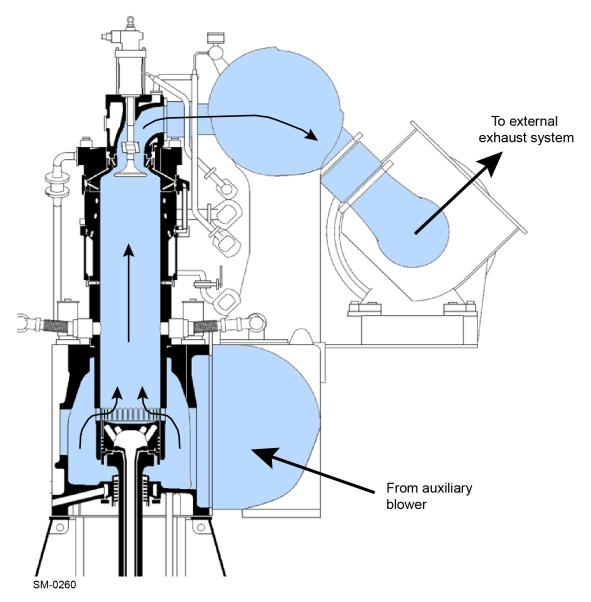
Figure 2-17: Exhaust gas ventilation
