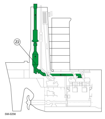
Figure 3-4: External exhaust gas system (hazard zone)
