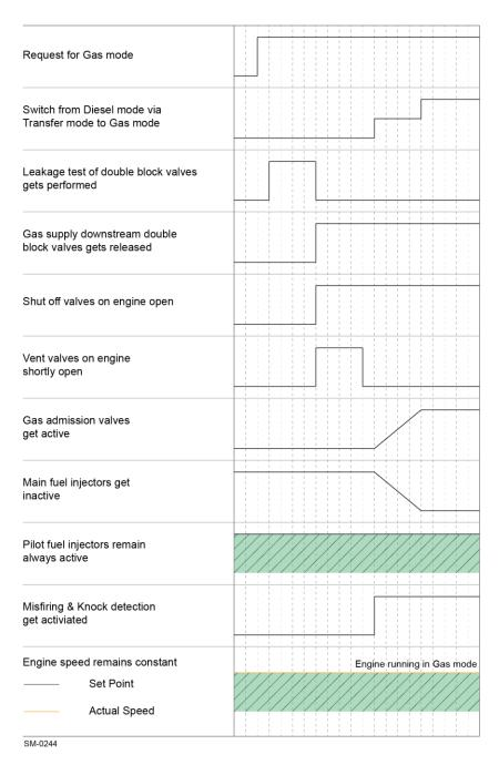
Figure 2-39: Gas mode event sequence – Transfer from diesel to gas mode
