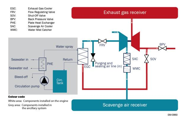
Figure 2-35: The iCER on-engine system with one turbocharger
