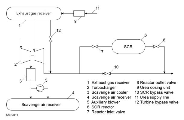
Figure 2-19: LP SCR with direct urea injection
