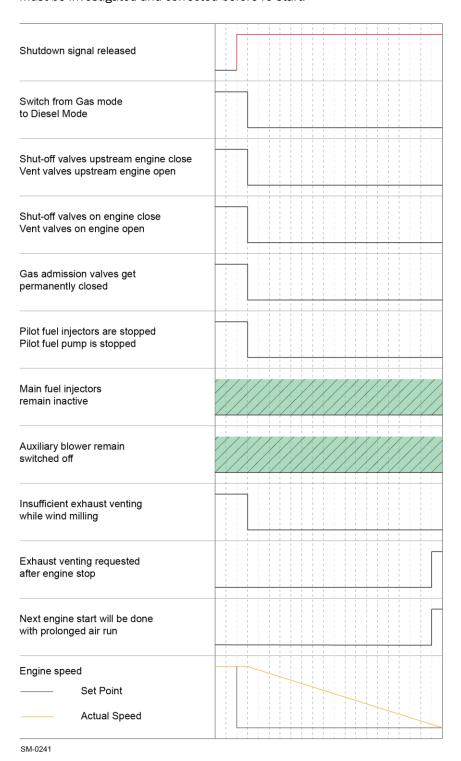
Figure 2-38: Gas mode event sequence – Non-cancellable shutdown and emergency stop
