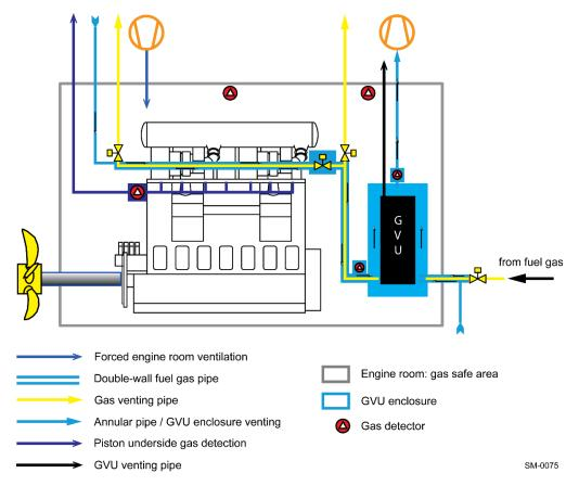
Figure 3-1: Example of gas detector positioning in the engine room, the gas supply system and the engine with GVU
