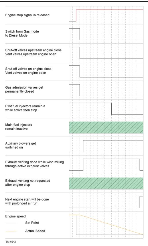
Figure 2-36: Gas mode event sequence – Engine stop
