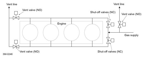
Figure 2-7: Piping design of fuel gas supply pipe to engine
