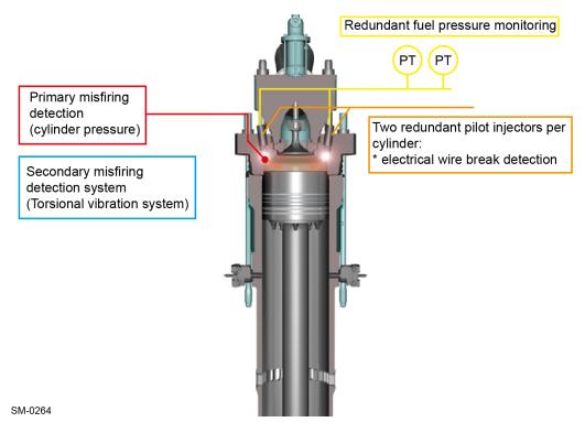
Figure 5-1: Misfiring monitoring concept
