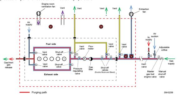
Figure 2-14: Purging from the inert valve on the ship side
