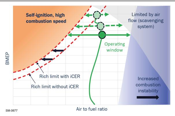
Figure 2-4: The X-DF operating window with iCER
