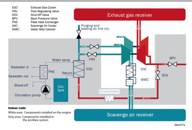
Figure 2-33: The iCER system (off-engine option) with two turbocharger and the exhaust gas return pipe routed to the turbocharger connection from below
