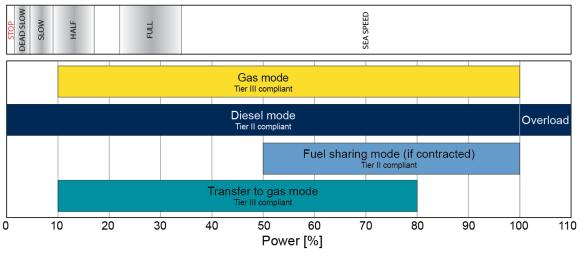
Figure 2-27: Operating modes of X-DF engines without iCER
