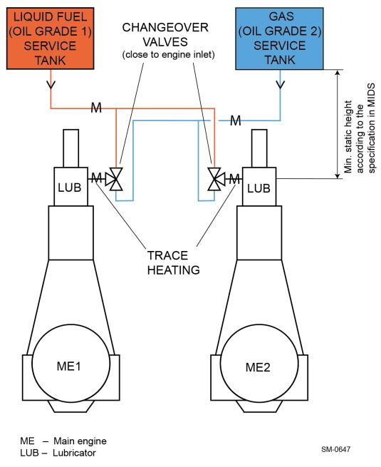
Figure 4-2: Cylinder LO system layout with iCAT for twin-engine installation
