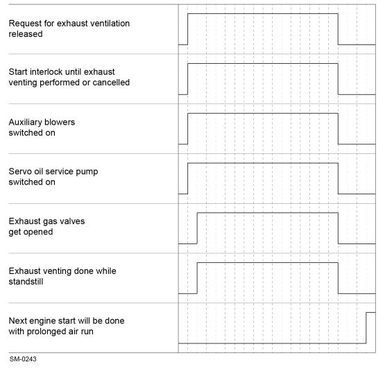
Figure 2-18: Exhaust gas ventilation procedure event sequence
