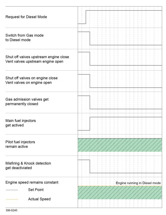
Figure 2-40: Gas mode event sequence – Transfer from gas to diesel mode
