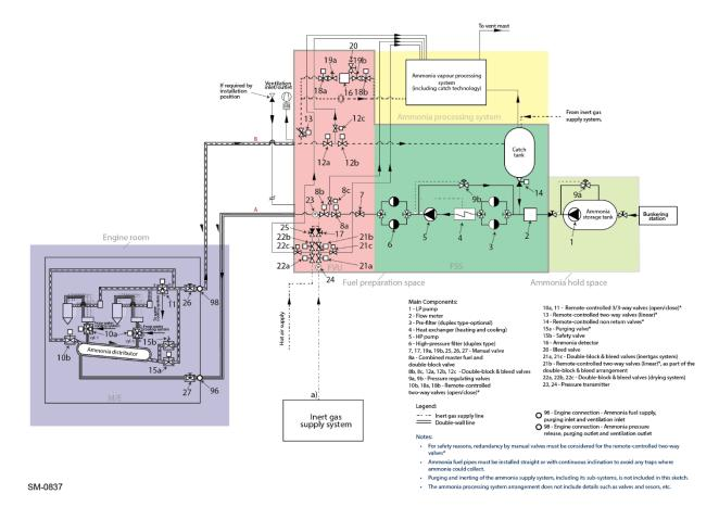
Figure 3-1: Proposal for the ammonia fuel system arrangement of an ammonia storage and supply system arrangement
