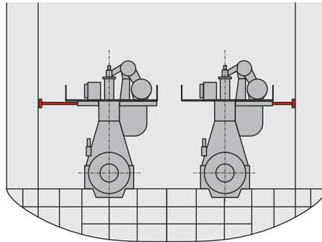
Installation of lateral stays on the fuel and exhaust side with:
