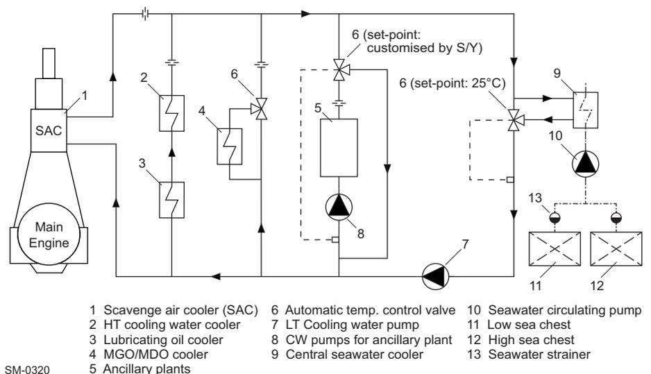
**Figure 4-4** LT cooling water circuit — Dual set-point temperatures
