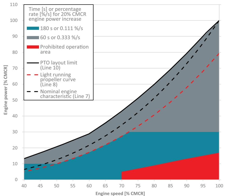
Figure 4-58 Maximum power increase rate for PTO application in gas mode
