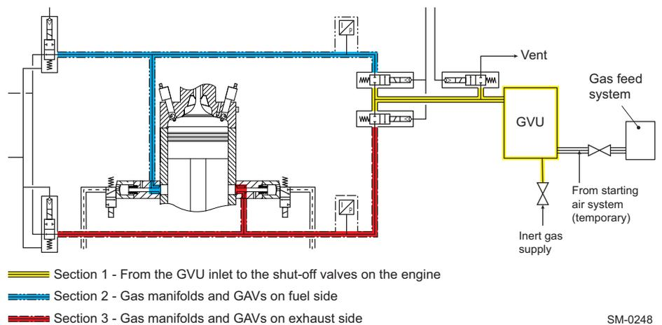
**Figure 4-34 Gas leak test sequence (engines with GVU)**
