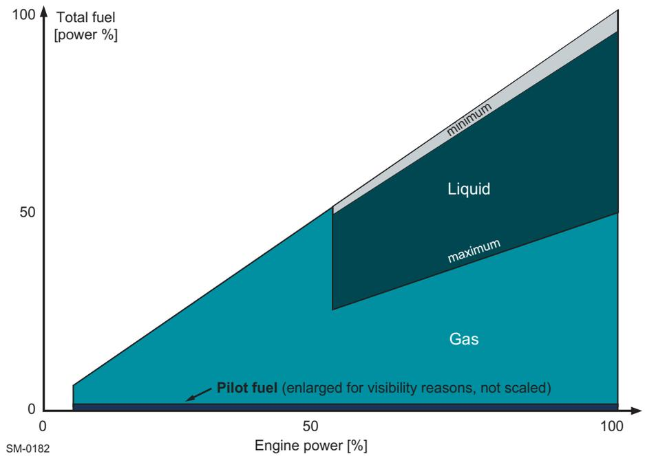
Figure 1-6 Fuel sharing mode — energy amount of different ratios of fuel
