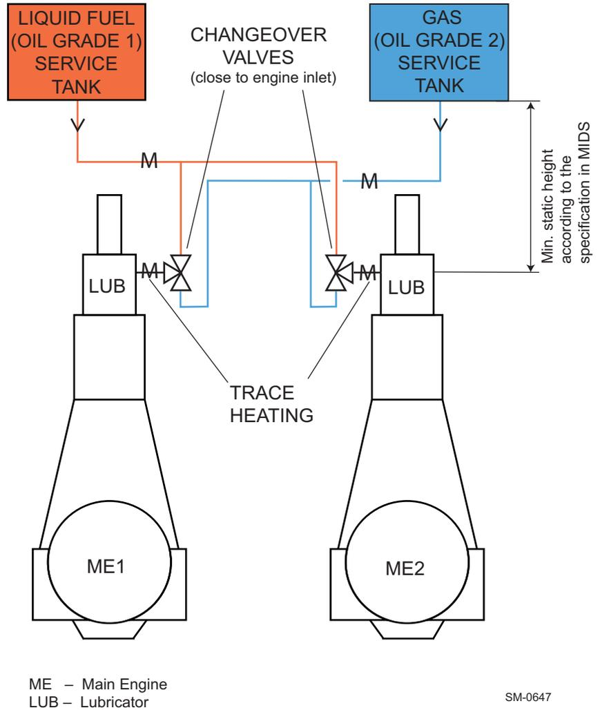
**Figure 4-9** Dual cylinder lubricating oil installation, enabling independent gas and liquid fuel (maximum 0.50% m/m sulphur) operation with a manual changeover valve
