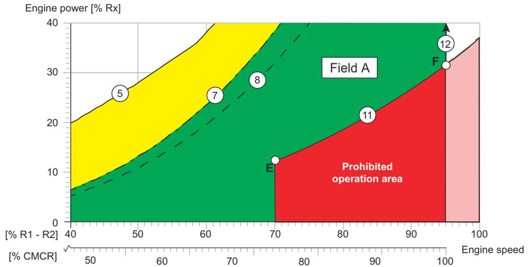
**Figure 2-8 Calculating the prohibited operation area for the CMCR speed**
