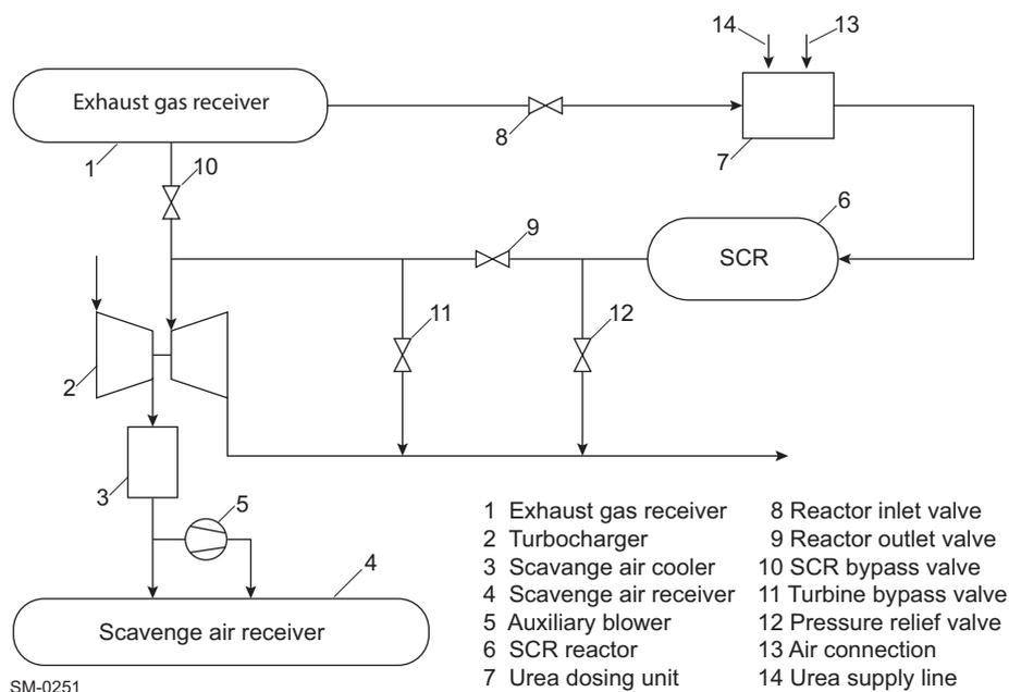
**Figure 7-3 High-pressure SCR**
