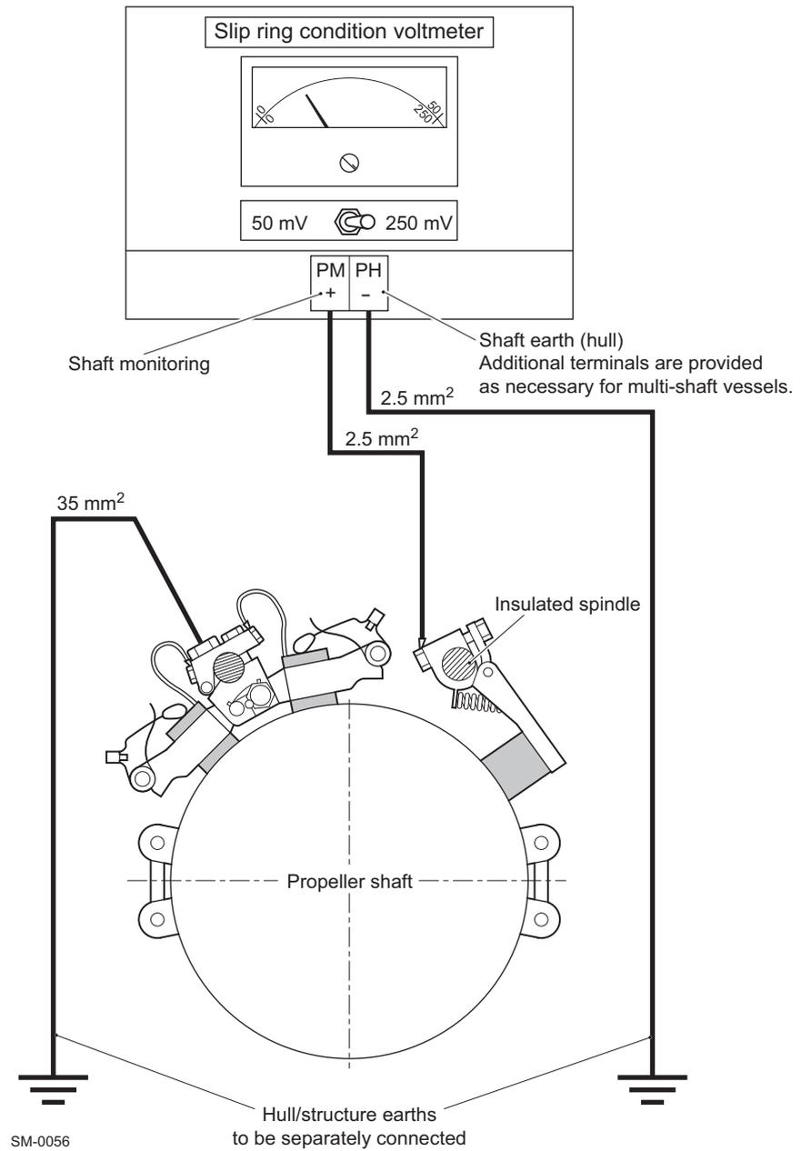
Figure 3-11 Typical shaft earthing with condition monitoring facility
