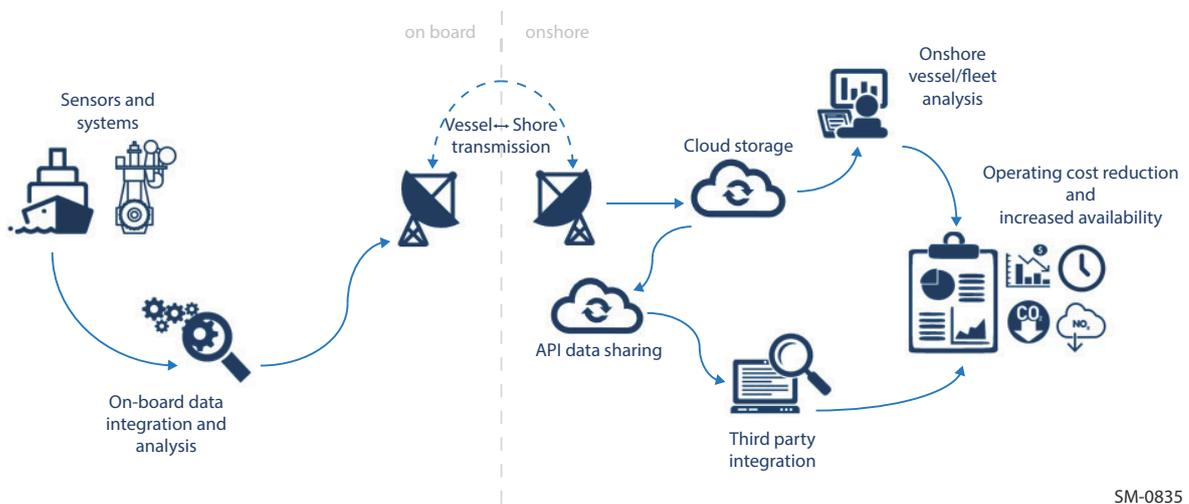
Figure 5-8 The WiDE data collection and analysis process
