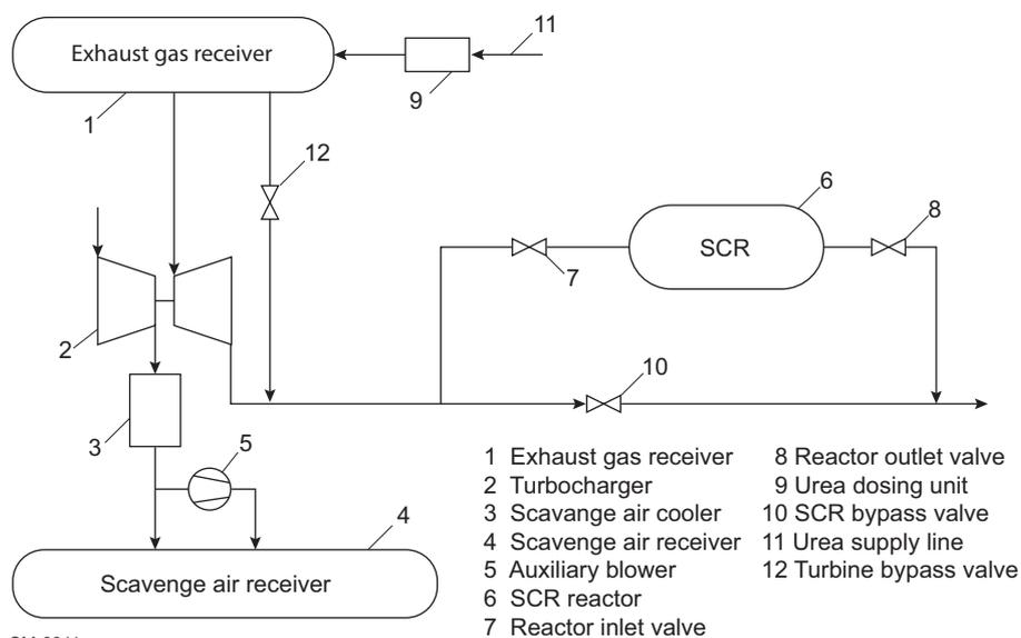
**Figure 7-4 Low-pressure SCR with direct urea injection**
