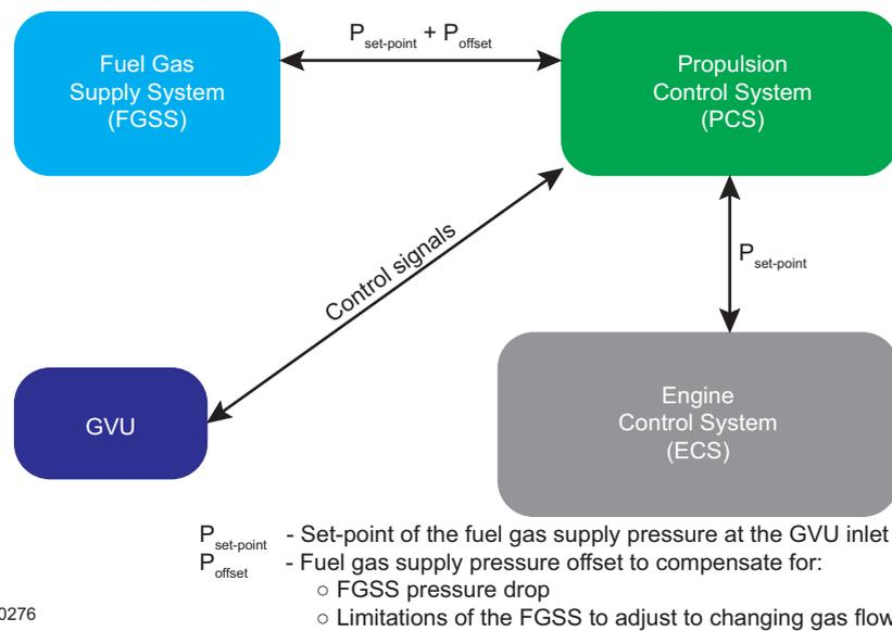
Figure 4-28 Fuel gas supply pressure control at the GUV inlet (engines with GUV)
