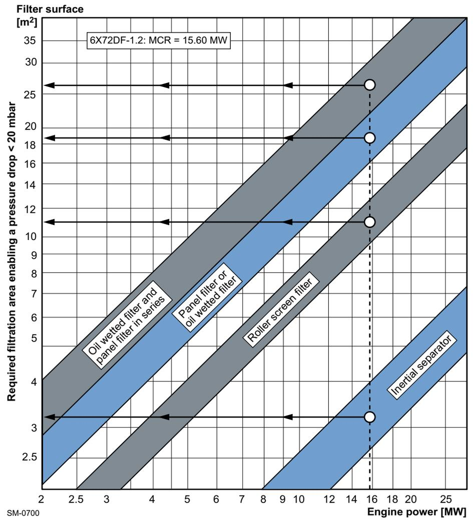
Figure 4-52 Air filter size (example for 6-cyl. engine)
