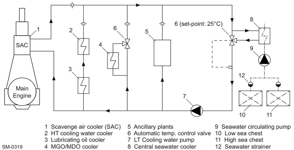
**Figure 4-3** LT cooling water circuit — Single set-point temperature
