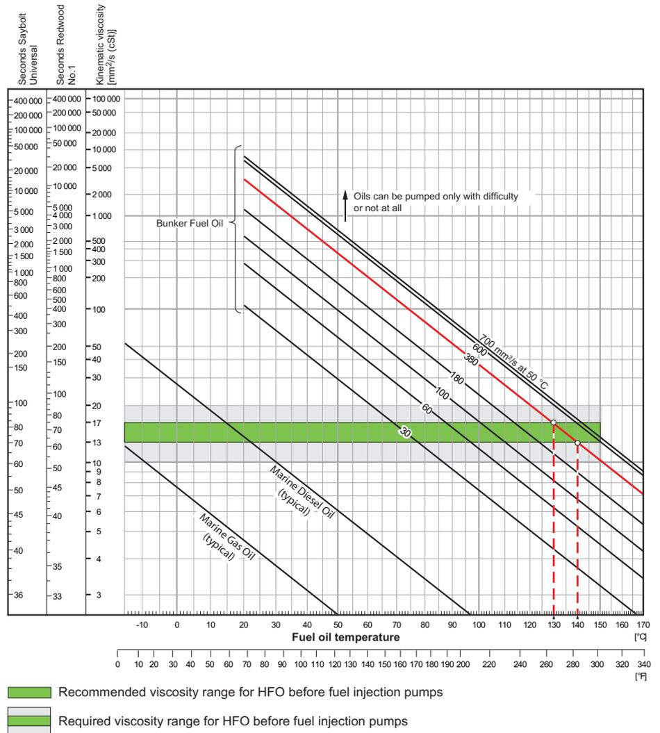
**Example** To obtain the recommended viscosity before fuel injection pumps a fuel oil of 380 mm<sup>2</sup>/s (cSt) at 50 °C must be heated up to 130 °C to 140 °C.
