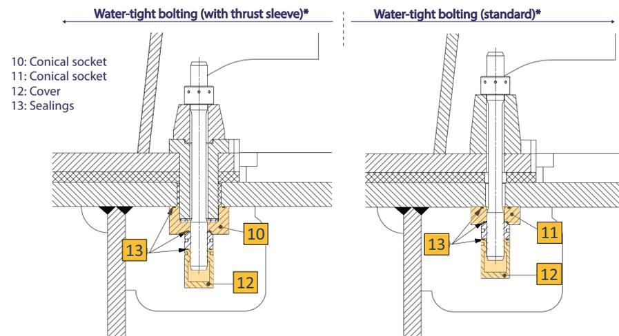
(\*Assembly parts for water-tight bolts)
