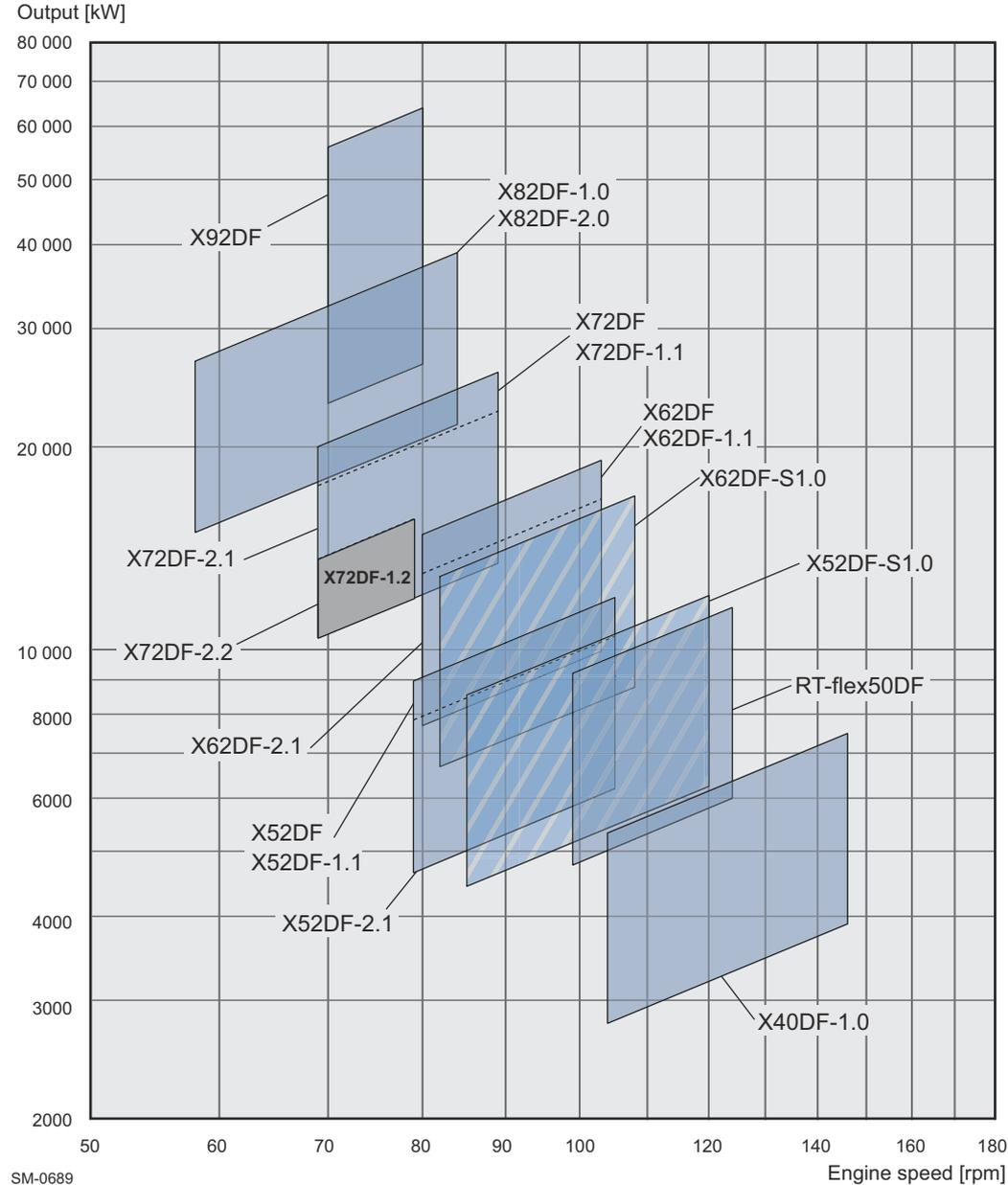
**Figure 1-1 Power/speed range of the WinGD X-DF engines**
