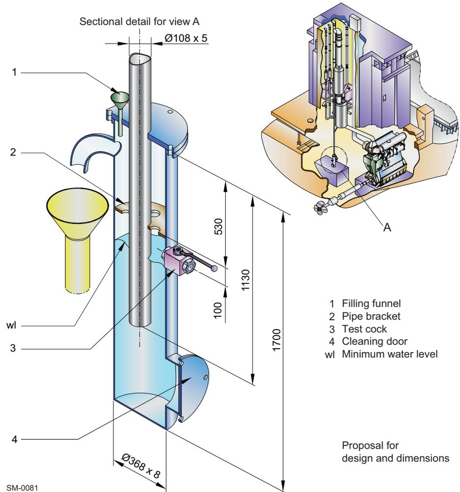
Figure 4-48 Arrangement of automatic water drain
