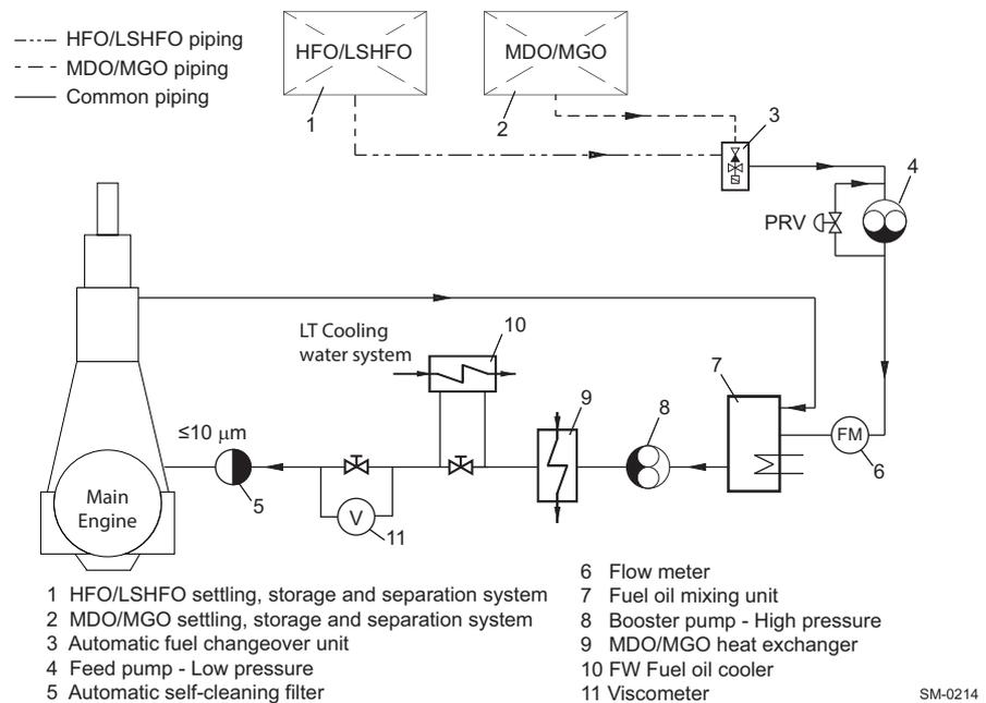
**Figure 4-41 Fuel oil filter arrangement ‘B’**
