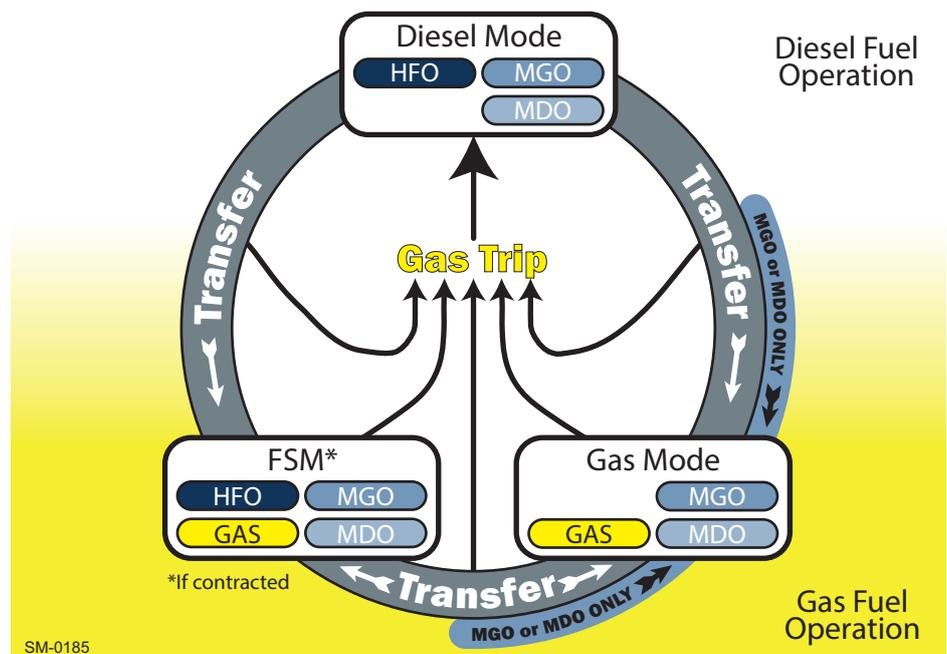
Figure 1-7 Fuel transfers and gas trips
