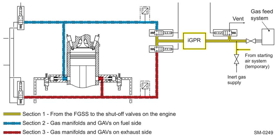
**Figure 4-33 Gas leak test sequence (engines with iGPR)**
