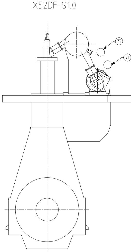
71 OUTLET - Exhaust gas turbocharger
