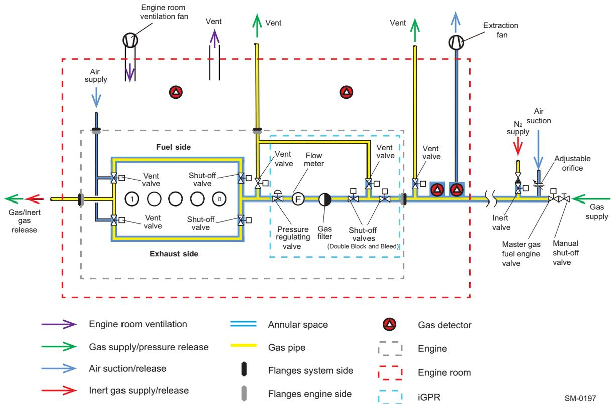
Figure 4-52 Fuel gas supply system with the iGPR
