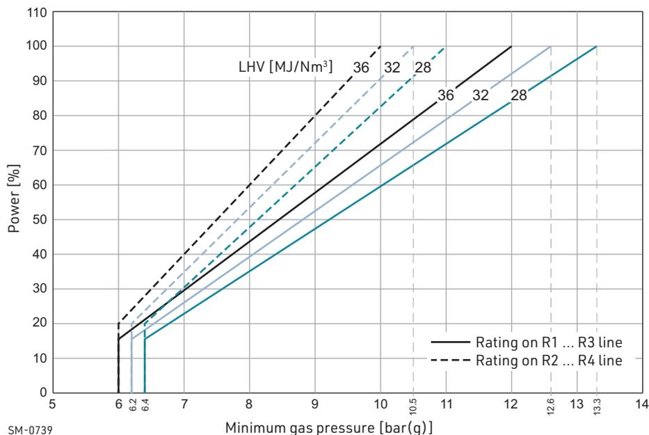
**Figure 4-48 Design fuel gas supply pressure requirements**
