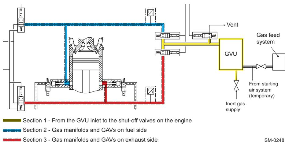
**Figure 4-56 Gas leak test sequence (engines with GVU)**
