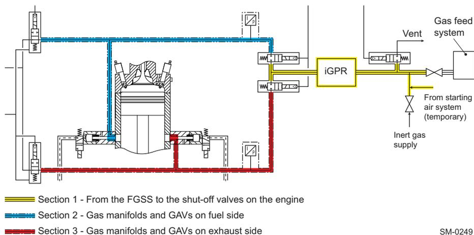
**Figure 4-55 Gas leak test sequence (engines with iGPR)**
