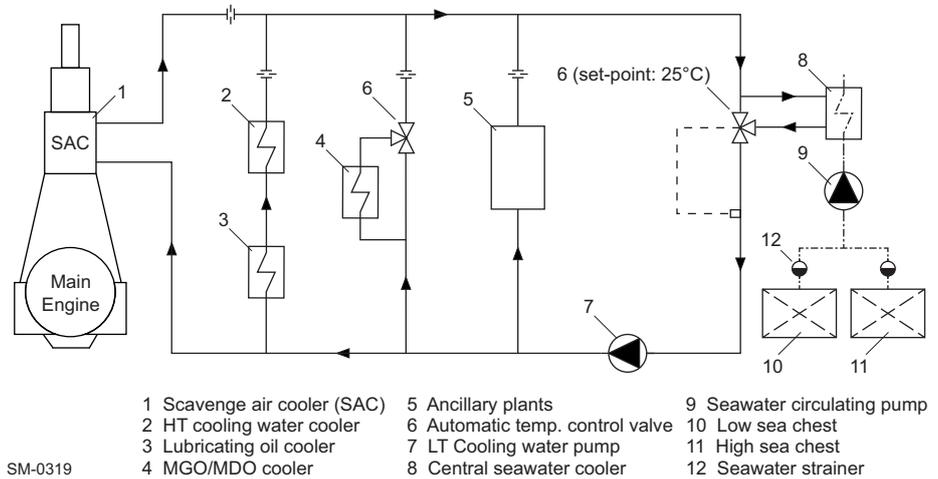
**Figure 4-25** LT cooling water circuit — Single set-point temperature
