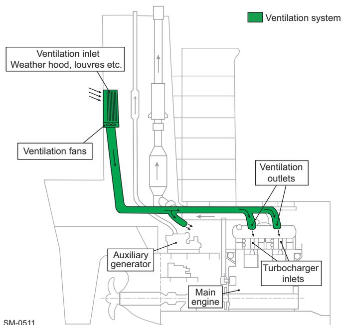
**Figure 4-73 Ventilation system arrangement 1 — Engine room ventilation system**
