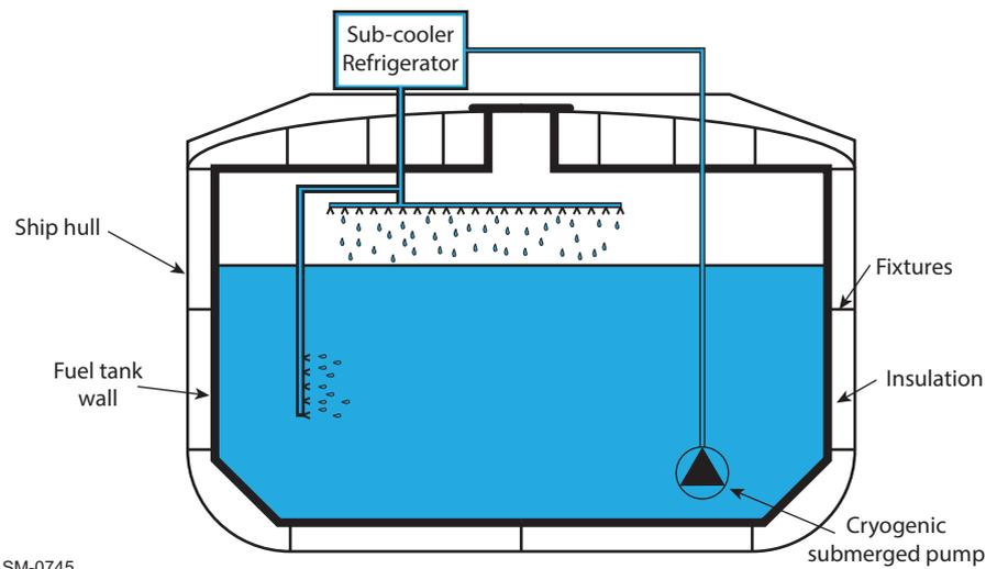
**Figure 4-47 An LNG sub-cooler within an integrated tank**
