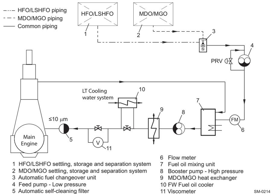
**Figure 4-63 Fuel oil filter arrangement ‘B’**
