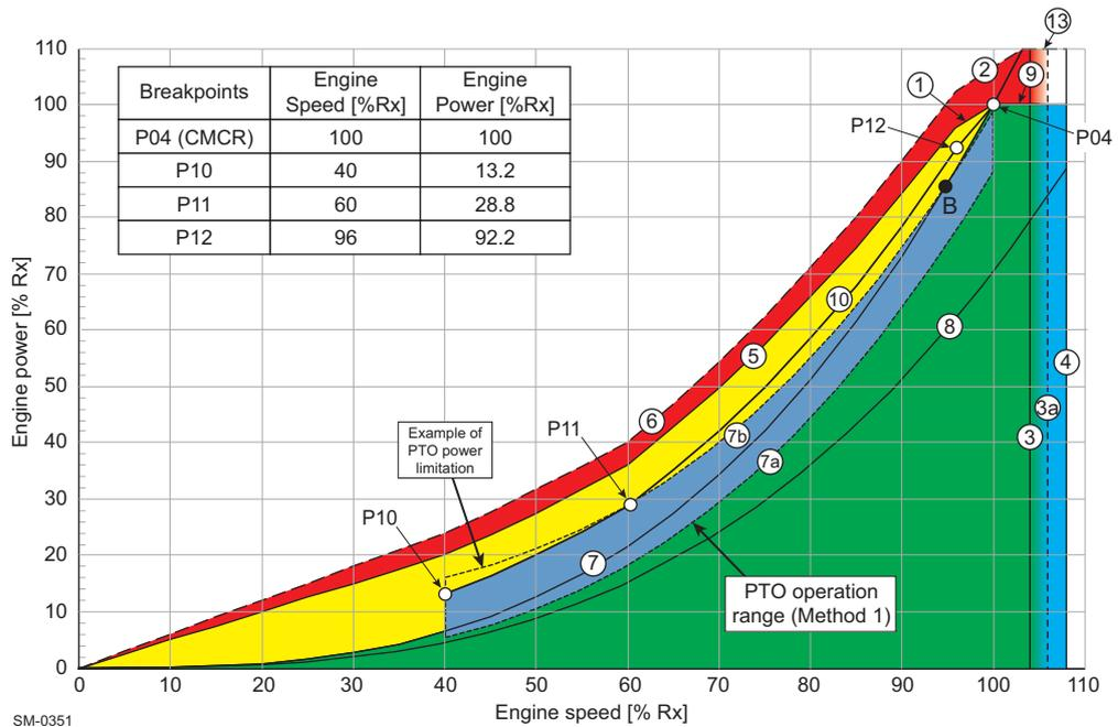
Figure 2-5 Power range limits for PTO operation — Method 1
