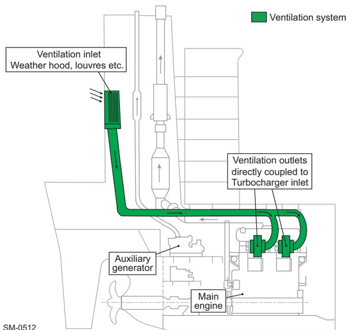
**Figure 4-74 Ventilation system arrangement 2 — Direct engine ventilation system**
