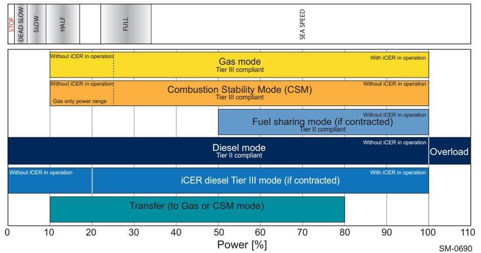
Figure 1-2 Operating modes of the X-DF2.0 engine
