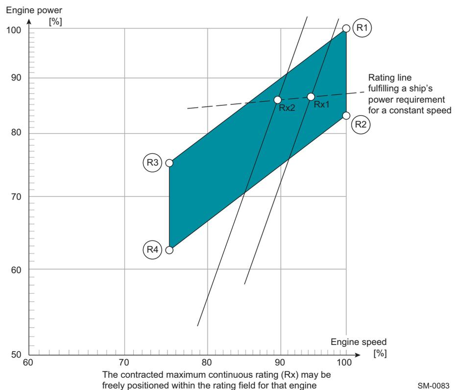
Figure 2-1 Rating field for the X52DF-2.1
