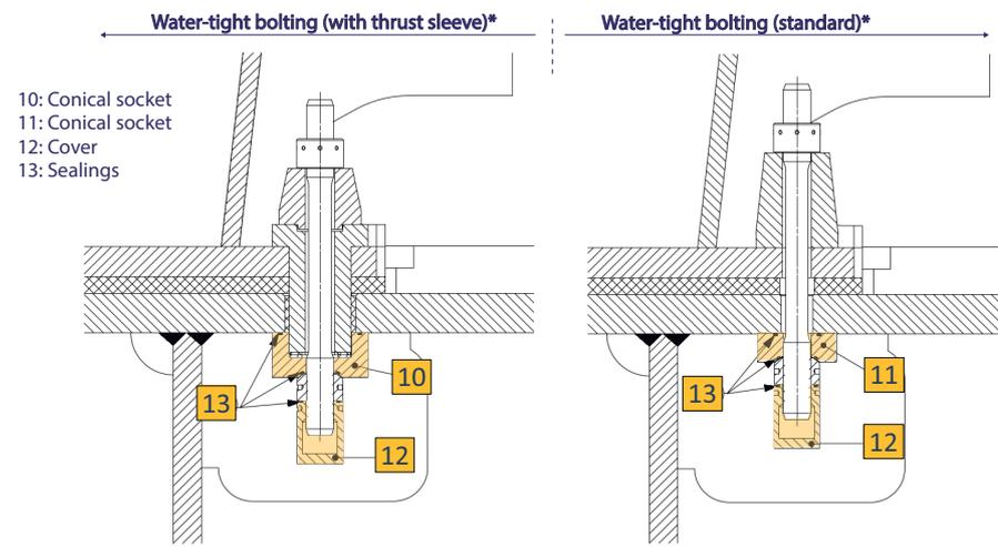
(\*Assembly parts for water-tight bolts)
