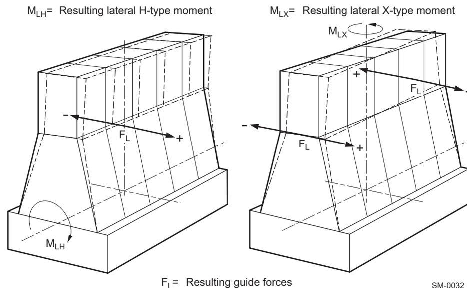
**Figure 6-5 Lateral vibration — X-type and H-type**
