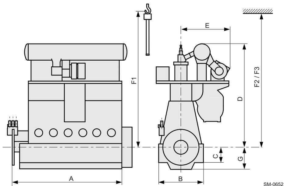
Figure 3-1 Engine dimensions
