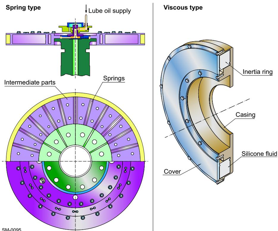
Figure 6-15 Vibration dampers (spring type and viscous type)
