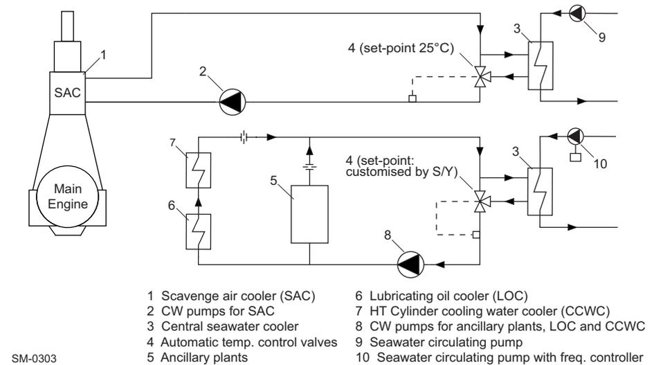
**Figure 4-27 Separate SAC and LT cooling circuits**
