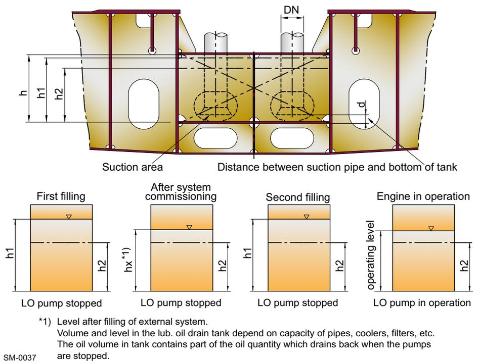
**Figure 4-34 Dimensioning and filling process of lubricating oil drain tank**
