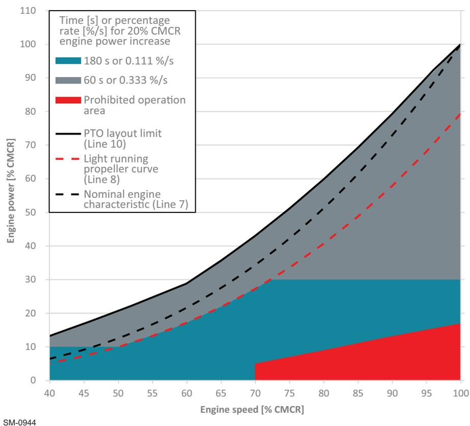
Figure 4-81 Maximum power increase rate for PTO application in gas mode
