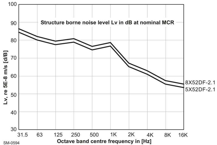
Figure 7-7 Structure-borne noise level at engine feet vertical
