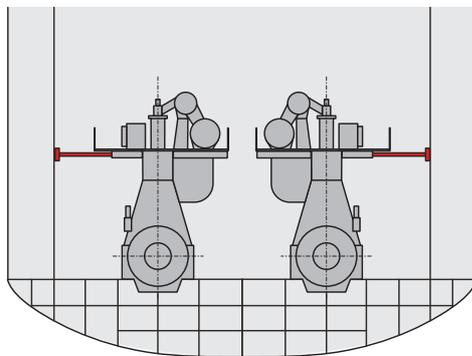
Installation of lateral stays on the fuel side with:
