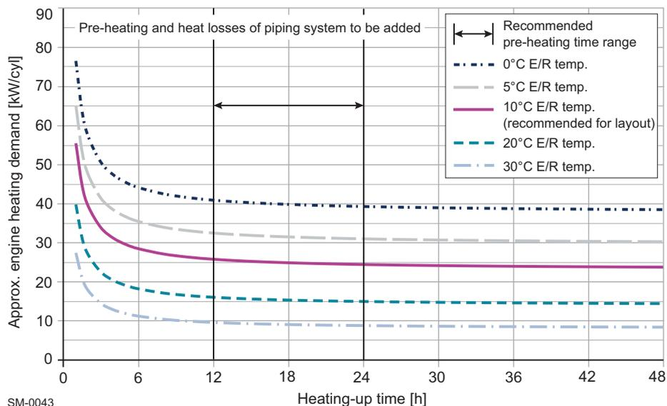
**Figure 4-29** Pre-heating power requirement per cylinder
