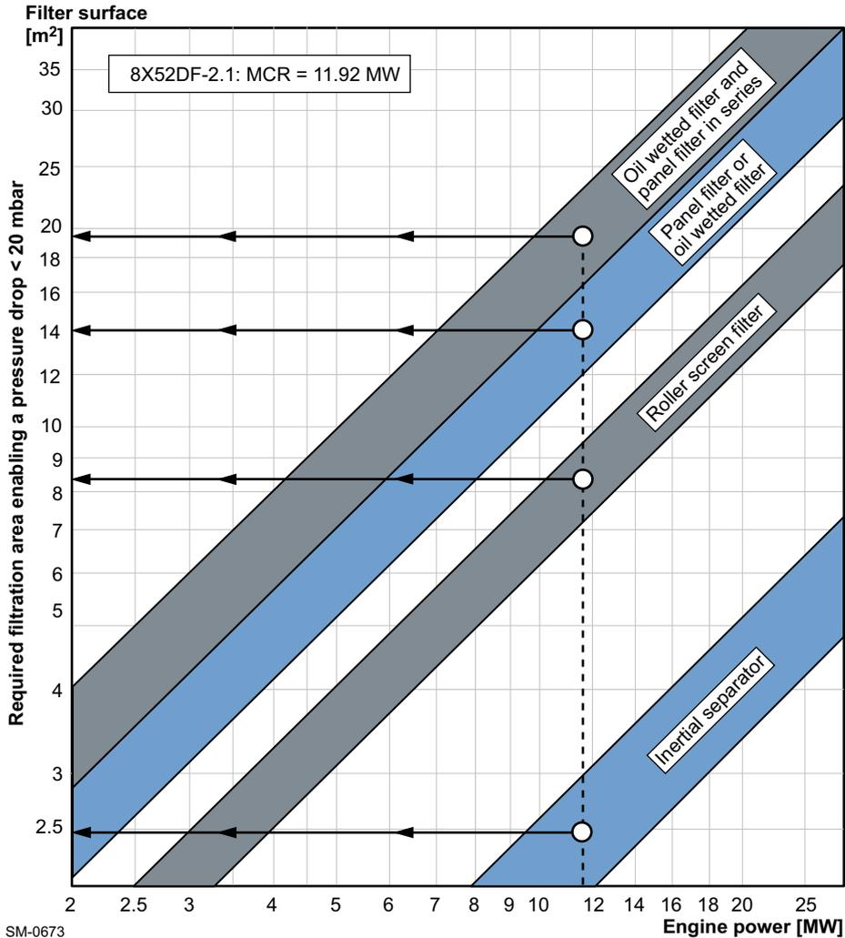
Figure 4-75 Air filter size (example for 8-cyl. engine)
