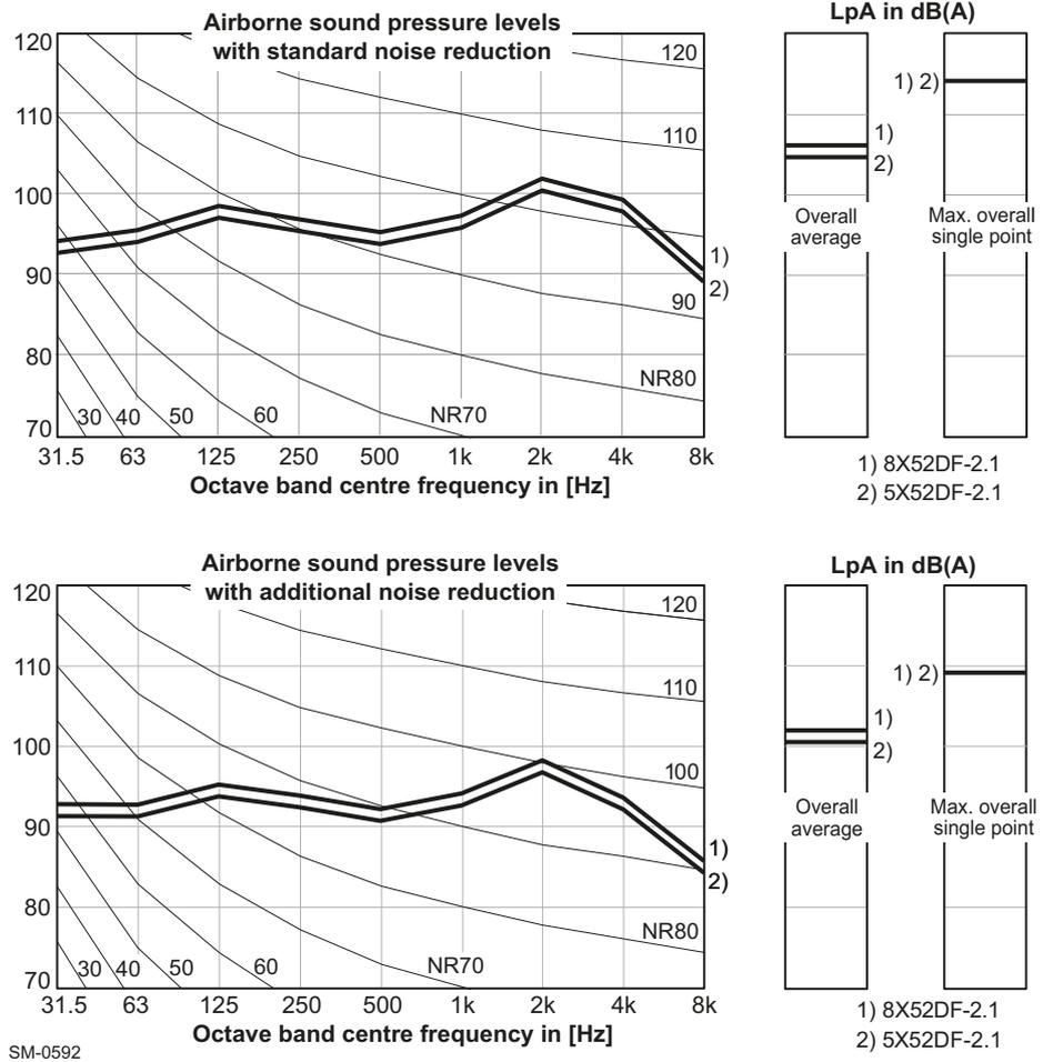
**Figure 7-4 Sound pressure level at 1 m distance from engine**
