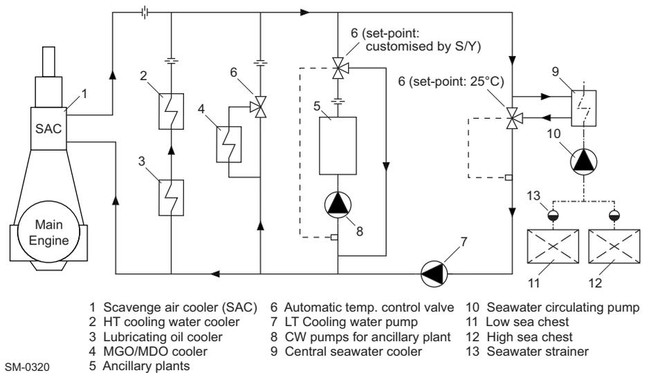
**Figure 4-26** LT cooling water circuit — Dual set-point temperatures
