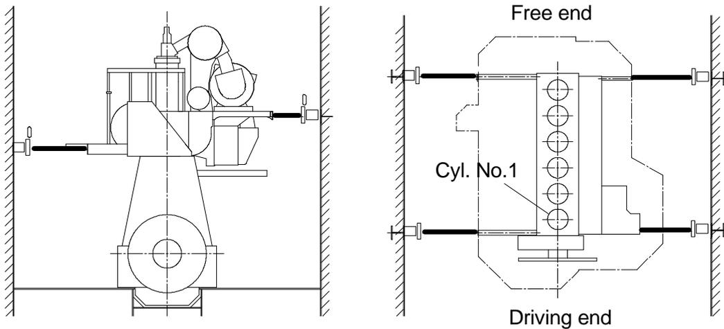
**Figure 3: Principle of lateral stays assembly**
