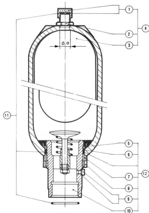
Figure6: Hydropneumatic accumulator parts
