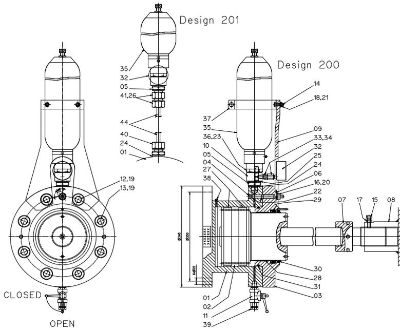
**Figure 8: Hydraulic cylinder assembly parts**
