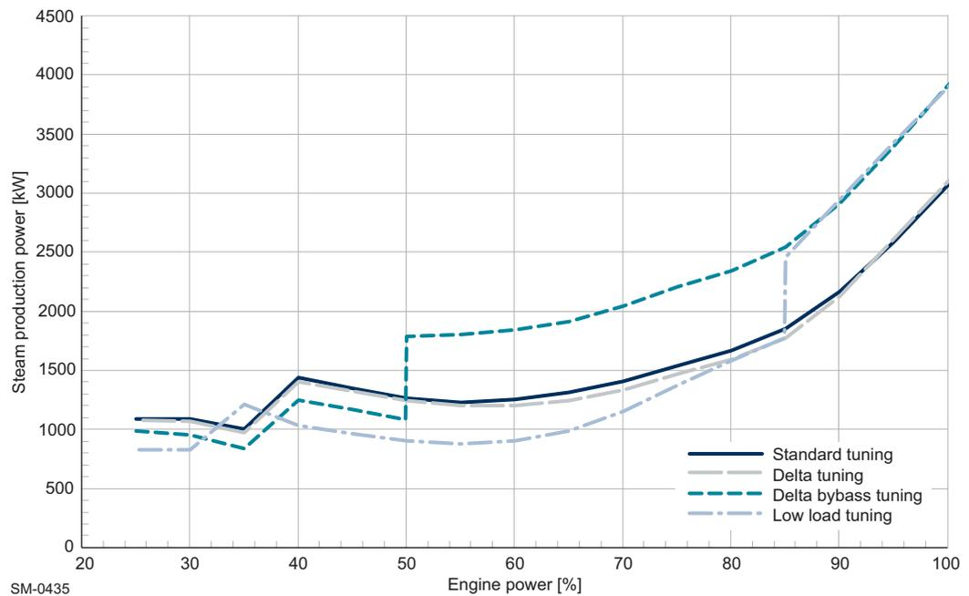
Figure 1-5 Steam production power diagram
