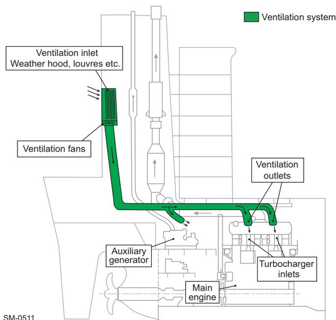
**Figure 4-19 Ventilation system arrangement 1 — Engine room ventilation system**
