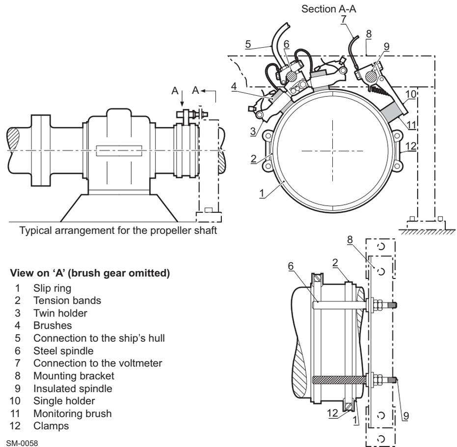
**Figure 3-4 Typical shaft earthing arrangement**
