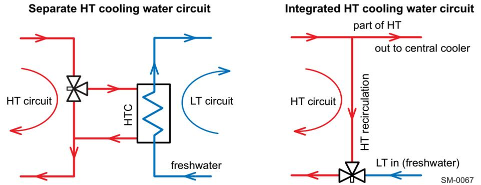
**Figure 4-4** Principal layouts of HT cooling water circuit
