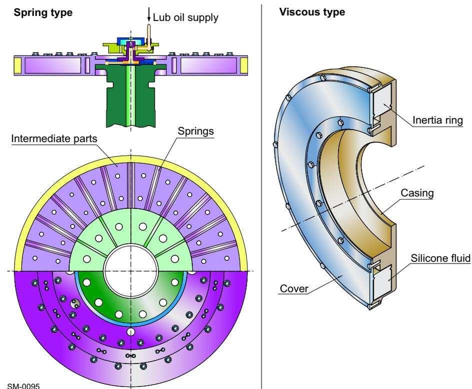
**Figure 6-8** Vibration dampers (spring type and viscous type)
