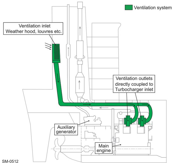
**Figure 4-20 Ventilation system arrangement 2 — Direct engine ventilation system**
