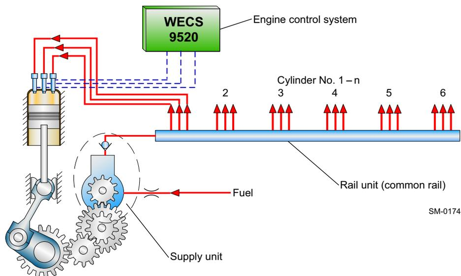
Figure 1-11 Flex system parts
