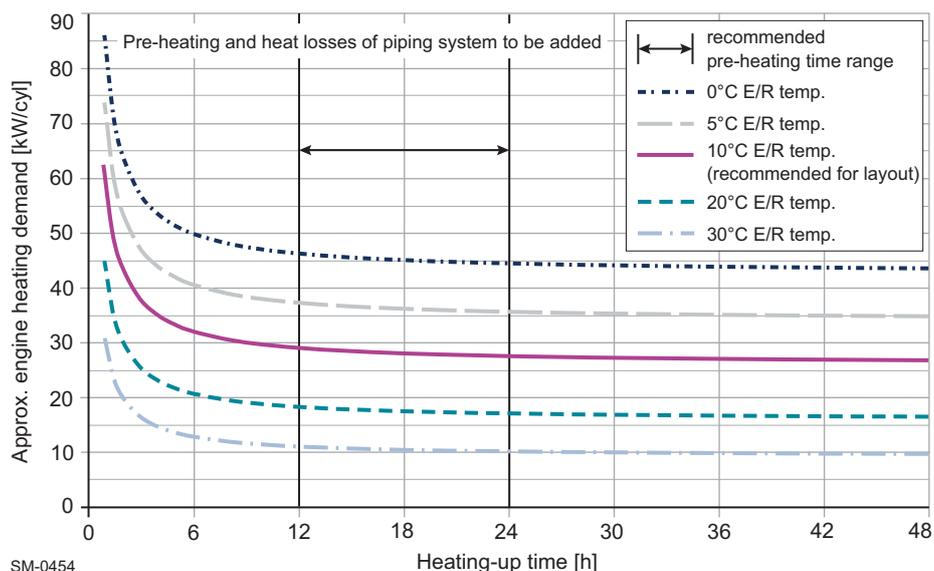
**Figure 4-5 Pre-heating power requirement per cylinder**
