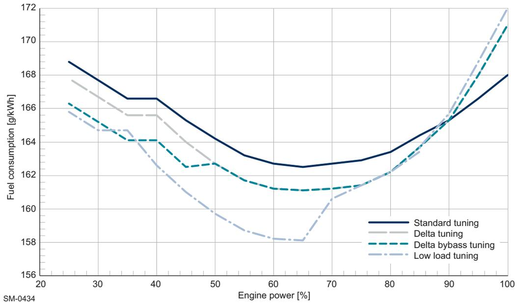
Figure 1-4 Typical BSFC curves in relation to engine power
