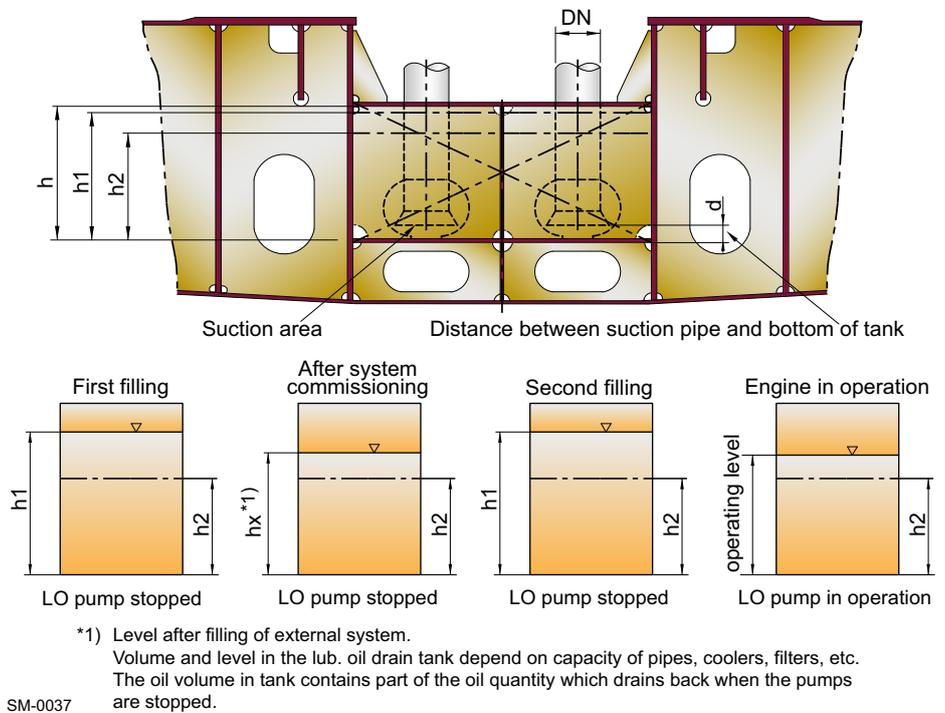
Figure 4-7 Dimensioning and filling process of lubricating oil drain tank
