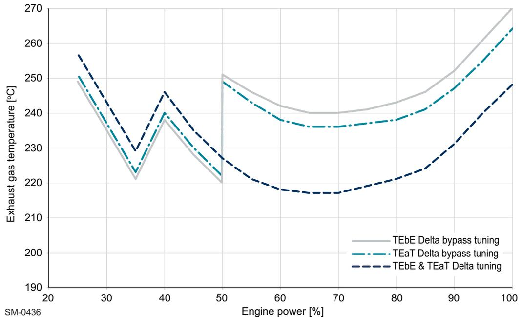
Figure 1-7 Exhaust gas temperature increase with DBT
