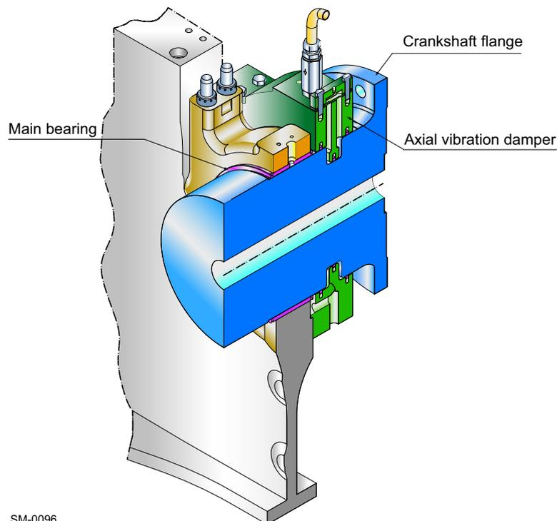
**Figure 6-9** Example of axial vibration damper
