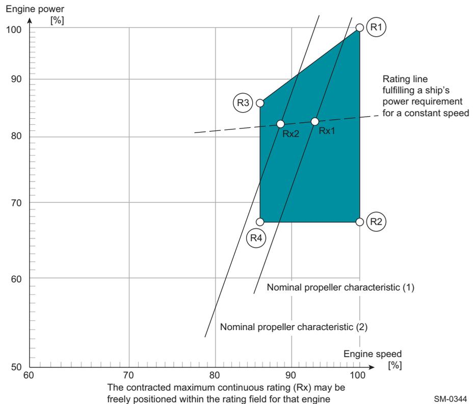
Figure 2-1 Rating field for RT-flex58T-E
