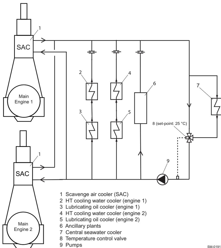
Figure 4-1 LT cooling water system for twin-engine installation
