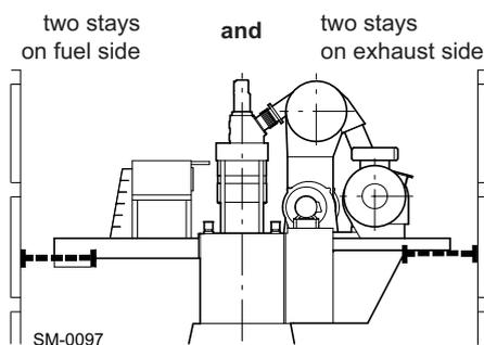
**Figure 6-6** General arrangement of hydraulic stays for both-side installation
