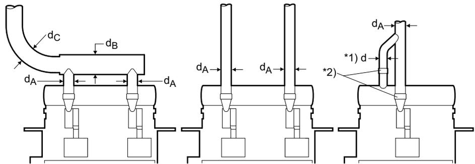
\*1) The purpose for this by-pass is to allow engine operation after a turbocharger failure. During normal operation it is blinded off. The by-pass can be omitted if agreed with the classification society and the owner.
