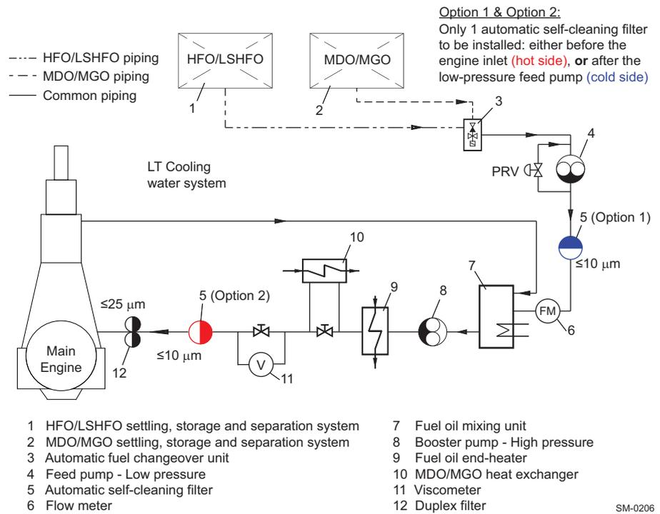
**Figure 4-12 Fuel oil filter arrangement 'A'**
