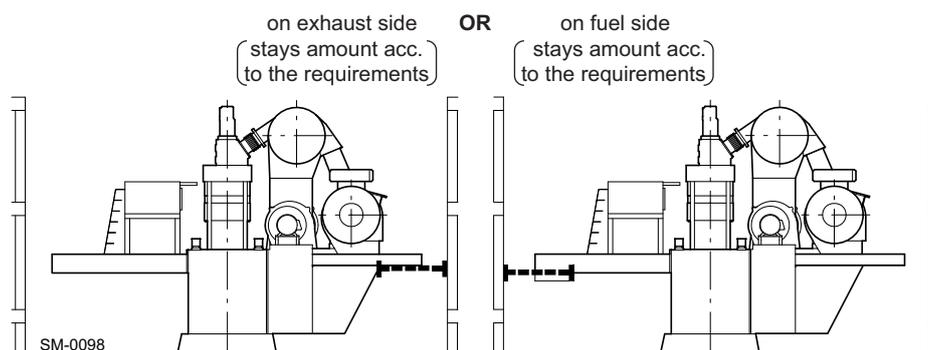
**Figure 6-5** General arrangement of hydraulic stays for one-side installation
