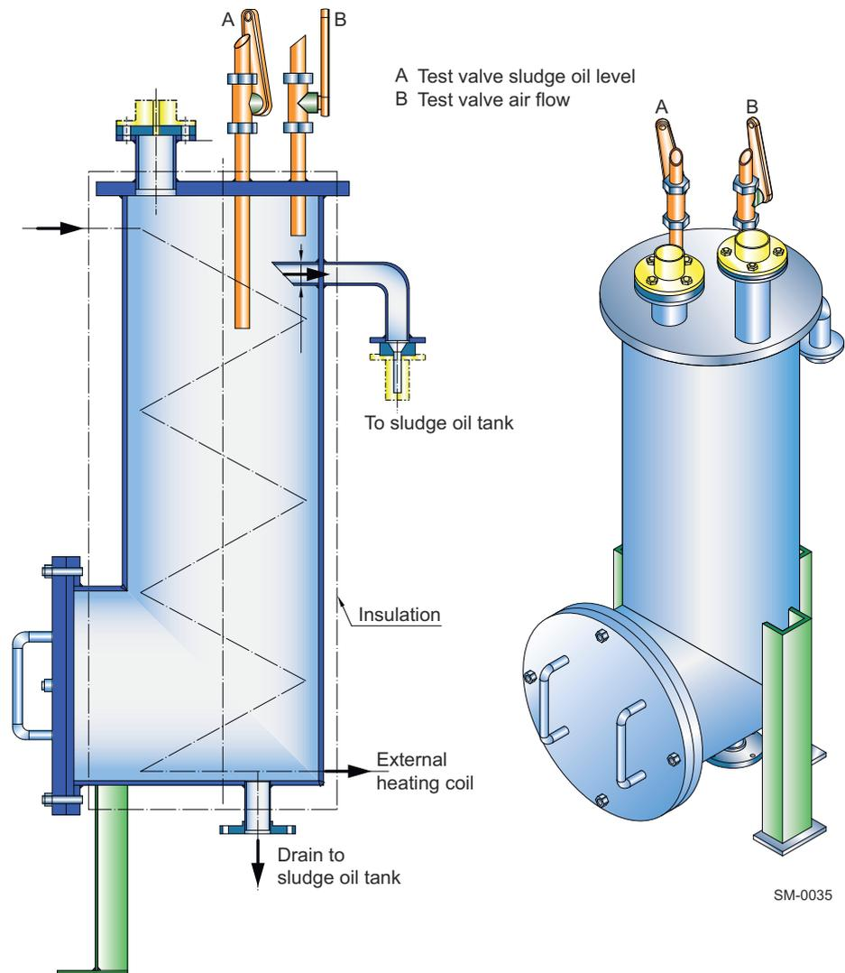
Figure 4-16 Sludge oil trap
