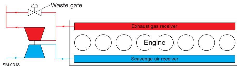
**Figure 1-6** Functional principle of an exhaust gas waste gate
