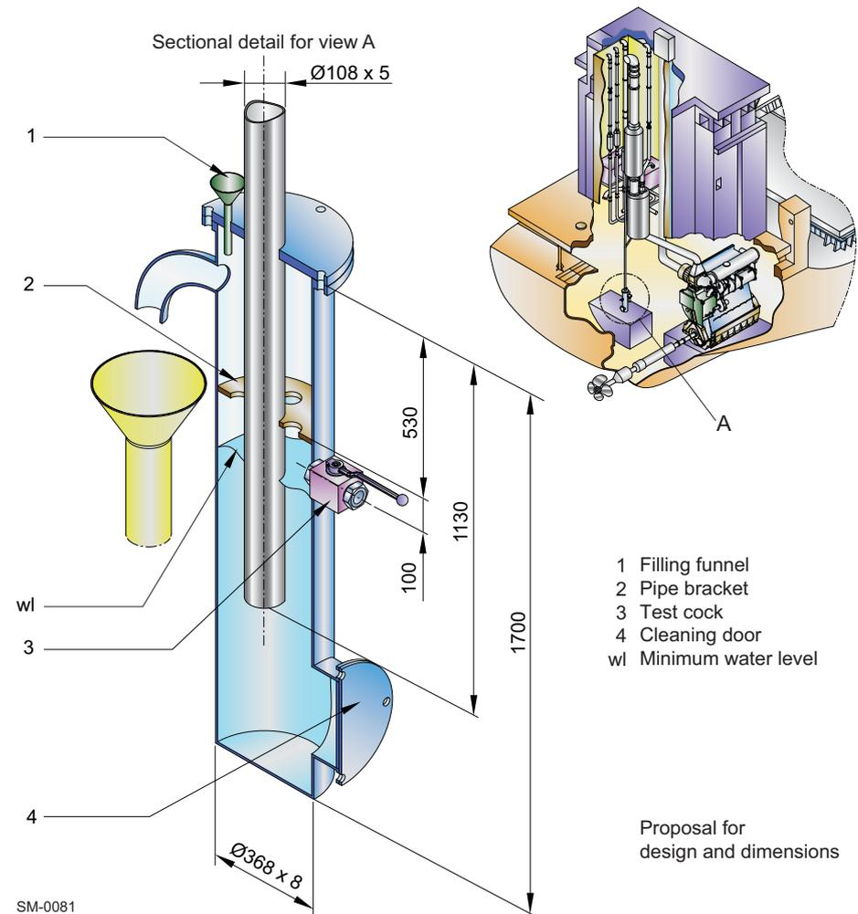
Figure 4-17 Arrangement of automatic water drain
