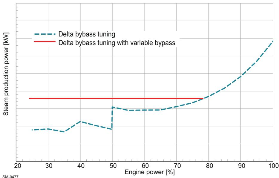
**Figure 1-8 Steam production of Delta bypass tuning with variable bypass**
