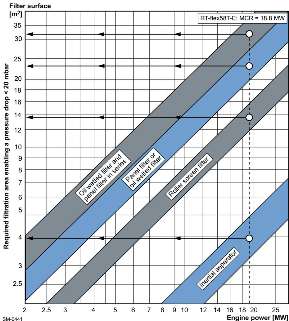
Figure 4-21 Air filter size (example for 8-cyl. engine)
