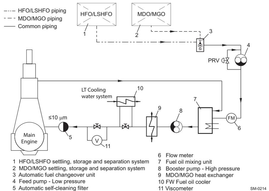
**Figure 4-13 Fuel oil filter arrangement 'B'**
