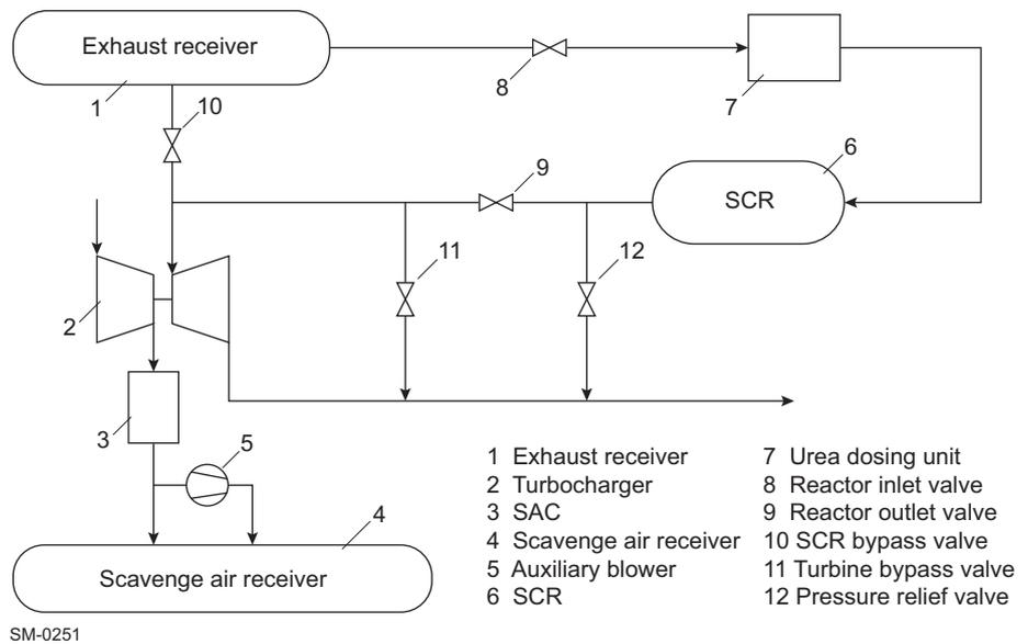
Figure 7-3 High-pressure SCR — Arrangement
