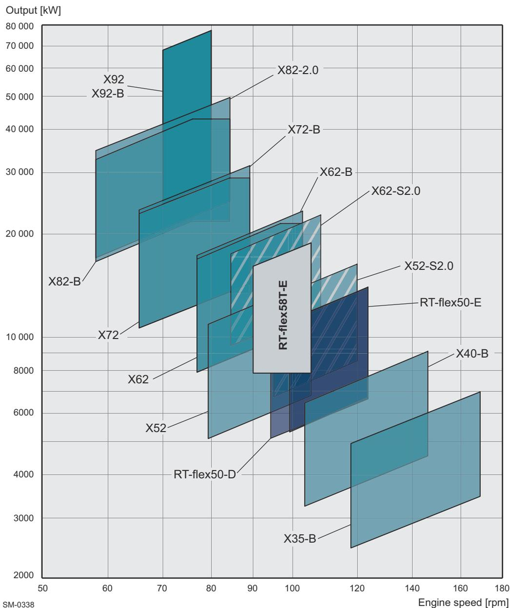
Figure 1-2 Power/speed range of WinGD diesel engines
