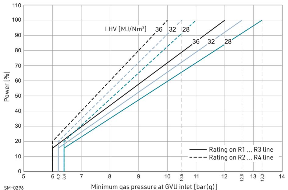
**Figure 4-26 Design gas feed pressure requirements (engines with GVU)**
