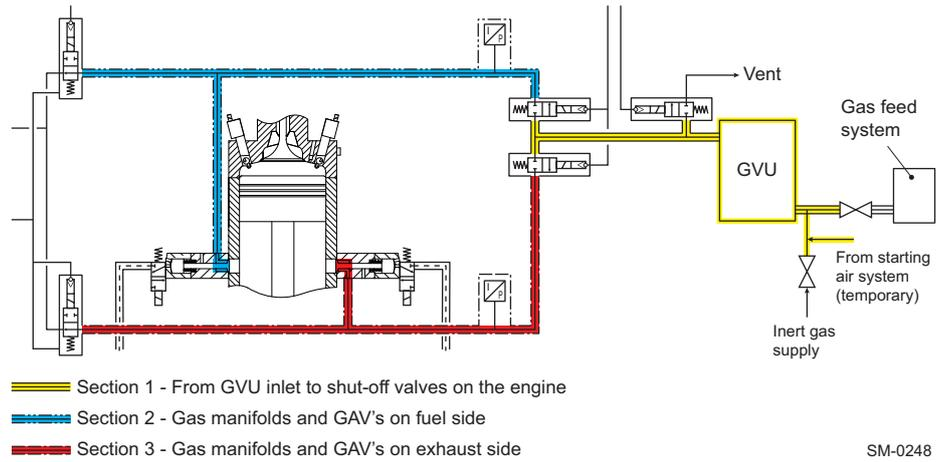
Figure 4-30 Gas leak test sequence (engines with GVU)
