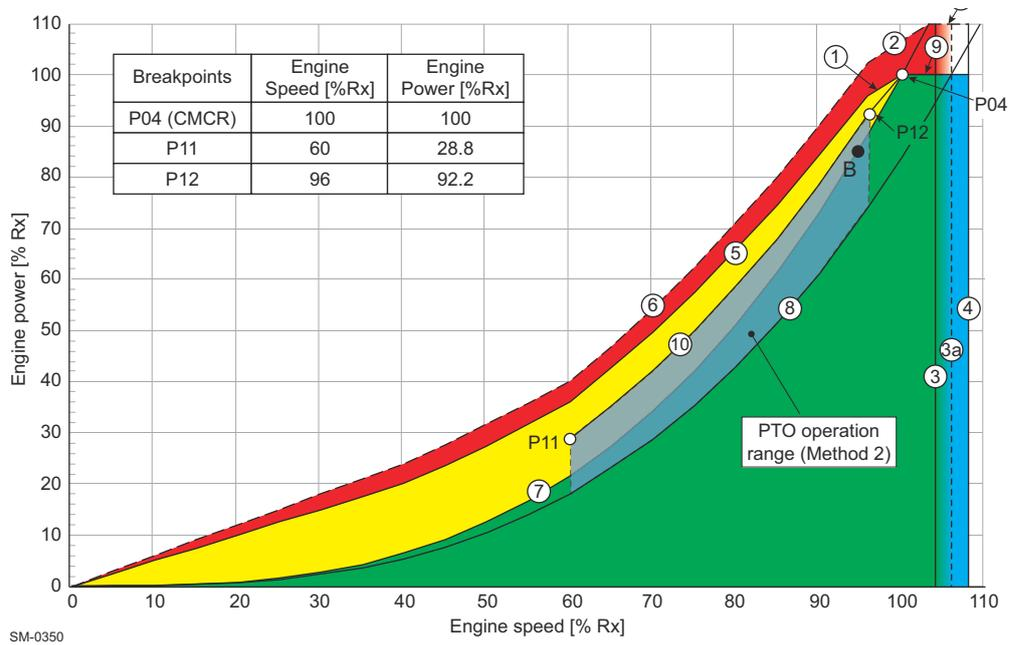
**Figure 2-6 Power range limits for PTO operation — Method 2**
