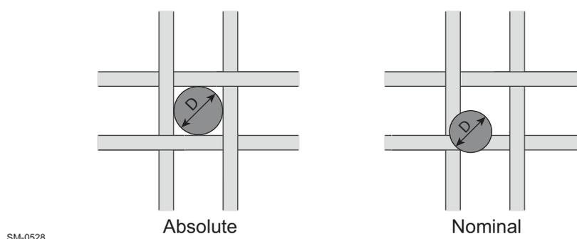
**Figure 4-17** Mesh size difference between absolute and nominal
