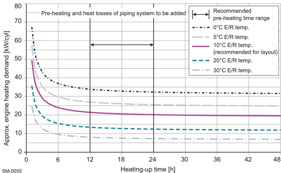
**Figure 4-9 Pre-heating power requirement per cylinder**
