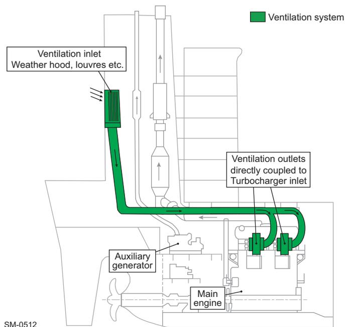
**Figure 4-42 Ventilation system arrangement 2 — Direct engine ventilation system**
