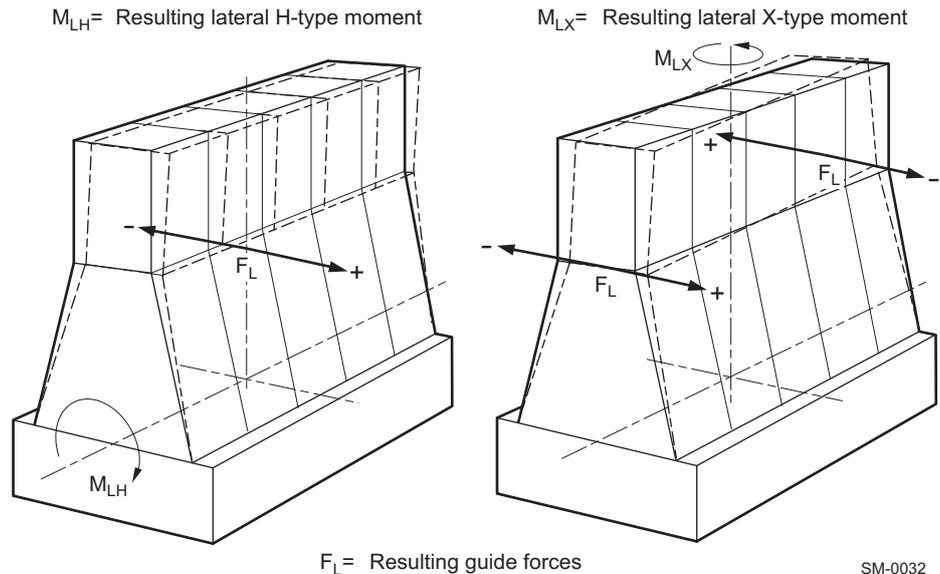
**Figure 6-4 Lateral vibration — X-type and H-type**
