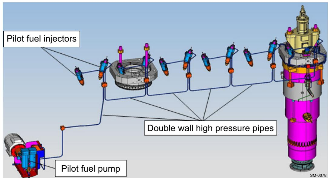
Figure 4-23 Pilot fuel high-pressure system
