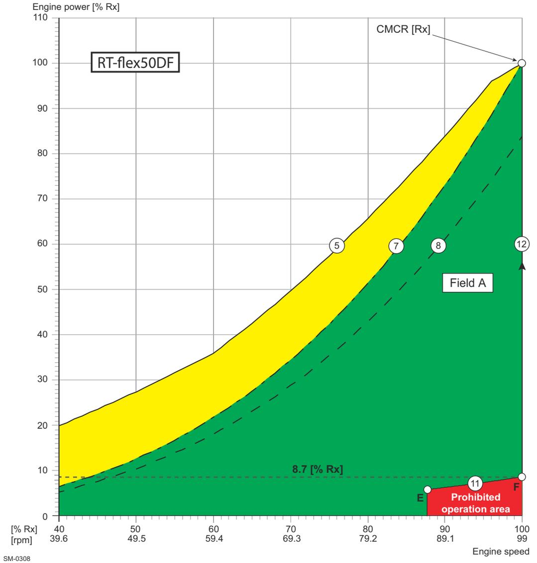
Figure 2-10 Prohibited engine operation area (CMCR speed = R3—R4)
