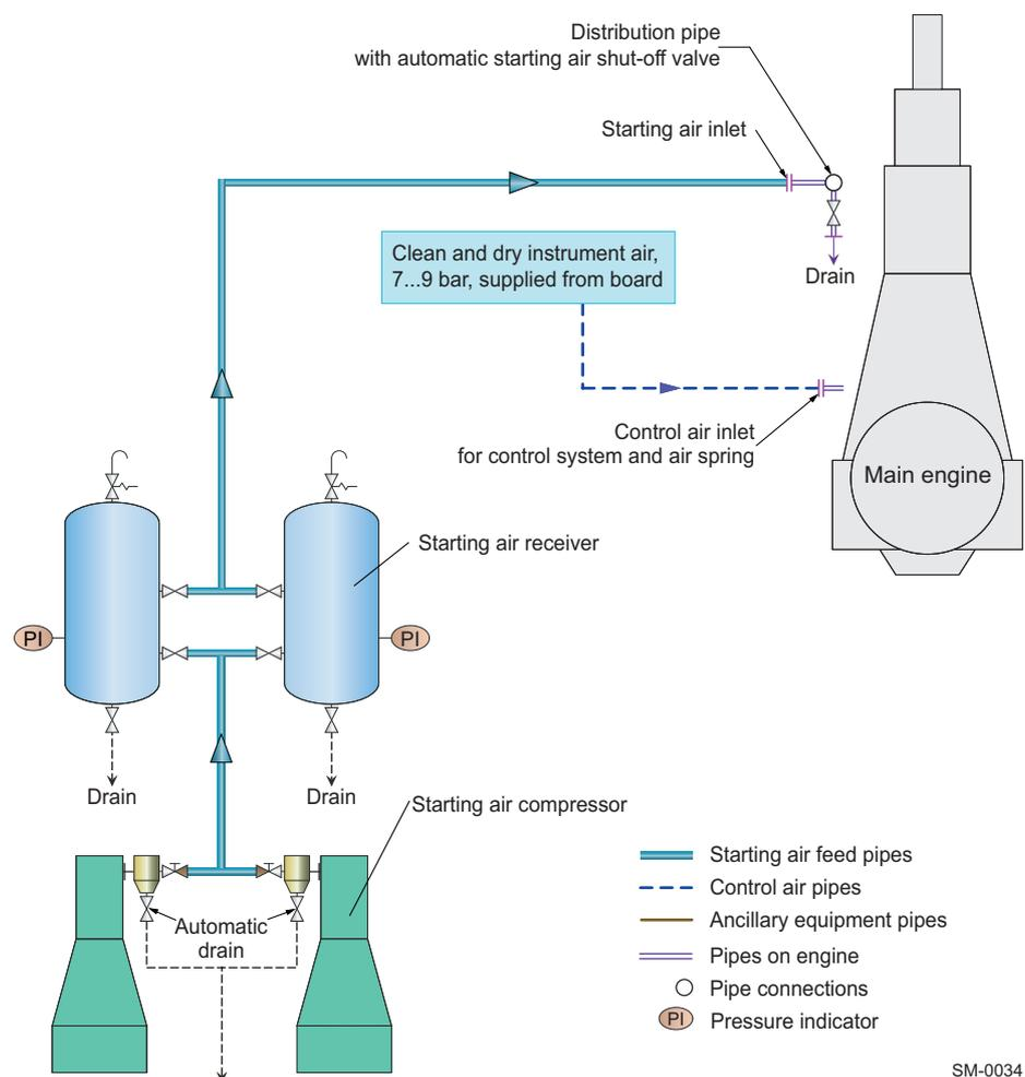
**Figure 4-37 Starting and control air system**
