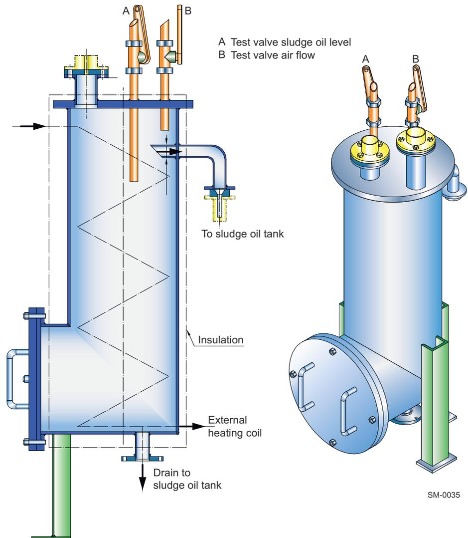
Figure 4-38 Sludge oil trap
