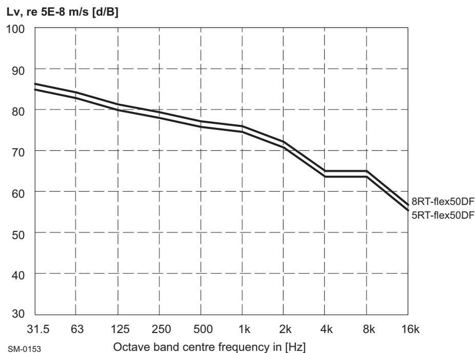
Figure 7-6 Structure-borne noise level at engine feet vertical
