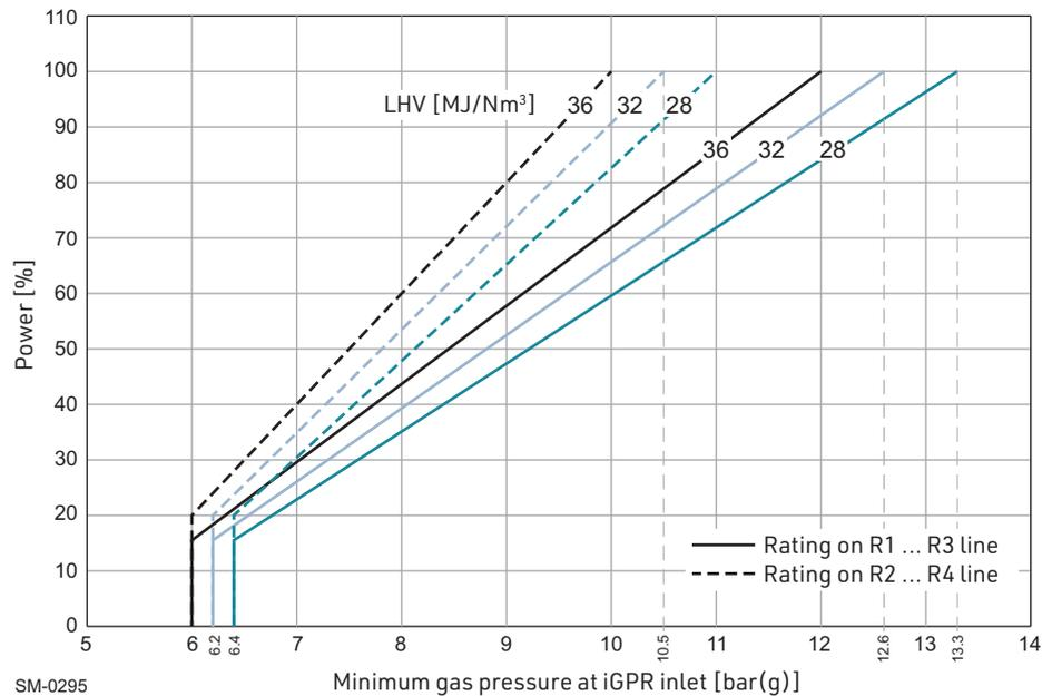
**Figure 4-33 Design gas feed pressure requirements (engines with iGPR)**
