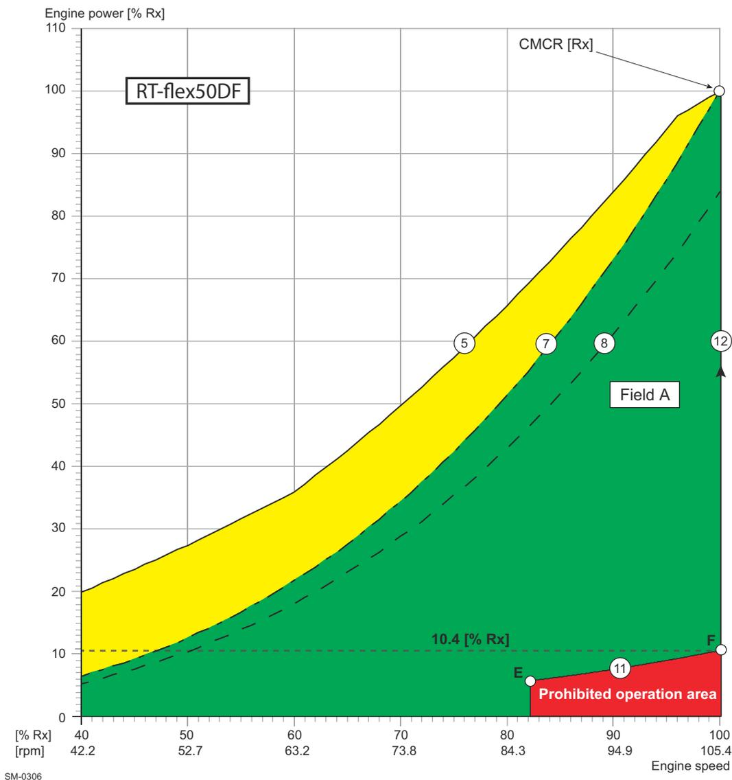
Figure 2-9 Prohibited engine operation area (CMCR speed = 85% of R1—R2)
