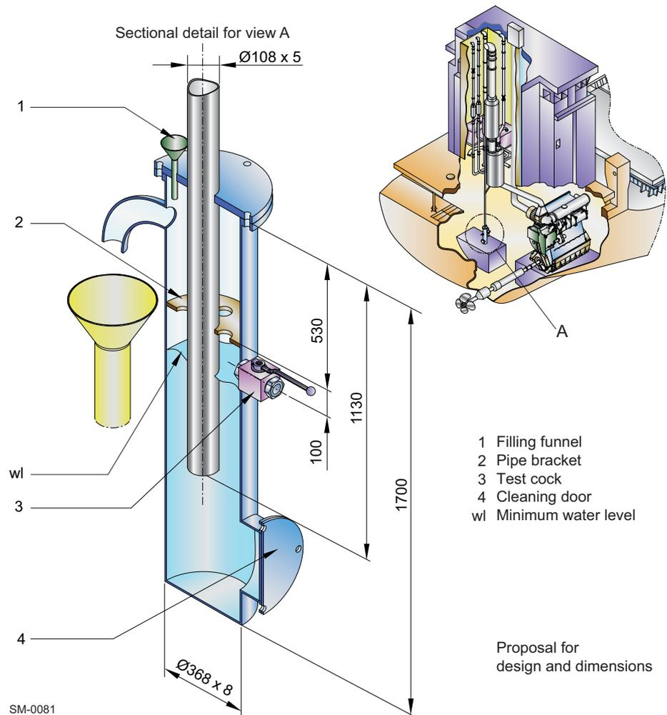
Figure 4-39 Arrangement of automatic water drain
