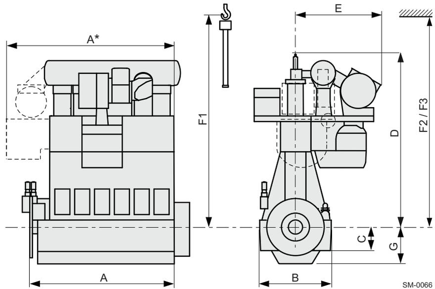
Figure 3-1 Engine dimensions
