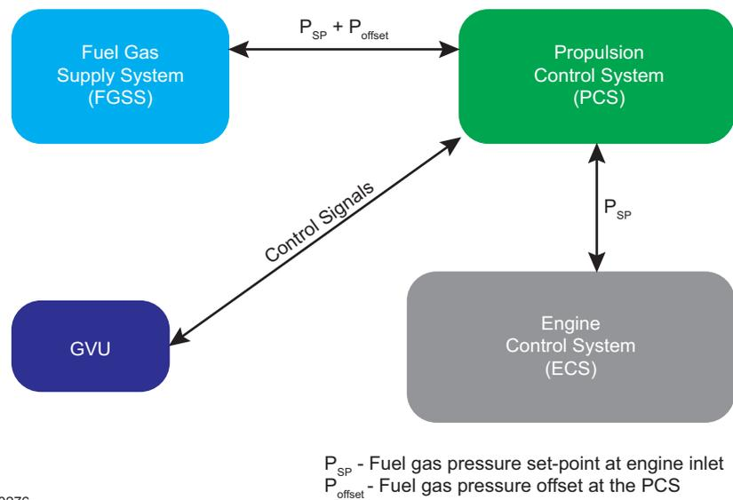
Figure 4-27 Fuel gas pressure control at engine inlet (engines with GVU)
