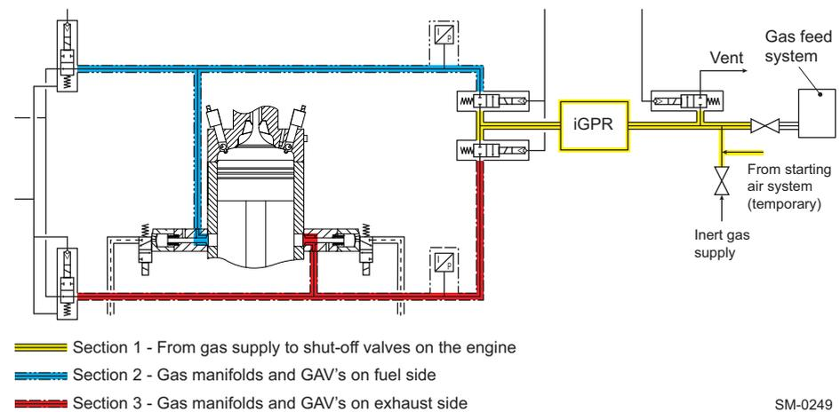
Figure 4-36 Gas leak test sequence (engines with iGPR)
