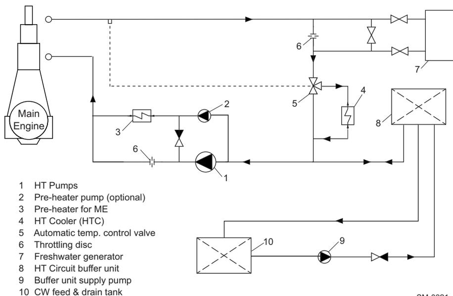
Figure 4-8 HT cooling water circuit
