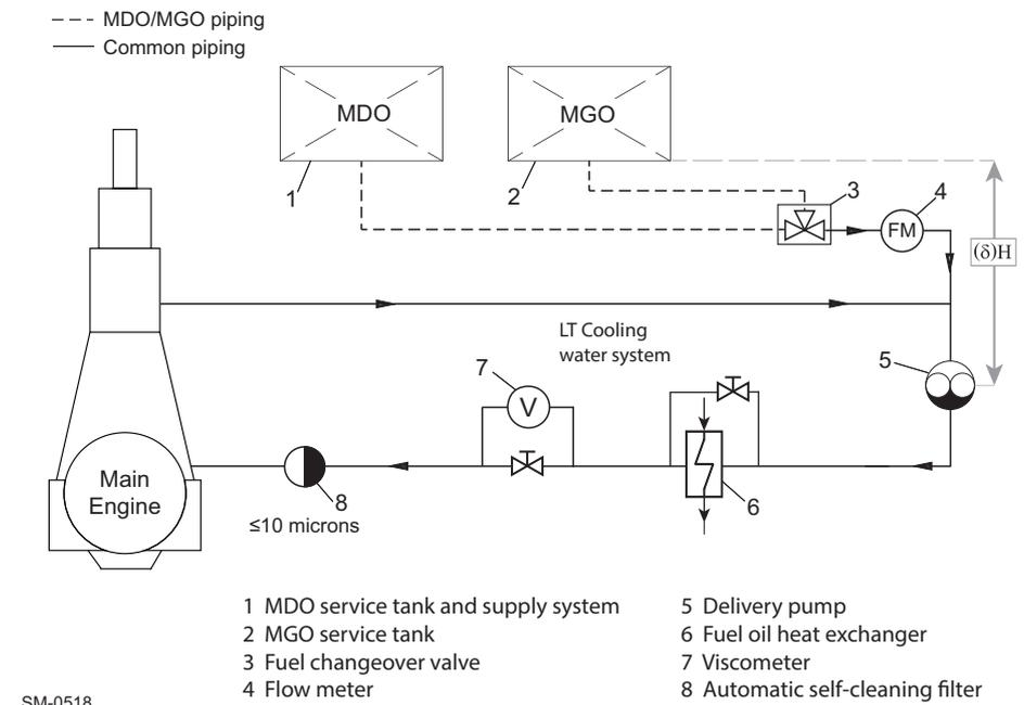
**Figure 4-20 Fuel oil system — Arrangement with only MDO/MGO or MGO**
