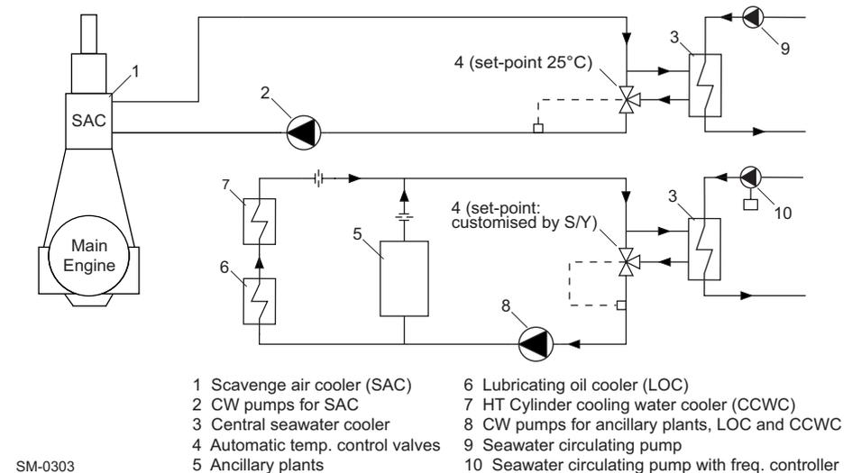
**Figure 4-7 Separate SAC and LT cooling circuits**
