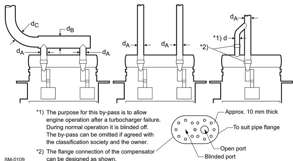
**Figure 4-40 Determination of exhaust pipe diameter**
