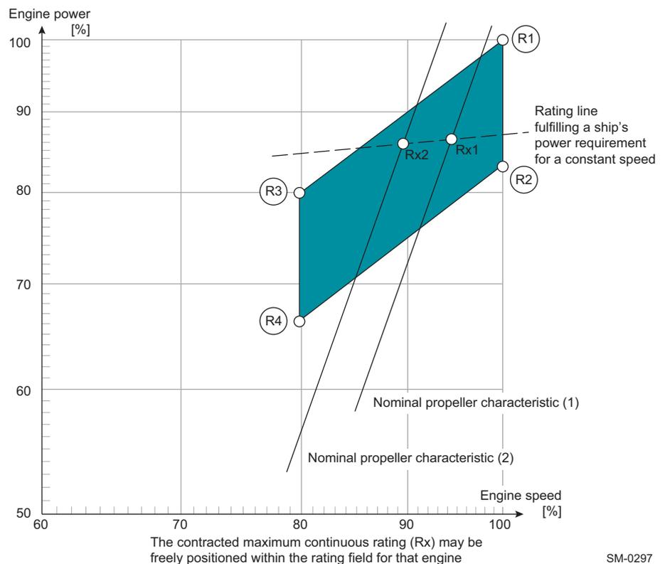
**Figure 2-1 Rating field for RT-flex50DF**
