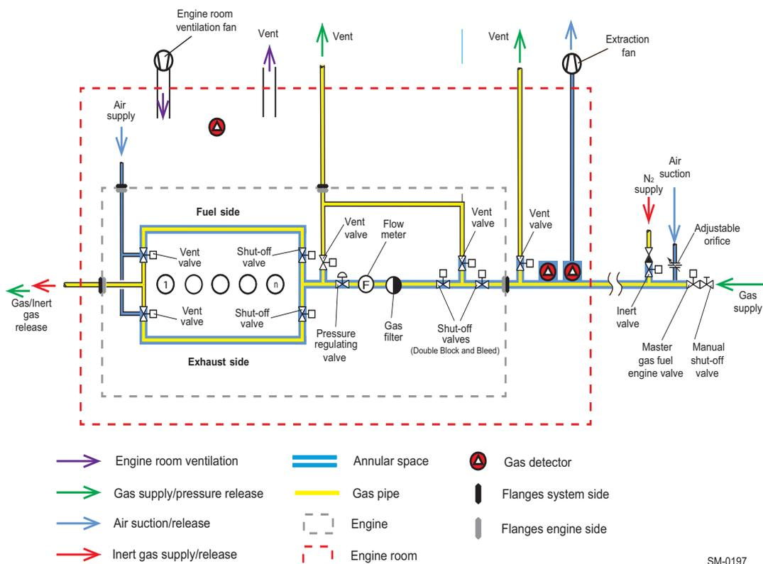
**Figure 4-35 Gas system with iGPR**
