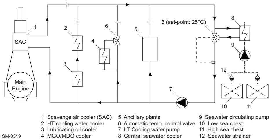
**Figure 4-5** LT cooling water circuit — single set-point temperature
