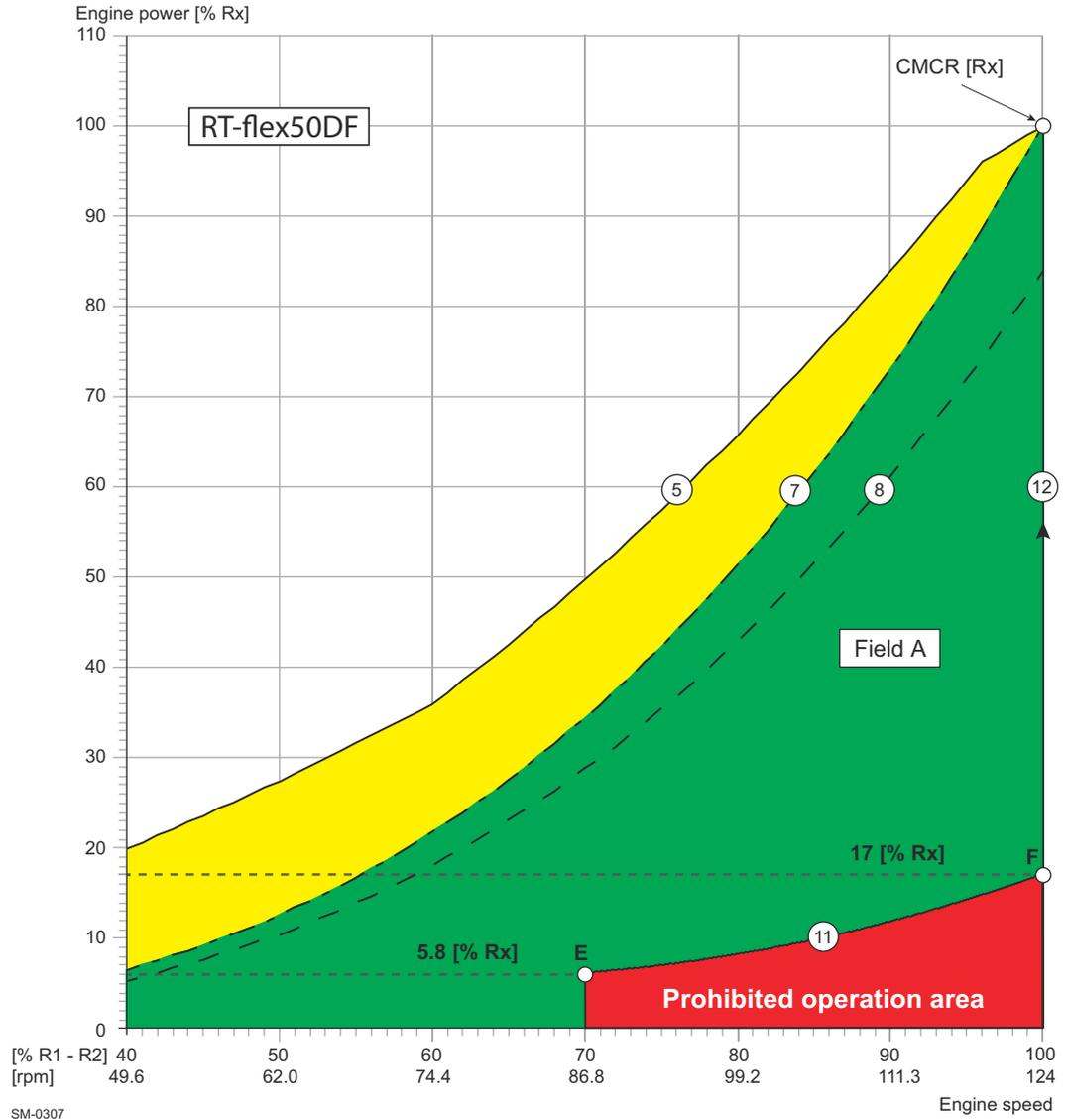
Figure 2-7 Prohibited engine operation area (CMCR speed = R1—R2)
