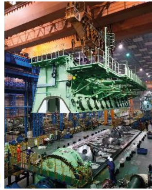
12X92DF: the largest Otto-cycle engine ever built.
