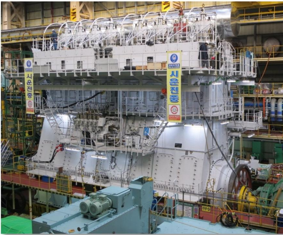
Figure 13: First 8X92 engine during shop-test at Hyundai Heavy Industries (HHI)
