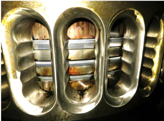
Figure 11: Good piston running behaviour W6X72
