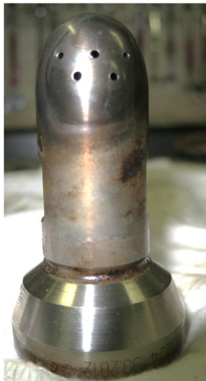
Figure 10: FAST nozzle tip of RT-flex82T after 12,600 running hours
