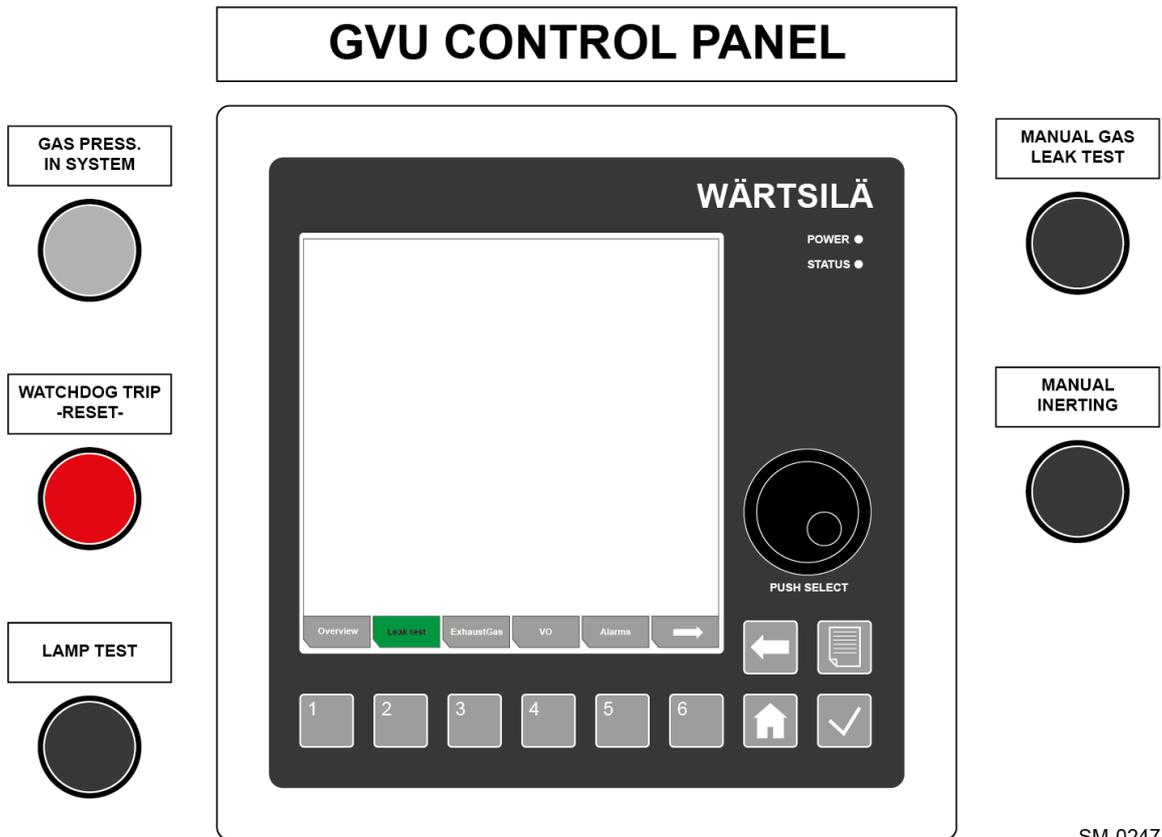
Figure 2-9: The GUV Human Machine Interface (HMI)
