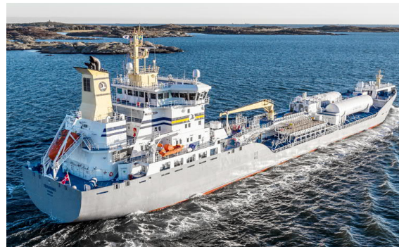
Picture: 5RT-flex50DF powered chemical tanker
