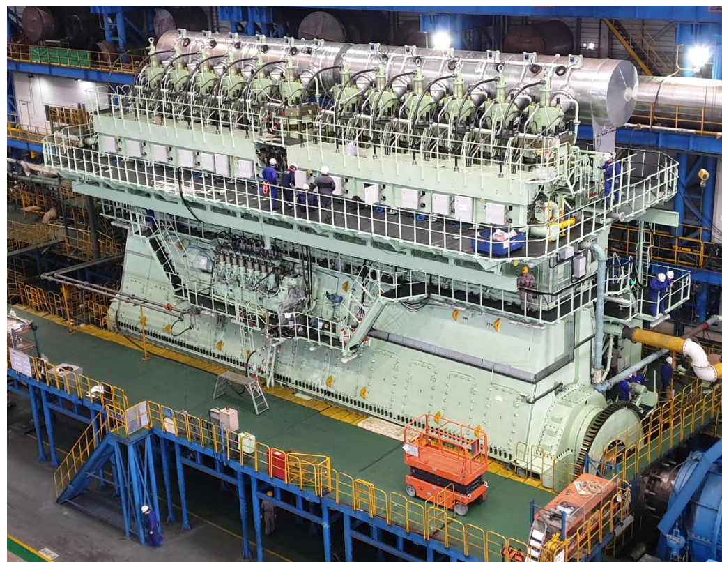
The 12X92DF on testbed
