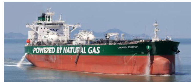
Picture: 7X62DF powered Aframax (Ice class) tanker
