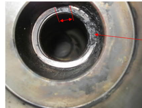
Conical sealing ring as found in pre-chamber – visible crack of conical sealing ring and damage caused by exhaust gas blow-by.
