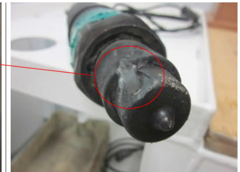
Pilot fuel injector valve with heavy damage due to long term exhaust gas blow-by.
