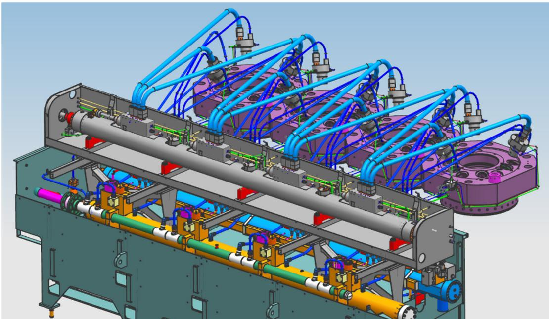
CAD design of fuel flexible injector on RTX-6
