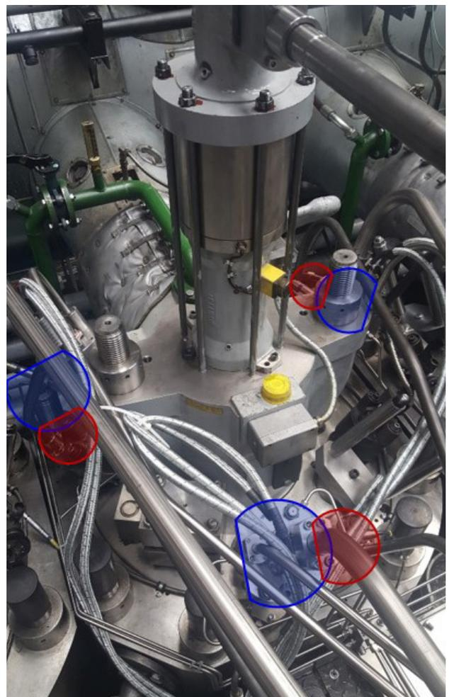
Engine cover: blue areas indicate the position of the fuel flexible injectors, red incates the classic injectors
